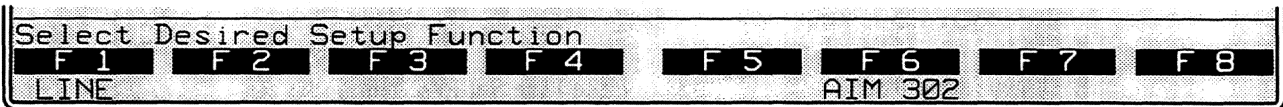
Figure 2-5 Softkey rack on Setup Menu screen for INTERVIEW 8800 PLUS ATM units after disabling WAN testing on the Line Setup screen; compare with softkey rack in Figure 2-3.
