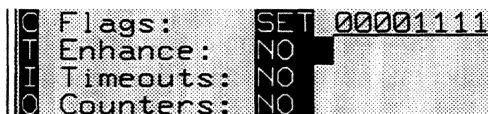
Figure 26-5 A set of eight flag bits may be set on any of the trigger menus.
