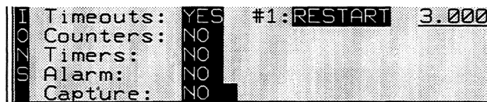
Figure 26-7 Timeout #1 activated to expire in three seconds.
