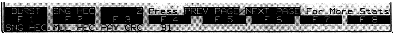
Figure 11-3 Coaxial DS-3 PLCP framing mode EVENT softkeys; B1 is not applicable to DS-3 direct framing mode.
