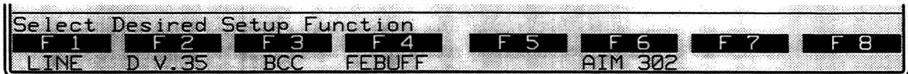
Figure 2-3 Sample softkey rack on Setup Menu screen for INTERVIEW 8800 PLUS ATM units: installed Test Interface Module is Dual-Port V.35 and installed ATM Interface Module is AIM 302.
