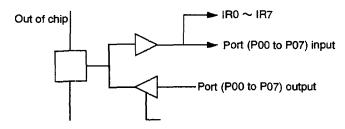
Figure 6-7. Structure of Pins 80 to 83 and 85 to 88
