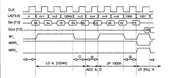
Figure 5-15. Prefetch cycle ( <------> denotes the prefetch cycle. Assumes memory location 1000h has 77h, memory location 1234h has 5Ah, and D register has 81H.)
