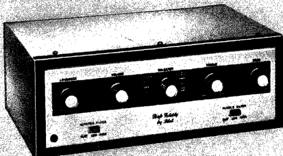
Pilot AA-903B 14-Watt Amplifier
