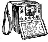
Frequency range: Continuously tuneable, 54 to 220 mc. Sensitivity: from 5 microvolts to 3 volts. Accuracy:  $\pm 2$  db over entire range. Ranges: 0-100-300-1000-10,000-30,000 microvolts RF; with use of built-in precision attenuator, measures 0-0.1-0.3-1-3 volts RF. Selectivity: 0.6 mc bandwidth at 3 db down. Image rejection: 9 db below signal level.
