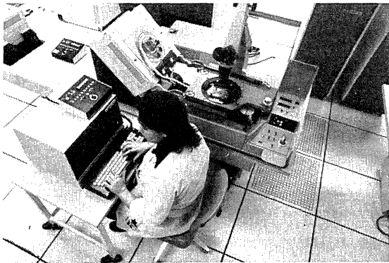
Automated mask inspection machine assures high quality photolithography.
