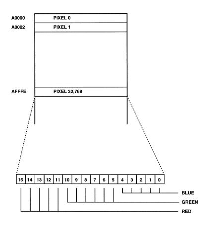
Figure D1-4. 65,536 Color (16-Bit) Packed-Pixel Mode
