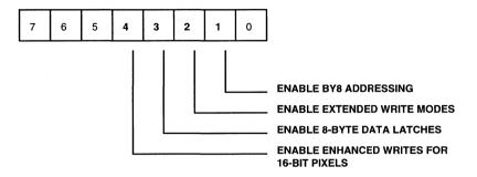
Figure D6–1. Color Expansion Controls
