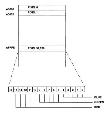
Figure D1-3. 32,768 Color (15-Bit) Packed-Pixel Mode
