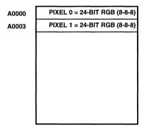
Figure D1–6. 24-bit True Color Packed-Pixel Mode
