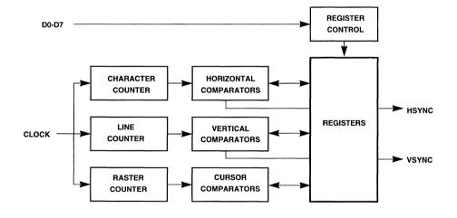
Figure 2–1. CRT Controller Functional Block Diagram
