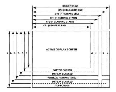
A - CR6 (V TOTAL) B - CR16 (V BLANKING END) C - CR11 (V RETRACE END) D - CR10 (V RETRACE START) E - CR15 (V BLANKING START) F - CR12 (V DISPLAY END) G - RIGHT BORDER H - DISPLAY BLANKED I - HORIZONTAL RETRACE (SYNC) J - DISPLAY BLANKED K - LEFT BORDER
