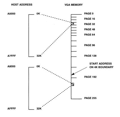
Figure D1–16. Dual-Page (32K Byte) Mapping Scheme
