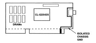
The CL-GD542X family has built-in latch-up protection circuitry, but to add **additional** latchup protection, power to the CL-GD542X should be provided through two 1 $\Omega$  1/4-Watt resistors. These resistors should be placed in parallel to +5V, with the power pins AVDDx and VDDx of CL-GD542X along with the decoupling capacitors shown in the following figure.
