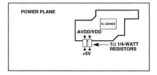
**NOTE:** The solid line cuts the main Power Plane and creates a separate power segment for the CL-GD542X. The main Power Plane can be used to supply the power for the DRAMs, Buffers, and EPROMs (if any).
