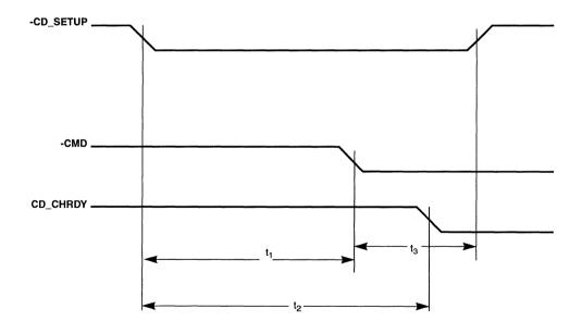
Figure 7–21. -CD\_SETUP Timing (MicroChannel® Bus)
