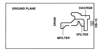
Use the following diagram as a reference for Ground Plane layout.
