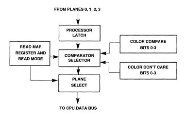
Figure 2–3. Graphics Controller Read Operation
