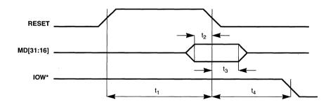
Figure 7–36. Reset Timing
