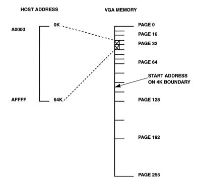
Figure D1–14. Single 64K Byte Page Mapping Scheme
