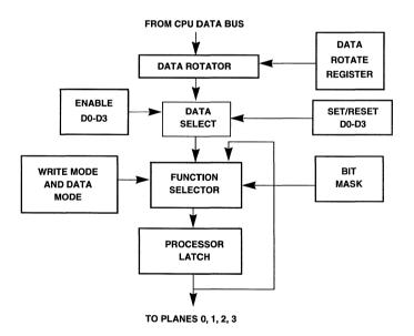
Figure 2–2. Graphics Controller Write Operation
