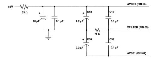
Figure B17–1. VFILTER Design Layout
