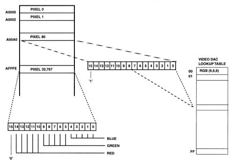
Figure D1–5. Mixed-32,768-Color (15-Bit) Packed-Pixel Data Format
