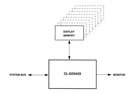
Figure 2–7. Video Subsystem Architecture
