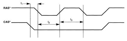
Figure 7–30. CAS\*-before-RAS\* Refresh Timing (Display Memory Bus)
