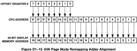
ure D1–15. 64K Page Mode Remapping Adder Alignme For 1-Mbyte Display Memory
