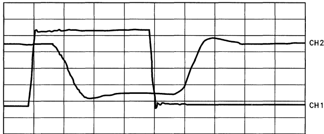
Figure 6. 5 MHz Output into 1000 pF Load
