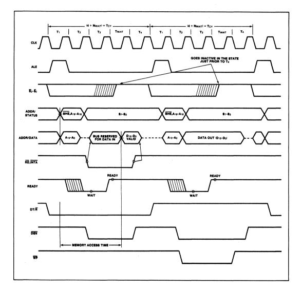
Figure 3. Basic System Timing
