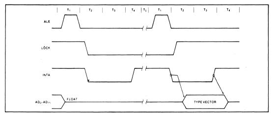
Figure 4. Interrupt Acknowledge Sequence
