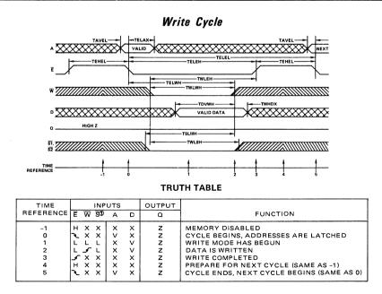
NOTES: 1 Device selected only if both  $\overline{S1}$  and  $\overline{S2}$  are low, and deselected if either  $\overline{S1}$  or  $\overline{S2}$  are high.
