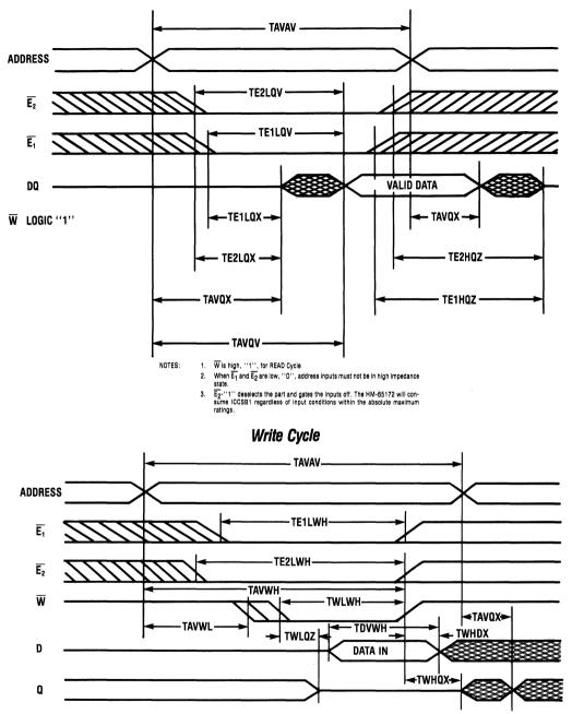
Writing data into the memory requires an overlap of  $\overline{E_1}$ ,  $\overline{E_2}$  and  $\overline{W}$ . When  $\overline{E_1}$  or  $\overline{E_2}$  transition low simultaneously with the  $\overline{W}$  low transition, or after  $\overline{W}$  transitions low, the outputs will remain in a high impedance state. After  $\overline{W}$  transitions high and if  $\overline{E_1}$  and  $\overline{E_2}$  are low, the DQ pins are in the output
