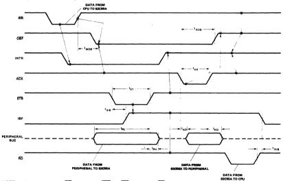
NOTE: Any sequence where WR occurs before ACK and STB occurs before RD is permissible. (INTR = IBF • MASK • STB • RD + OBF • MASK • ACK • WR )
