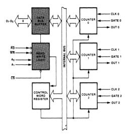
Figure 1. Data Bus Buffer and Read/Write Logic Function
