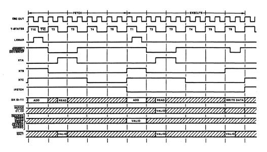
The dynamic or high frequency timing illustrates the propagation delays at specified operating frequencies. (Refer to specifications) It defines the interface requirements for memory and I/O devices on the bus.
