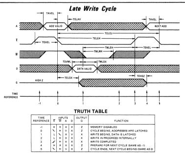
The late write cycle is a cross between the early write cycle and the read-modify-write cycle.
