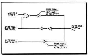
Both the 80C86 and the 82C55A use this on-chip "bus-hold" circuitry to provide valid input voltages to specific inputs without using external resistors.
