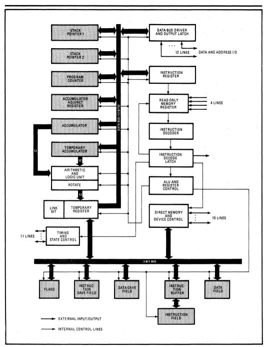
1. Chip off the old block. The 6120 C-MOS processor chip implements the much-used PDP-8 architecture, executing an extended PDP-8/A instructions set. The design uses two system buses — the data and address I/O bus and the C-bus — and 12 special-purpose registers (tinted):
