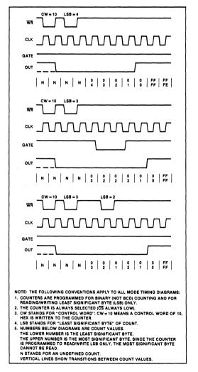
pulses after any trigger. The one-shot pulse can be repeated without rewriting the same count into the counter. GATE has no effect on OUT.
