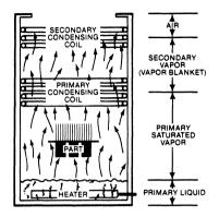
Fig 4—To meet high-volume production needs, vaporphase reflow soldering bonds LCCs to a substrate through the use of dried solder paste. Within the soldering chamber, the populated substrate absorbs heat in the primary saturated-vapor region and reflows the solder joints. Lifting the substrate into the secondary-vapor region cools, dries and cleans the soldered assembly.
