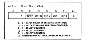
Figure 8, Read-Back Command Format
