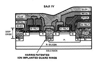
The next generation process was SAJI IV. SAJI IV features the selection oxidation and planar surface characteristics of SAJI III while adding further device scaling with the option of high resistivity substrates which reduces internal junction capacitances and increases speed. Self-aligned implanted P+ and N+ guardbands were also added, which increased the isolation between devices and reduced adjacent device interaction and increased packing density.
