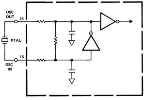
FIGURE 14 - Oscillator input schematic
