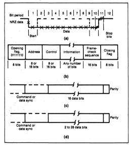
The data formats of UARTS (a), protocol controllers (b), and Manchester encoder-decoders (c and d) differ vastly, each offering advantages for different applications. The HD-6408 and HD-15530 (c) have a fixed, 16-bit word length, whereas the HD-15531 (d) has a programmable word length.
