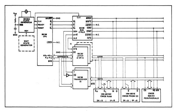
Figure 5b. Maximum Mode 80C86 Typical Configuration
