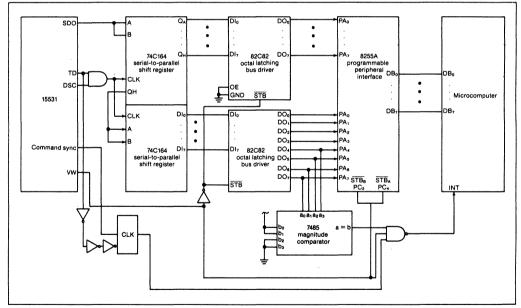
5. A receiver circuit built around the 15531 uses 74C164 shift registers for serial-to-parallel conversion. The 82C82 latching bus drivers and the 7485 magnitude comparator provide hard-wired address recognition. As with the receiver, an 8255A acts as the interface to the controller.
