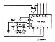
FIGURE 3 19200 Baud Operation
