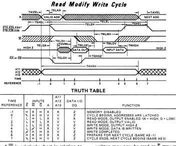
If the pulse width of  $\overline{W}$  is relatively short in relation to that of  $\overline{E}$ , a combination read write cycle may be performed. If  $\overline{W}$  remains high for the first part of the cycle, the output will become active during time (T = 1) provided  $\overline{G}$  is low. Data out will be valid during time (T =2). After the data is read,  $\overline{W}$  can go low. After minimum TWLWH,  $\overline{W}$  may return high. The information just
