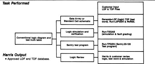
Design verification is next conducted using the TEGAS
