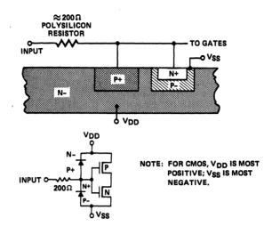
Figure 3 – Junction isolated dual-diode protection networks are most commonly used in today's CMOS circuits.
