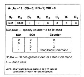
Figure 7, Counter Latch Command Format
