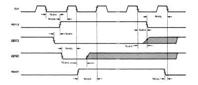
FIGURE 5. WAVEFORMS FOR READY SIGNALS (FOR ASYNCHRONOUS DEVICES)
