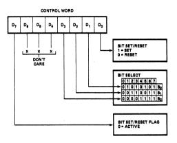
Figure 5 Bit Set/Reset Format
