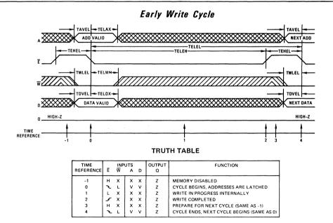
The early write cycle is the only cycle where the output is guaranteed not to become active. On the falling edge of  $\overline{E}$  (T = 0), the addresses, the write signal, and the data input are latched in on chip registers. The logic value of  $\overline{W}$ at the time  $\overline{E}$  falls determines the state of the output buffer for that cycle. Since  $\overline{W}$  is low when  $\overline{E}$  falls, the output buffer is latched into the high impedance state and
