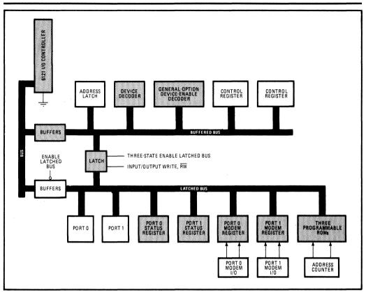
3. C-MOS to the rescue. When the DP278 communications controller for the DECmate was using too much power, consumption was cut from 6 to 4 watts by using the C-MOS 6121 I/O controller chip and replacing 16 TTL chips with 14 C-MOS chips (tinted).
