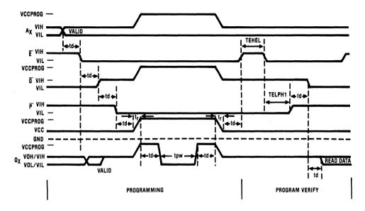
Figure 3 — Programming and Verify Cycle
