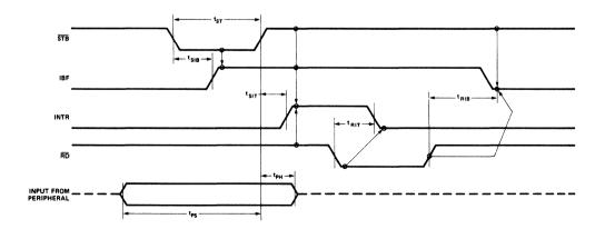
Figure 7 MODE 1 (Strobed Input)
