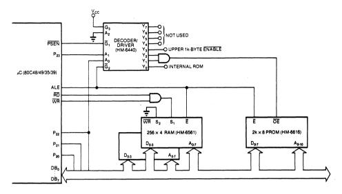
Fig 5—Memory expansion for single-chip μCs doesn't necessarily introduce a large power penalty. This design applies to systems using the CMOS or NMOS versions of the 8048 as well as other 8048-family members.
