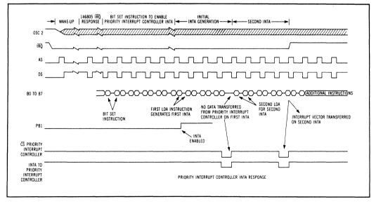
Fig 5 Timing diagram of microprocessor response to a wake-up interrupt. Any of several interrupts can initiate the wake-up response.
