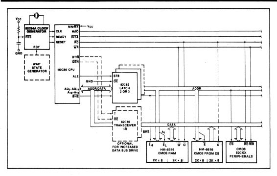
Figure 5a. Minimum Mode 80C86 Typical Configuration
