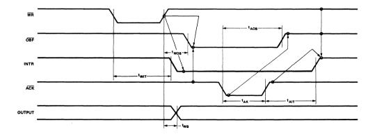
Figure 9 MODE 1 (Strobed Output) Combinations of MODE 1: Port A and Port B can be individually defined as input or output in Mode 1 to support a wide variety of strobed I/O applications.
