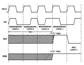
NOTE: Manchester Data In is not synchronous with Decoder Clock, Decoder Clock is synchronous with decoded NRZ out of SDO.
