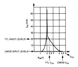
Fig 1—CMOS-memory operating current varies widely over device operating-voltage range. Standby current is at a minimum when  $V_{IN}$  is at either power-supply rail. Note the difference in operating current associated with the  $V_{OH}$ (highest output-voltage level) for TTL and CMOS.
