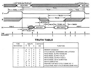
If the pulse width of  $\overline{W}$  is relatively short in relation to that of  $\overline{E}$  a combination read-write cycle may be performed. If  $\overline{W}$  remains high for the first part of the cycle, the outputs will become active during time (T = 1). Data out will be valid during time (T = 2). After the data is read,  $\overline{W}$  can go low. After minimum TWLWH,  $\overline{W}$  may return high. The
