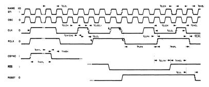
NOTE: ALL TIMING MEASUREMENTS ARE MADE AT 1.5 VOLTS, UNLESS OTHERWISE NOTED.
