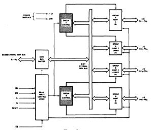
Figure 2 82C55A Block Diagram Showing Group A and Group B Control Functions
