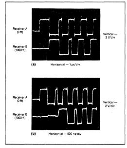
Oscilloscope photos of the network controller's receiver output show waveforms taken at data rates of 1 Mbit/s (a) and 2.5 Mbits/s (b). Although distortion is slightly greater at the higher data rate, the difference is virtually insignificant.
