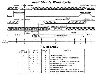
The read modify write cycle begins as all other cycles on the falling edge of  $\overline{E}$  (T= 0). The  $\overline{W}$  line should be high at (T = 0) in order to latch the output buffers in the active state. During (T = 1) the output will be active but not valid until (T = 2). On the falling edge of the  $\overline{W}$  (T = 3) the data present at the output and input are latched. The
