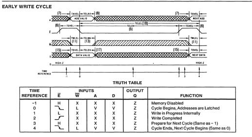
The early write cycle is the only cycle where the output is guaranteed not to become active. On the falling edge of  $\overline{E}$  (T = 0), the addresses, the write signal, and the data input are latched in on chip registers. The logic value of  $\overline{W}$  at the time  $\overline{E}$  falls determines the state of the output buffer for that cycle. Since  $\overline{W}$  is low when  $\overline{E}$  falls, the output buffer is latched into the high impedance state and will remain in that
