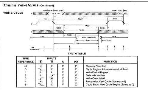
The write cycle is initiated by the falling edge of  $\overline{E}$  (T = 0), which latches the address information in the on-chip registers. There are two basic types of write cycles, which differ in the control of the common data-in/data-out bus.
