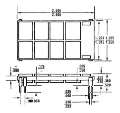
NOTE: All Dimensions are  $\frac{\text{Min}}{\text{Max}}$  , Dimensions are in inches.
