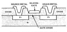
FIGURE 3. SILICON-GATE PFET STRUCTURE CROSS-SECTION SHOWS THE HEAVILY DOPED SOURCE AND DRAIN REGION. THEY ARE SEPARATED BY THE NARROW GAP OVER WHICH LIES A THIN-GATE OXIDE AND GATE MATERIAL.
