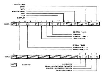
FIGURE 2. STATUS AND CONTROL REGISTER BIT FUNCTIONS
