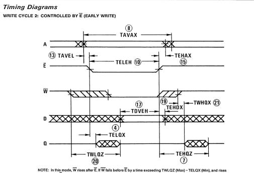
NOTE: In this mode, W rises after E. If W falls before E by a time exceeding TWLQZ (Max) - TELQX (Min), and rises after E by a time exceeding TEHQZ (Max) - TWHQZ (Min), then Q will remain in the high impedance state throughout the cycle. The address must remain stable whenever E and W are both low.
