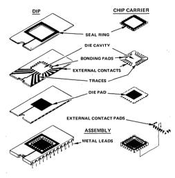
FIGURE 1. EXPLODED VIEW OF CHIP CARRIER AND DIP
