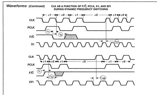
NOTE: This is an asynchronous input. The setup and hold times are required to guarantee the response shown.
