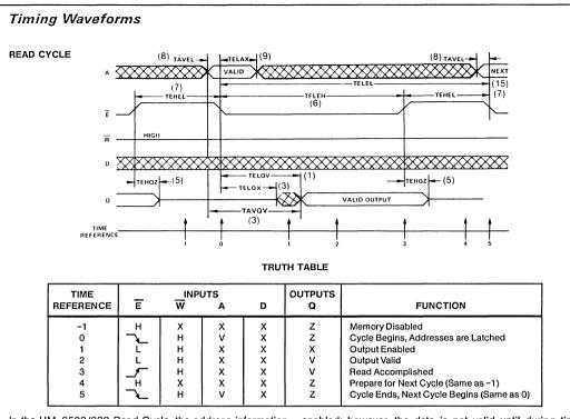
In the HM-6508/883 Read Cycle, the address information is latched into the on chip registers on the falling edge of  $\overline{E}$  (T = 0). Minimum address setup and hold time requirements must be met. After the required hold time, the addresses may change state without affecting device operation. During time (T = 1) the data output becomes
