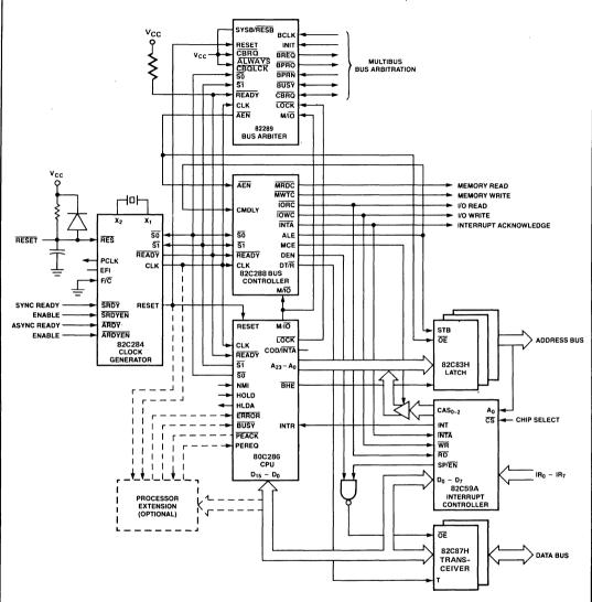
FIGURE 32. MULTIBUS SYSTEM BUS INTERFACE
