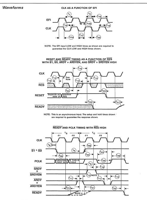
NOTES: 1. This is an asynchronous input. The setup and hold times shown are required to guarantee the response shown.
