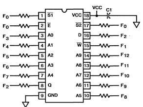
All Resistors  $47k\Omega \pm 5\%$   $F_0 = 100kHz \pm 10\%$   $F_1 = F_0 + 2, F_2 = F_1 + 2, F_3 = F_2 + 2 \cdot \cdot \cdot F_{12} = F_{11} + 2$ VCC = 5.5V  $\pm 0.5V$ VIH = 4.5V  $\pm 10\%$ VIL = -0.2V to +0.4V C1 = 0.01 \mu F Min. 3
