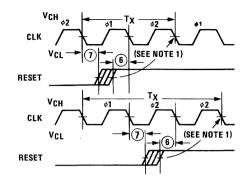
NOTE: When RESET meets the setup time shown, the next CLK will start or repeat ¢2 of a processor cycle.
