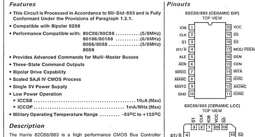
The Harris 82C88/883 is a high performance CMOS Bus Controller manufactured using a self-aligned silicon gate CMOS process (Scaled SAJI IV). The 82C88/883 provides the control and command timing signals for 80C86, 80C88, 8086, 8088, 8089, 80186, and 80188 based systems. The high output drive capability of the 82C88/883 eliminates the need for additional bus drivers.
