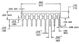
LEAD MATERIAL: Type B LEAD FINISH: Type A PACKAGE MATERIAL: Ceramic, 90% Alumina PACKAGE SEAL: Material: Glass Frit Temperature: 450°C ± 10°C Method: Furnace Seal
