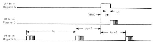
$\label{eq:tp1} \begin{array}{l} \mbox{tp1} = \mbox{Periodic Interrupt Time Interval (500 ms, 250 ms, 125 ms, 62.5 ms, etc. per Table 5)} \\ \mbox{tUC} = \mbox{Update Cycle Time (248 $\mu$s or 1984 $\mu$s)} \\ \mbox{tBUC} = \mbox{Delay Time Before Update Cycle (244 $\mu$s)} \\ \mbox{92CS-42706} \end{array}$
