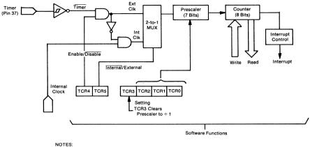
1. Prescaler and 8-bit counter are clocked falling edge of the internal clock (AS) or external input
