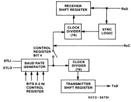
Fig. 6 - Transmitter receiver clock circuits.
