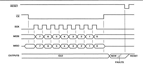
FIGURE 3. BYTE TIMING WITH ASYNCHRONOUS RESET
