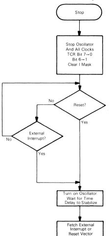
Fig. 16 - Stop function flowchart.
