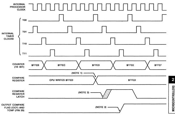
NOTES: 1. The CPU write to the compare register may take place at any time, but a compare only occurs at timer state T01. Thus, a 4-cycle difference may exist between the write to the compare register and the actual compare.
