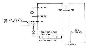
Fig. 3 - Power-sensing functional diagram.
