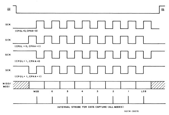
Fig. 21 – Data Clock Timing Diagram
