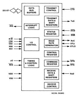
Fig. 1 - CDP65C51/51A interface diagram
