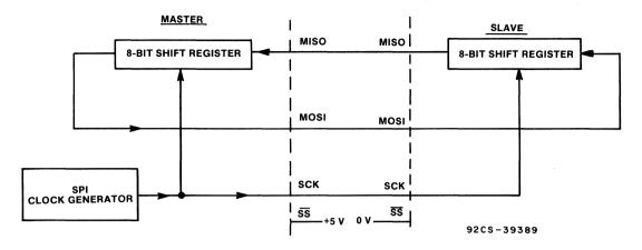
Fig. 23 - Serial Peripheral Interface Master-Slave Interconnection
