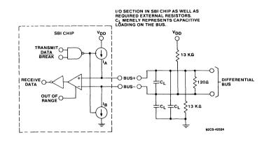
Fig. 4 - Differential Driver/Receiver.
