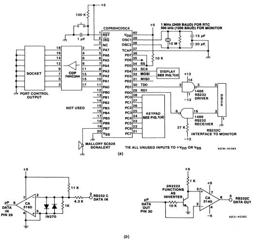
Fig. 1 - (a) Evaluation hardware. Keypad, display, port A control, and Sonalert not needed for CDP68HC05C4 monitor. RS-232 interface optional for real-time controller. (b) Alternative RS-232C interface.
