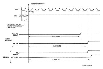
Fig. 4 - 6402-type receiver timing differences.
