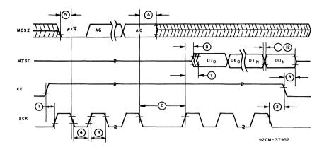
Fig. 15 - READ-cycle timing waveforms.
