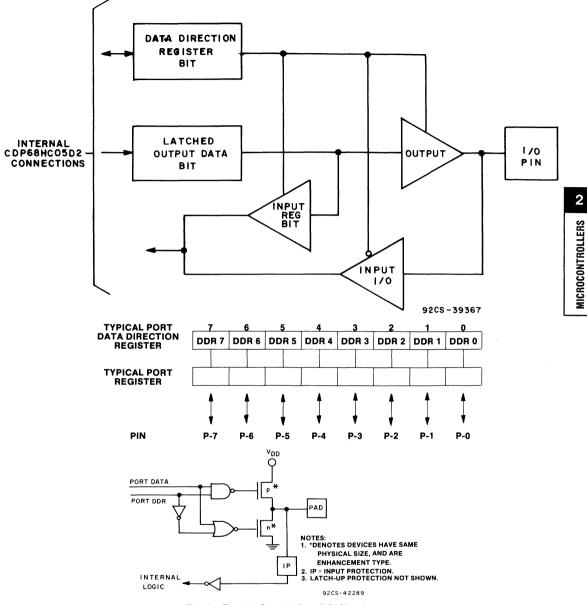
Fig. 3 – Typical Parallel Port I/O Circuitry
