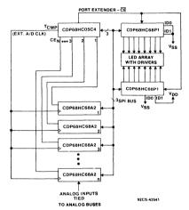
Fig. 9 - Digital storage scope with added A/D converters.
