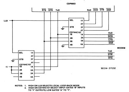
Fig. 22 - Loop-back circuit schematic.
