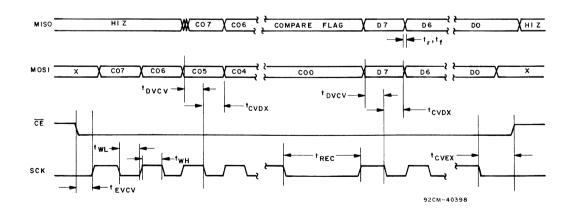
Fig. 8 - Write cycle timing waveforms.
