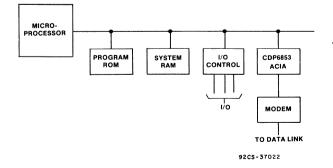
Fig. 21 – Simplified system diagram.
