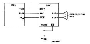
Fig. 9 - Using the SCI mode.
