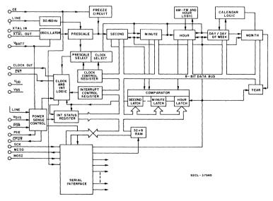
Fig. 1. - CDP68HC68T1 functional block diagram.
