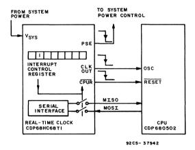
Fig. 4 - Power-down functional diagram.
