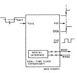
Fig. 10 - Power-up functional diagram (initiated by a rise in voltage on the  $V_{\text{sys}}$  pin).
