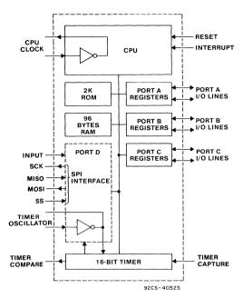
Fig. 1 - CDP68HC05D2 block diagram showing Serial Peripheral Interface portion of Port D.
