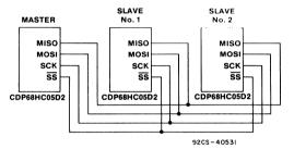
Fig. 10 - Single-master, multicomputer system with common slave-select interconnection.
