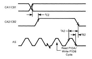
Fig. 6 - Control timing diagrams.
