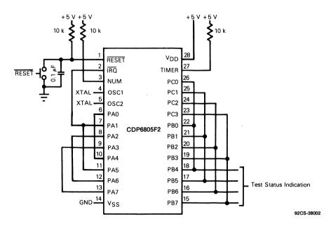
Fig. 10 - Self-check pinout configuration.
