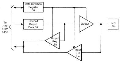
Fig. 8 - Typical port I/O circuitry.
