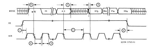
Fig. 14 - WRITE-cycle timing waveforms.
