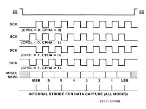
Fig. 4 - Data-clock timing diagram.
