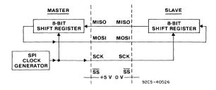
Fig. 3 - Serial Peripheral Interface master/slave interconnection.
