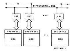
Fig. 2 - Possible network configuration - various microcomputers using SBI chips to communicate along differential bus.
