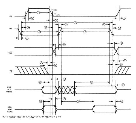
Fig. 2 — CDP6818 bus timing waveforms.
