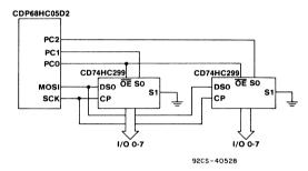
Fig. 7 - Increasing the number of output ports on a CDP68HC05D2 Microcomputer.
