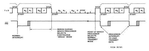
Fig. 18 - Transmit continuous "BREAK".
