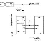
Fig. 6 - CDP68HC68T1 in circuit equipped with battery back-up.
