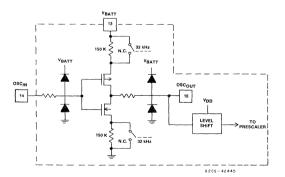
Fig. 23 - CDP68HC68T1 oscillator circuit. 150k resistor is placed in series with oscillator output only when 32+kHz is selected in clock control register.
