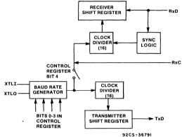
Fig. 7 - Transmitter receiver clock circuits.
