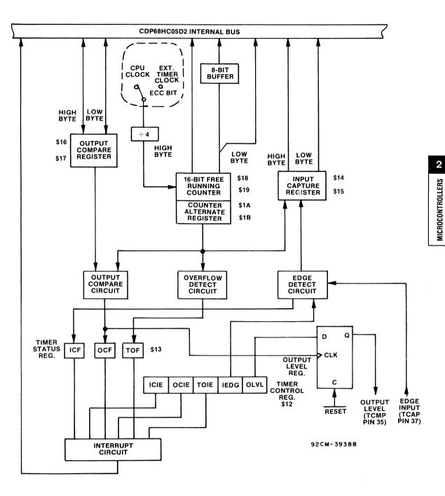
Fig. 15 - Programmable Timer Block Diagram
