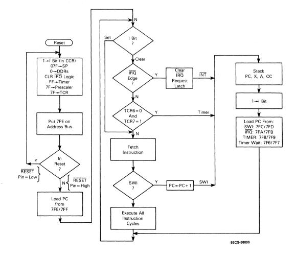
Fig. 14 - RESET and INTERRUPT processing flowchart.
