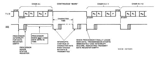
Fig. 9 - Transmit data register not loaded by processor.
