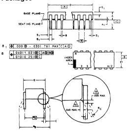
(D) SUFFIX (JEDEC MS-015-CB) 28 LEAD DUAL-IN-LINE SIDEBRAZED CERAMIC PACKAGE
