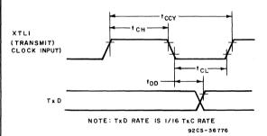
Fig. 23 - Transmit timing waveforms with external clock.
