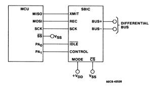
Fig. 10 - Using the SPI mode.
