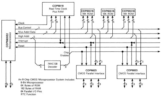
Fig. 9 - A typical CMOS microprocessor system.
