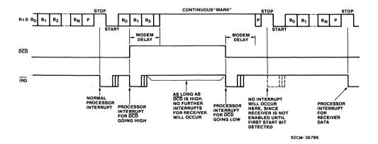
Fig. 17 - Effect of DCD on receiver.
