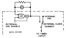
Fig. 14 - External Timer Oscillator Controls
