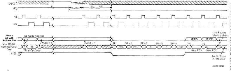
Represents the internal gating of the OSC1 input pin.  $t_{CVC}$  is one instruction cycle (for f\_OSC=5 MHz, t\_{CVC}=1  $\mu$ s)
