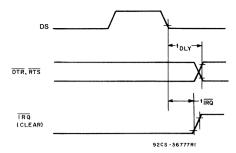
Fig. 27 - Interrupt- and output-timing waveforms.
