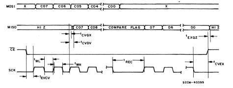
Fig. 9 - Read cycle timing waveforms.
