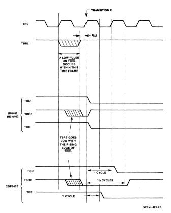
Fig. 3 - 6402-type transmitter timing differences.
