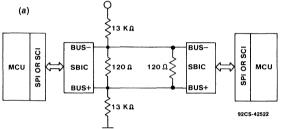
(a) Hardware configuration for a network consisting of two microcomputers. Notice that the pullup resistor is connected to the BUS- pin and the pulldown to BUS+.
