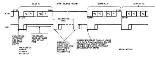
Fig. 10 - Transmit data register not loaded by processor.
