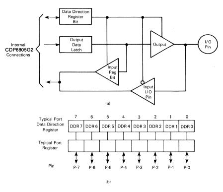
Fig. 9 – Typical port I/O circuitry.
