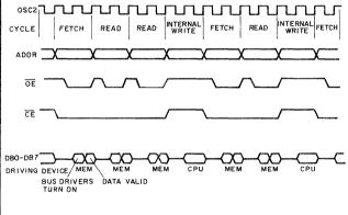
FIGURE 2. TYPICAL CYCLE TIMING FOR THE CDP68EM05C4 EMULATOR.
