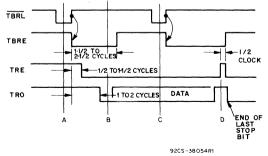
Fig. 3 - Transmitter timing waveforms.
