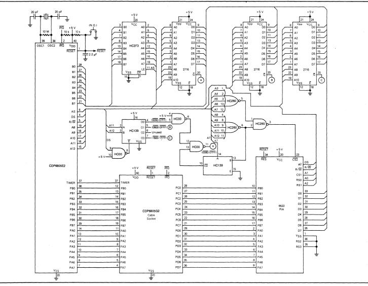
FIGURE 3 - CDP6805G2 Emulator Schematic Diagram
