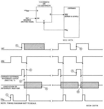
Fig. 3 - Conversion of edge and level-sensitive interrupts to edgeonly: required hardware and resulting timing.
