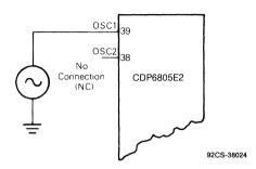
Fig. 10 - External clock connection.
