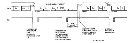
Fig. 19 - Receive continuous "BREAK".
