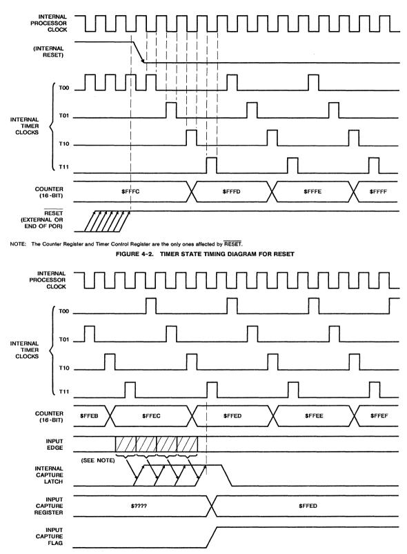
NOTE: If the input edge occurs in the shaded area from one timer state T10 to the other timer state T10 the input capture flag is set during the next state T11. FIGURE 4-3. TIMER STATE TIMING DIAGRAM FOR INPUT CAPTURE
