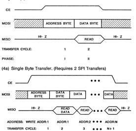
(4b) Multiple (N) byte Transfer. (Efficient Device Communication Requiring N+1 SPI Transfers)
