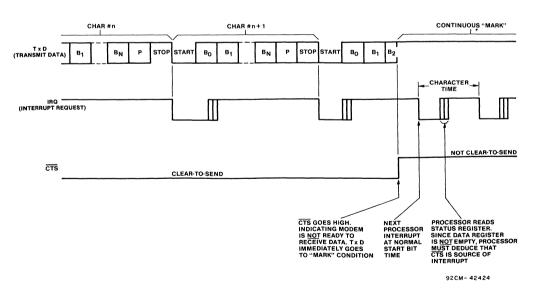
Fig. 8 - Effect of CTS on transmitter (CDP65C51).
