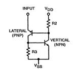
FIGURE 5. IMPROPER BIASING CAN LATCH-UP THIS SCR CONFIGURATION.
