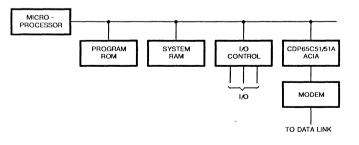
Fig. 20 - Simplified system diagram.
