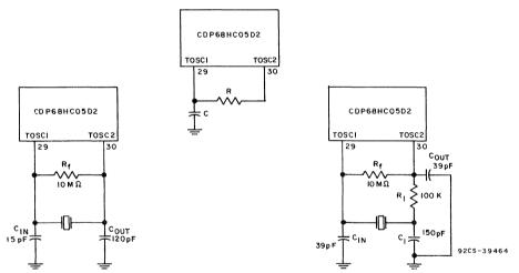
(b) Crystal Oscillator connections for crystal speeds above approx. 400 KHz. The C<sub>in</sub> and C<sub>out</sub> values may vary depending upon crystal manufacturer.
