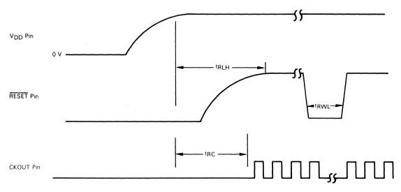
Fig. 7 — Power-up timing waveforms.
