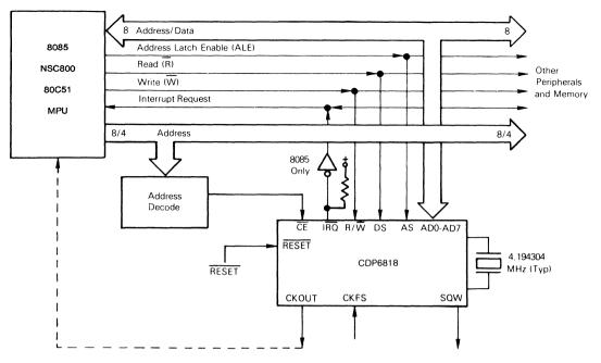
Fig. 18 — CDP6818-interfaced to competitor compatible multiplexed bus microprocessors.
