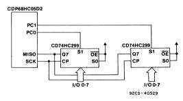
Fig. 8 - Increasing the number of input ports on a CDP68HC05D2 Microcomputer.
