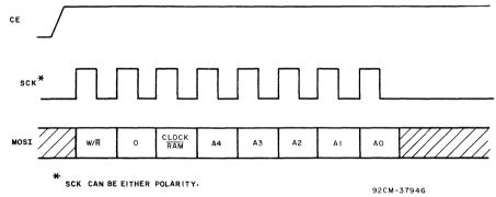
Fig. 9 - Address/Control byte-transfer wavefurms.
