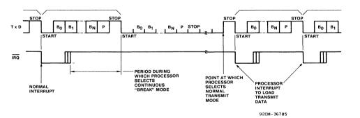
Fig. 19 - Transmit continuous "BREAK".
