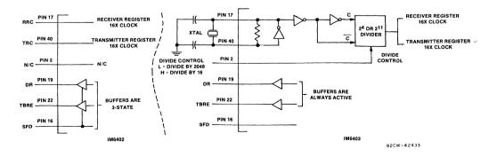
Fig. 5 - Functional difference between IM6402 and IM6403 UART - IM6403 has on-chip 4/11 stage divider.
