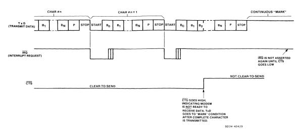
Fig. 9 - Effect of CTS on transmitter (CDP65C51A).
