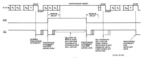
Fig. 16 - Effect of DCD on receiver.
