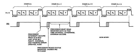
Fig. 9 - Continuous data receive.
