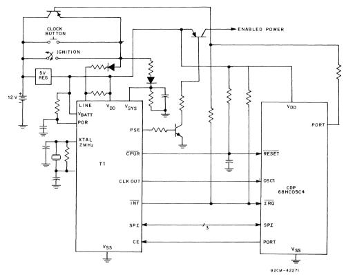
Example of an automotive system. The Vsvs and LINE inputs can be used to sense the ignition turning on and off. An external switch is included to activate the system without turning on the ignition. Also, the CMOS CPU is not powered down with the system V<sub>DD</sub>, but is held in a low power reset mode during power down. When restoring power the CDP68HC68T1 will enable the CLK OUT pin and set the PSE and CPUR high.
