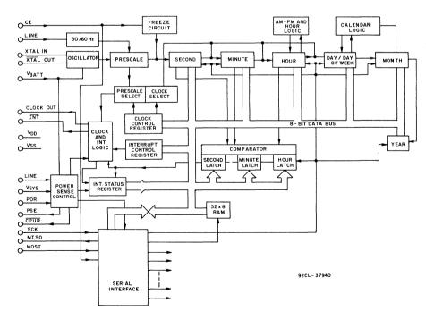
Figure 1 - Real-time clock functional diagram
