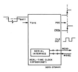
Fig. 6 - Power-up functional diagram (initiated by a rise in voltage on the "V<sub>SYS</sub>" pin).
