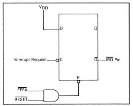
FIGURE 2 - Edge-Sensitive Interrupt Circuit, Schematic Diagram
