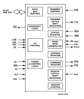
Fig. 1 – CDP6853 interface diagram.
