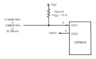
Fig. 10 — External Time-base connection.
