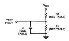
FIGURE 9.1. EQUIVALENT TEST LOAD
