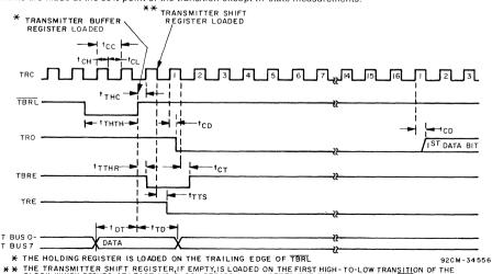
★ THE TRANSMITTER SHIFT REGISTER, IF EMPTY, IS LOADED ON THE FIRST HIGH-TO-LOW TRANSITION OF THE CLOCK WHICH OCCURS AT LEAST 1/2 CLOCK PERIOD + 1THC ATTER THE TRAILING EDGE OF TBRL AND TRANSMISSION OF A START BIT OCCURS 1/2 CLOCK PERIOD + 1CD LATER
