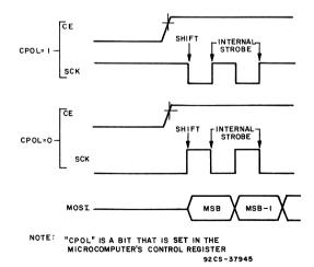
Fig. 8 - Serial RAM clock (SCK) as a function of MCU clock polarity (CPOL).
