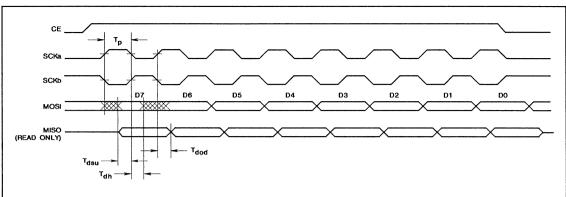
FIGURE 3. TIMING DIAGRAM FOR SERIAL PERIPHERAL INTERFACE
