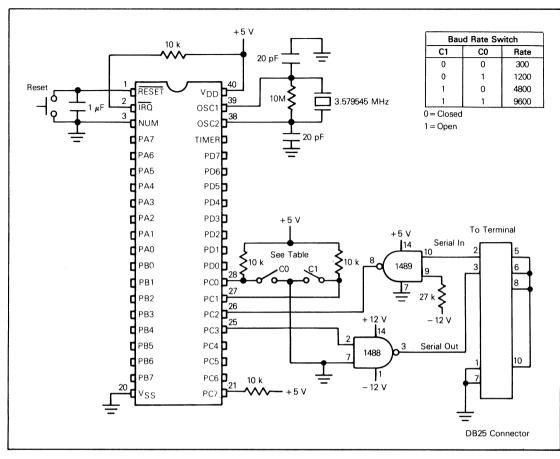
Fig. 1 - Monitor mode schematic diagram.
