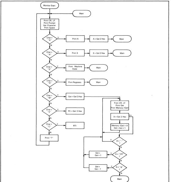
Fig. 2 - Monitor mode operating flowchart.
