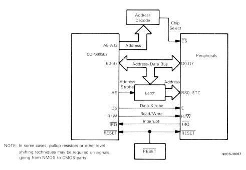
Fig. 21 - Connection to peripherals.
