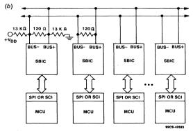
(b) Hardware configuration for a network consisting of 3 or more MCU's. Notice that the bus utilizes no more than 1 set of 13K bias resistors and no more than two 120Ω termination resistors.
