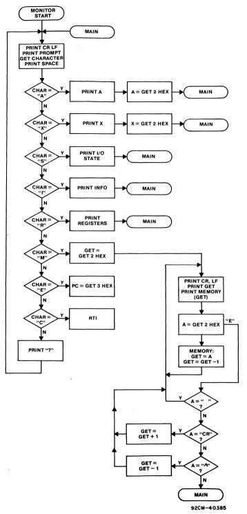
Fig. 2 - Flowchart of the monitor-mode program.
