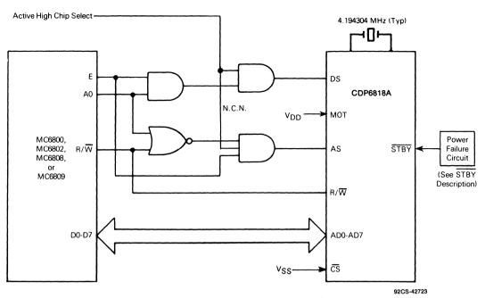
Fig. 20 - CDP6818A interfaced with Motorola Processors.
