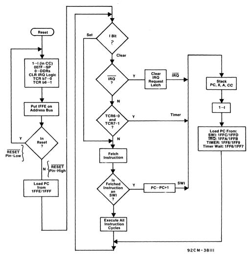
Fig. 2 - RESET and INTERRUPT processing flowchart (CDP6805G2).
