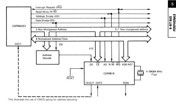
Fig. 19 - CDP6818 interface to CDP6805E2 CMOS multiplexed microprocessor with slow address decoding.
