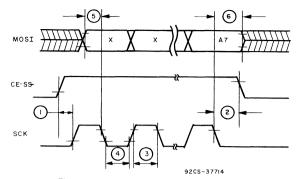
Fig. 6 - Page/Device byte timing waveforms.
