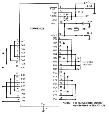
Fig. 10 - Self-check circuit.
