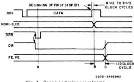
Fig. 4 - Receiver timing waveforms.
