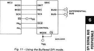
Fig. 11 - Using the Buffered SPI mode.
