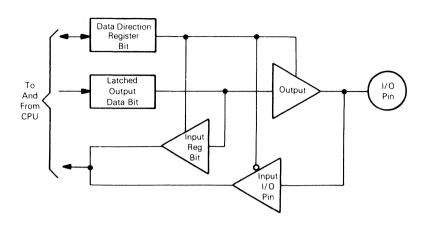
Fig. 11 - Typical I/O port circuitry
