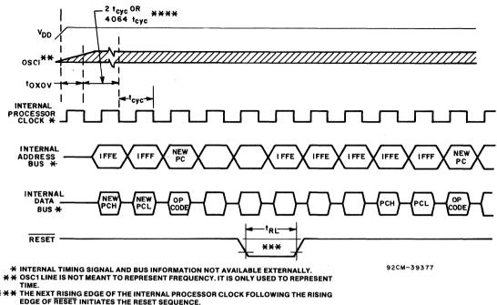
\*\*\*\* DELAY IS MASK PROGRAMMABLE. (REFER TO THE SECTION DESCRIBING POWER-ON-RESET IN THE RESETS INFORMATION OF THIS DATA SHEET).
