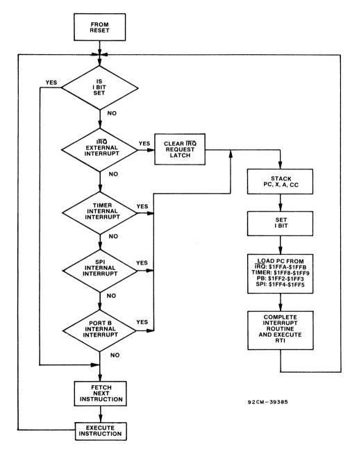
Fig. 9 - Hardware Interrupt Flowchart
