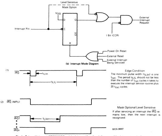
Fig. 1 - External interrupt (CDP6805G2): (a) interrupt functional diagram, (b) interrupt mode diagram.
