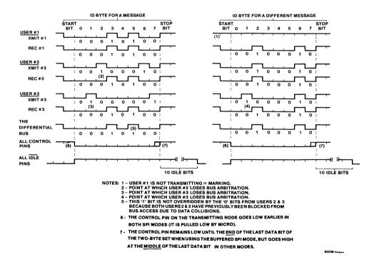
Fig. 6 - Example of the SBI chip operating during bus arbitration.
