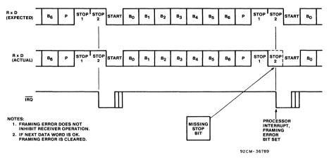
Fig. 16 - Framing error.
