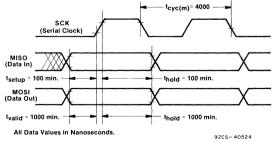
Fig. 13(b) - SPI control timing diagram for the CDP68HC05D2 Microcomputer. SPI configured as master with serial clock control bits set for CPOL, CPHA = 0, 0 at a baud rate of 250 kilobits per second.
