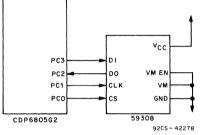
Fig. 9 - CDP6805G2 I/O lines used to simulate a serial bus and communicate with NCR 59308 64 x 16-bit EEPROM.
