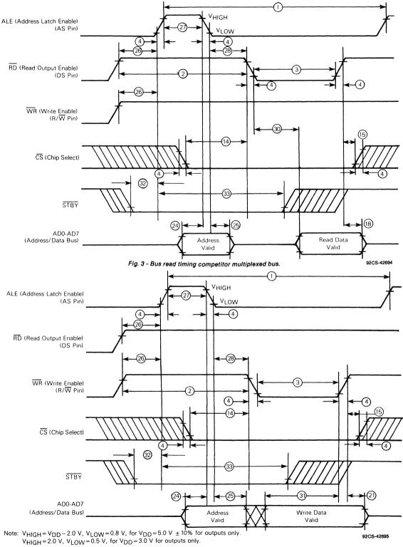
Fig. 4 - Bus write timing competitor multiplexed bus.
