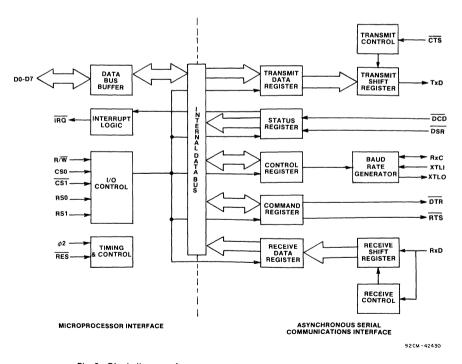
Fig. 2 - Block diagram of a representative second-generation UART, the CDP65C51.
