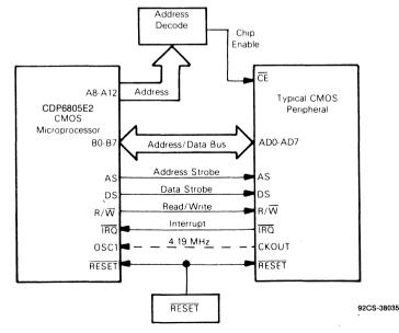
Fig. 20 - Connection to CMOS peripherals.
