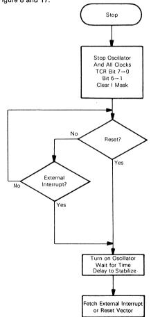
Fig. 17 - Stop function flowchart
