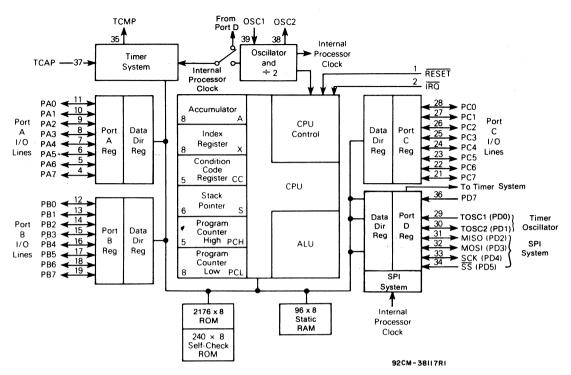
Fig. 1 — CDP68HC05D2 CMOS microcomputer block diagram.
