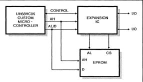
CS = CONTROL D = DATA AH = HIGH ORDER ADDRESS BYTE AL = LOW ORDER ADDRESS BYTE
