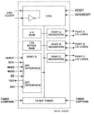
Fig. 4 - Block diagram of CDP68HC05C4.
