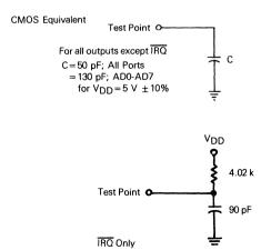
Fig. 2 - Equivalent test loads.
