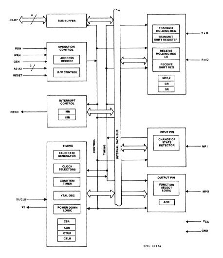
Fig. 13 - Functional block diagram of the IM26C91.
