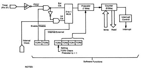
Prescaler and 8-bit counter are clocked falling edge of the internal clock (AS) or external
