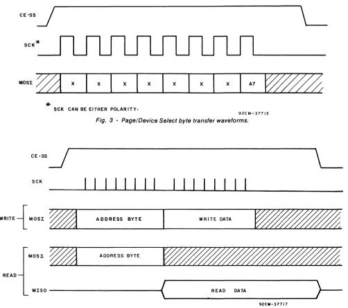
Fig. 4 - Single-byte transfer.
