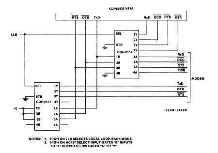
Fig. 21 - Loop-back circuit schematic.
