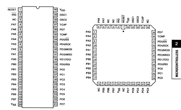
D Suffix - 40-Lead Dual-In-Line Side-Brazed Ceramic Package E Suffix - 40-Lead Dual-In-Line Plastic Package
