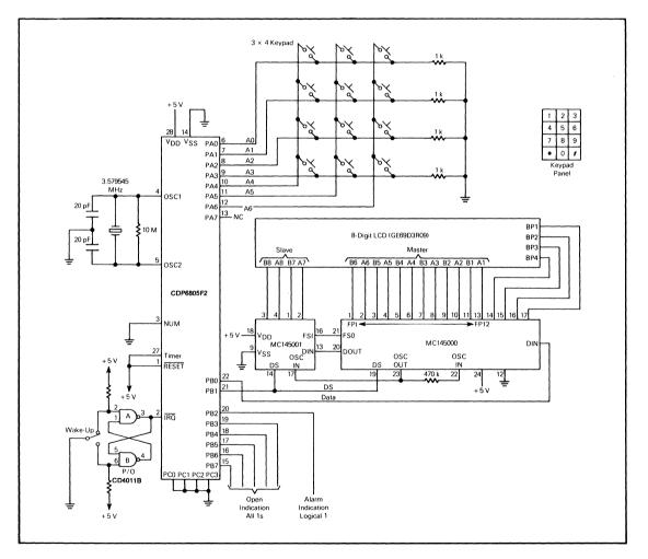
Fig. 1 - Digital lock system schematic diagram.
