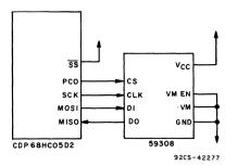
Fig. 5 - CDP68HC05D2 microcomputer interfaced to NCR 59308 64 x 16-bit EEPROM.
