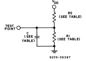
Fig. 24 - Equivalent Test Load
