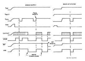
Fig. 8 - Timing diagram showing outputs controlled by V<sub>SYS</sub>, interrupts, and power-down instruction.
