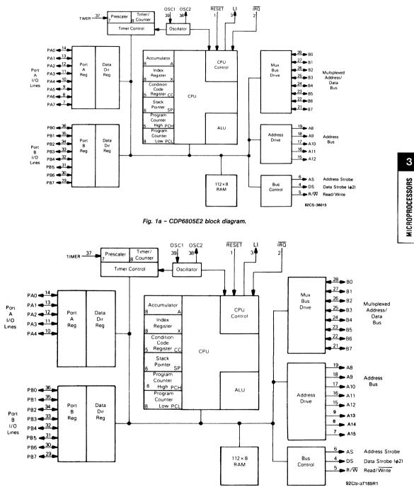
Fig. 1b - CDP6805E3 block diagram.
