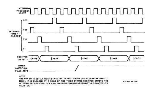
Fig. 19 - Timer State Diagram For Timer Overflow
