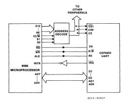
Fig. 12 - Interfacing the CDP6853 to an 8085 microprocessor (Intel type bus).
