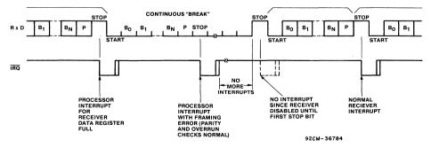
Fig. 20 - Receive continuous "BREAK".
