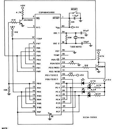
THE RC OSCILLATOR OPTION MAY ALSO BE USED IN THIS CIRCUIT
