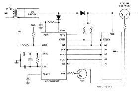
Fig. 3 - The real-time clock interfaced to an MPU.
