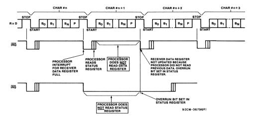
Fig. 12 - Effect of overrun on receiver.
