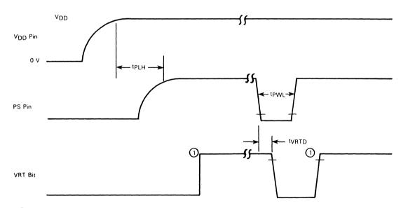
(1) The VRT bit is set to a "1" by reading Register d. The VRT bit can only be cleared by pulling the PS pin low (see REGISTER D (\$0D)).
