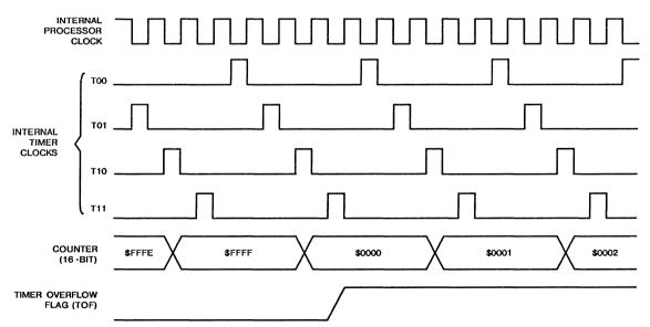
NOTE: The TOF bit is set at timer state T11 (transition of counter from \$FFFF to \$0000). It is cleared by a read of the timer status register during the internal processor clock high time followed by a read of the counter low register.
