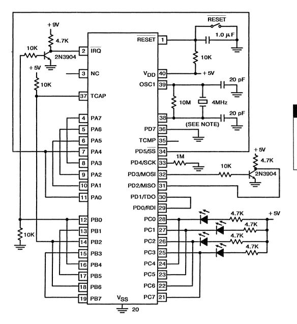
NOTE: The RC Oscillator Option may also be used in this circuit.
