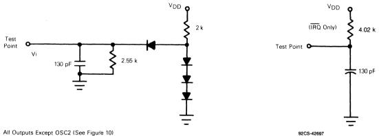
Fig. 6 - TTL equivalent test load.
