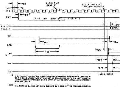
★ IF A PENDING DA HAS NOT BEEN CLEARED BY A READ OF THE RECEIVER HOLDING REGISTER BY THE TIME A NEW WORD IS LOADED INTO THE RECEIVER HOLDING REGISTER, THE OE SIGNAL WILL COME TRUE.
