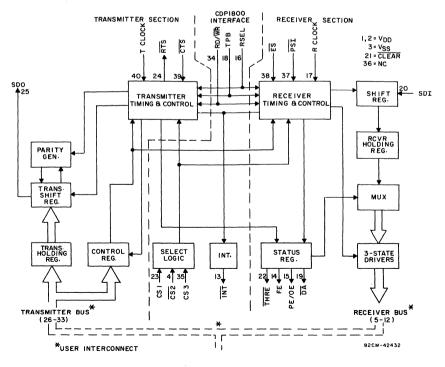
Fig. 6 - Block diagram of the CDP1854A in Mode 1.
