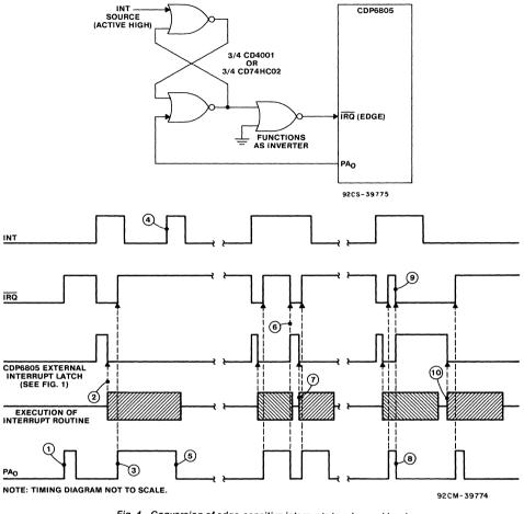
Fig. 4 - Conversion of edge-sensitive interrupts to edge and levelsensitive interrupts: required hardware and resulting timing.
