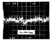
FIGURE 1. HFA1105 NOISE PERFORMANCE,  $A_V = +2$ ,  $R_F = 510\Omega$
