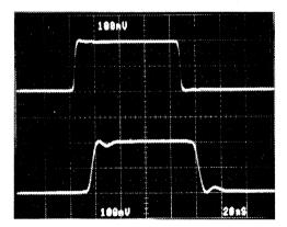
$\label{eq:FIGURE 4. SMALL SIGNAL RESPONSE} \end{tabular} Vertical Scale: $V_{IN}$ = 100mV/Div., $V_{OUT}$ = 100mV/Div. Horizontal Scale: $20ns/Div. $$Point of the statement o$
