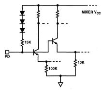
FIGURE 35. ENABLE PIN INPUT CIRCUIT
