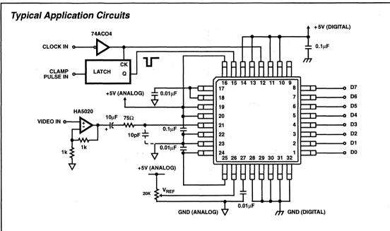
FIGURE 15. INPUT CLAMP APPLICATION (INTERNAL REFERENCE USED)
