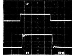
FIGURE 5. LARGE SIGNAL RESPONSE Vertical Scale:  $V_{IN}$  = 1V/Div.,  $V_{OUT}$  = 1V/Div. Horizontal Scale: 50ns/Div.
