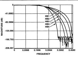
FIGURE 10. COMPOSITE RESPONSE OF FIXED COEFFICIENT HALFBAND FILTERS
