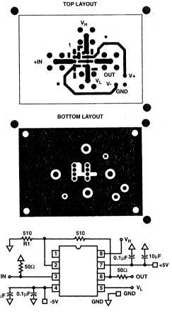
FIGURE 4. EVALUATION BOARD SCHEMATIC AND LAYOUT
