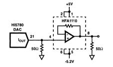
FIGURE 5. HIGH SPEED CURRENT TO VOLTAGE CONVERSION
