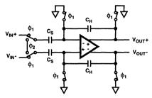
FIGURE 14. ANALOG INPUT SAMPLE-AND-HOLD
