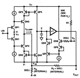
FIGURE 4. HFA1113 SIMPLIFIED VH CLAMP CIRCUITRY
