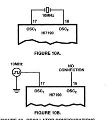
FIGURE 10. OSCILLATOR CONFIGURATIONS
