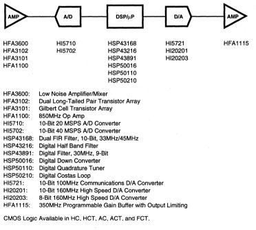
FIGURE 17. 10-BIT COMMUNICATIONS COMPONENTS
