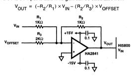
FIGURE 5. INVERTING BUFFER
