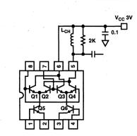
FIGURE 11. OUTPUT PORT S22 TEST SET UP
