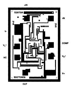
† Output Clamping Function (V<sub>H</sub>, V<sub>L</sub>) is available to users of the HFA1102 in die form. Please refer to the HFA1130 data sheet for infomation regarding the operation and use of this function. 2
