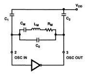
Where:  $C_M =$  Motional Capacitance  $L_M =$  Motional Inductance  $R_M =$  Motional Resistance  $C_0 =$  Shunt Capacitance
