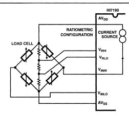
FIGURE 7. BURN-OUT CURRENT SOURCE CIRCUIT
