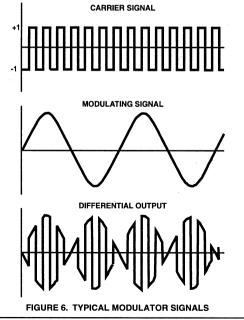
Figure 6 shows the typical input waveforms where the frequency of the carrier is higher than the modulating signal. The output waveform shows a typical suppressed carrier output of an up converter or an AM signal generator.
