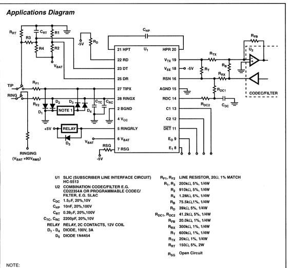
The anodes of D<sub>3</sub> and D<sub>4</sub> may be connected directly to the V<sub>BAT</sub> supply if the application is exposed to only low energy transients. For harsher environments it is recommended that the anodes of D<sub>3</sub> and D<sub>4</sub> be shorted to ground through a transzorb or surgector. TELECOMMUNI-CATIONS
