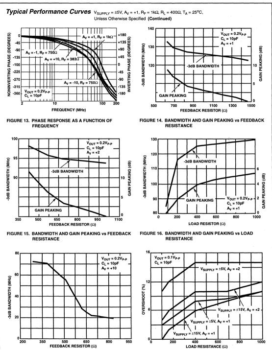
FIGURE 18. SMALL SIGNAL OVERSHOOT vs LOAD
