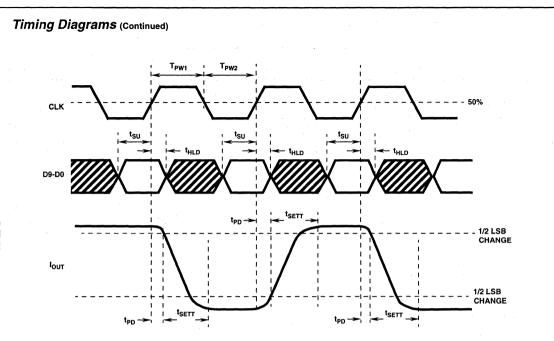
FIGURE 3. PROPAGATION DELAY, SETUP TIME AND MINIMUM PULSE WIDTH DIAGRAM
