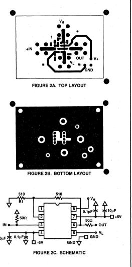
FIGURE 2. EVALUATION BOARD SCHEMATIC AND LAYOUT
