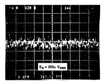
FIGURE 2. HFA1106 NOISE PERFORMANCE, UNCOMPENSATED,  $A_V = +2$ ,  $R_F = 100\Omega$
