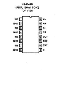
The HA4344B is a very wide bandwidth 4 x 1 crosspoint switch ideal for professional video switching, HDTV, computer display routing, and other high performance applications. This circuit features very low power dissipation, excellent differential gain and phase, high off isolation, symmetric slew rates, fast switching, and latched control signals. When disabled, the output is switched to a high impedance state, making the HA4344B ideal for matrix routers.
