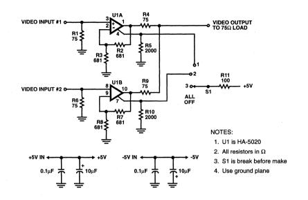
FIGURE 57. TWO CHANNEL HIGH IMPEDANCE MULTIPLEXER
