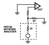
FIGURE 1. TEST CIRCUIT FOR TRANSIMPEDANCE MEASUREMENTS
