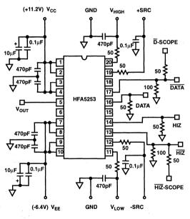
FIGURE 19. DECOUPLING CIRCUIT SCHEMATIC
