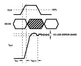
FIGURE 1. FULL SCALE SETTLING TIME DIAGRAM
