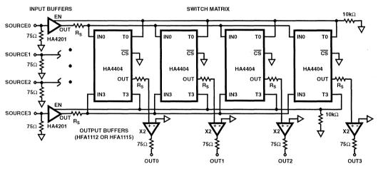
FIGURE 1. 4 x 4 SWITCHER/ROUTER APPLICATION
