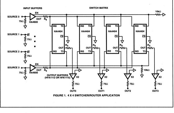
for the input buffer, the HA4404 as the switch matrix, and the HFA1112 (programmable gain buffer) as the gain of two output driver. Figure 2 details a 16 x 1 switcher (basically a 16:1 mux) which uses the HA4201 (1 x 1 crosspoint) and the HA4404 in a cascaded stage configuration to minimize capacitive loading at each output node, thus increasing system bandwidth.
