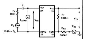
FIGURE 10. CURRENT GAIN -RSN TO METALLIC
