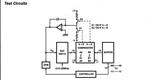
FIGURE 14. INTEGRAL AND DIFFERENTIAL NON-LINEARITY ERROR AND OFFSET VOLTAGE TEST CIRCUIT
