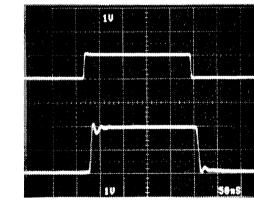
FIGURE 5. LARGE SIGNAL RESPONSE Vertical Scale: V<sub>IN</sub> = 1V/Div., V<sub>OUT</sub> = 1V/Div. Horizontal Scale: 50ns/Div.
