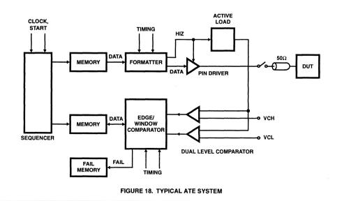
the DUT pin with digital signals. When the DUT pin acts as an output, the pin driver output will be in high impedance mode (HIZ) with a logic "1" applied to the "HIZ" pin. During this high impedance mode the pin driver presents a capacitance of less than 5pF to the DUT. Special care has to be taken to match the impedance (to  $50\Omega$ ) at the pin driver output to minimize reflections.
