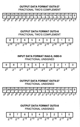
The MUX/Adder can be configured to implement programmable rounding at bit locations  $2^{-10}$  through  $2^1$ . The round is implemented by adding a 1 to the specified location (see Table 2). For example, to configure the part such that the output is rounded to the 10 MSBs, OUT18 - 27, the round position would be chosen to be  $2^{-1}$ .
