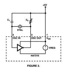
SPECIAL ANALOG CIRCUITS Typical values of the capacitors in Figure 2 are shown below. Some trial and error may be required before the best combination is determined. The values listed are total capacitance including parasitic or other sources. Remember that in the 10kHz to 100kHz frequency range setting the HA7210 switches in two internal 15pF capacitors.
