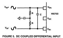
The resistors, R, in Figure 5 are not absolutely necessary but may be used as load setting resistors. A capacitor, C, connected from  $V_{IN+}$  to  $V_{IN-}$  will help filter any high frequency noise on the inputs, also improving performance. Values around 20pF are sufficient and can be used on AC coupled inputs as well.
