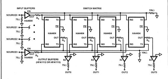
FIGURE 1. 4 x 4 SWITCHER/ROUTER APPLICATION
