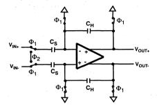
FIGURE 3. ANALOG INPUT SAMPLE-AND-HOLD
