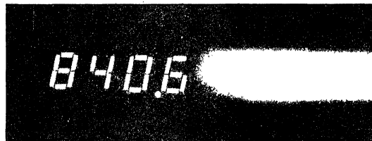
Figure 14. Effect of anti-reflection surface on an optical filter.
