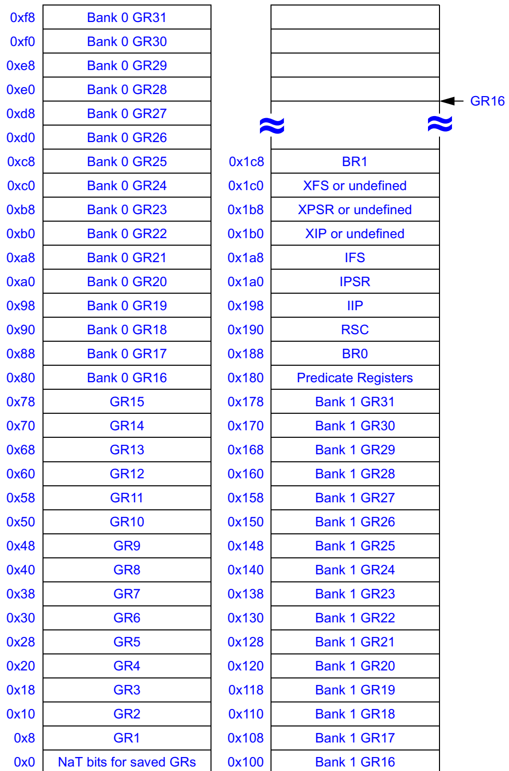
Figure 11-13. Processor State Saved in Min-state Save Area
