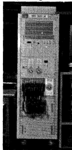
Fig. 3 Monitored temperature cycling tester
