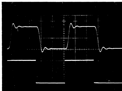
FIGURE 13. MF6-50 Step Input Response, Vertical = 2V/div., Horizontal = 1 ms/div., f_{CLK} = 100 kHz
