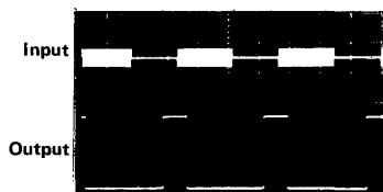
Response to 100mV RMS tone burst. R_L = 100 ohms.
