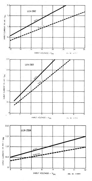
Figure 9 INPUT CURRENT AS A FUNCTION OF INPUT VOLTAGE
