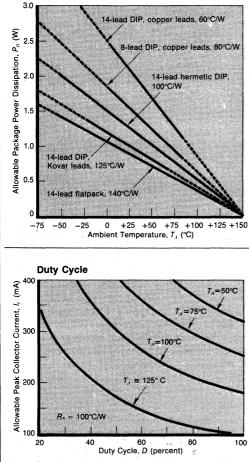
Typical thermal-resistance ratings for ICs in still air range from 60°C/W to 140°C/W. The slope of each curve on this graph is equal to the derating factor G $\theta$ , which is the reciprocal of thermal resistance R $\theta$ . For an ambient temperature of 50°C, a typical 14-lead flatpack with an R $\theta$  of 140°C/W can dissipate about 0.7 W. A typical DIP, however, with 14 copper-alloy leads can dissipate almost 1.7 W at 50°C.
