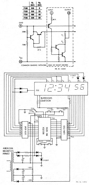
TYPICAL SIX-DIGIT CLOCK USING TYPE UDN-7183A
