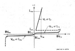
SCR ANODE CHARACTERISTICS WITH GATE CONNECTED TO CATHODE THROUGH RGK
