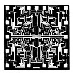
The Series ULN-4036A quad high-performance monolithic operational amplifiers are supplied in 14lead dual in-line packages conforming to JEDEC outline TO-116 (MO-001AA) and are rated for continuous operation over the temperature range of 0°C to +70°C.
