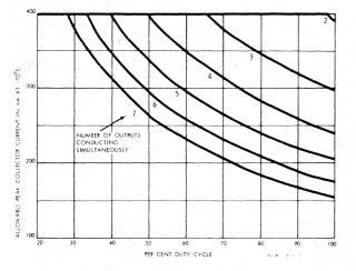
Figure 1 Collector current as a function of Duty cycle and number of outputs
