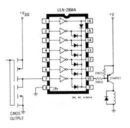
Figure 7 Type ULN-2004A SCHEMATIC AND APPLICATION
