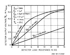
Figure 7 DETECTOR OUTPUT VOLTAGE AS A FUNCTION OF DETECTOR LOAD RESISTANCE
