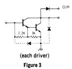
TYPE ULN-2001A SCHEMATIC
