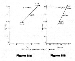
Figure 18B indicates the maximum  $V_{CE(sot)}$  changes as the current is increased from 300 mA to 500 mA. This information is necessary for calculations of package power dissipation if the system duty cycle presents questions of average power.
