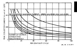
PEAK COLLECTOR CURRENT AS A FUNCTION OF DUTY CYCLE AND NUMBER OF OUTPUTS AT  $+ 125^{\circ}$ C
