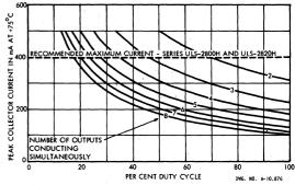
PEAK COLLECTOR CURRENT AS A FUNCTION OF DUTY CYCLE AND NUMBER OF OUTPUTS AT +75°C
