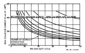
PEAK COLLECTOR CURRENT AS A FUNCTION OF DUTY CYCLE AND NUMBER OF OUTPUTS AT + 100°C
