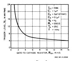
Figure 9 SCR TRIGGER LEVEL AS A FUNCTION OF GATE-TO-CATHODE RESISTANCE (RGK)
