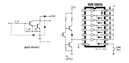
Figure 6 TYPE ULN-2003A SCHEMATIC AND APPLICATION
