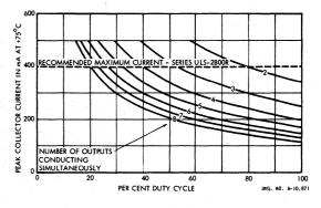
PEAK COLLECTOR CURRENT AS A FUNCTION OF DUTY CYCLE AND NUMBER OF OUTPUTS AT  $+75^{\circ}$ C
