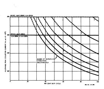
PEAK COLLECTOR CURRENT AS A FUNCTION OF DUTY CYCLE AND NUMBER OF OUTPUTS
