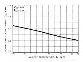
Figure 2 QUIESCENT POWER SUPPLY CURRENT DRAIN AS A FUNCTION OF AMBIENT OPERATING TEMPERATURE
