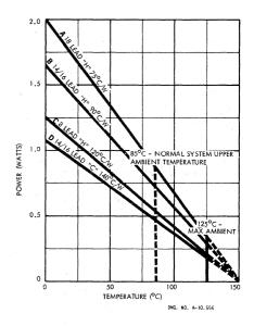
Figure 4 SIDE BRAZED CERAMIC AND FLAT PACK (Aerospace and Military)
