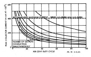
PEAK COLLECTOR CURRENT AS A FUNCTION OF DUTY CYCLE AND NUMBER OF OUTPUTS AT +125°C
