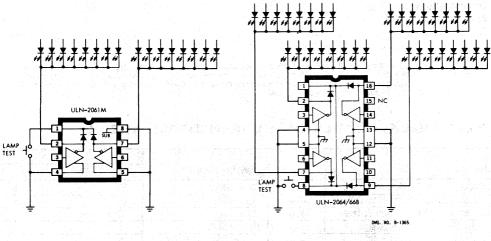
COMMON-CATHODE LED DRIVERS (Types ULN-2068/70B are also applicable)
