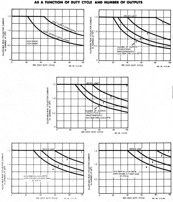
PEAK COLLECTOR CURRENT S & FUNCTION OF DUTY CYCLE, AND NUMBER OF OUTPUT
