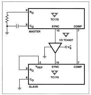
Figure 4 Master/Slave Parallel Operation
