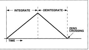
Figure 9 Dual-Slope Conversion
