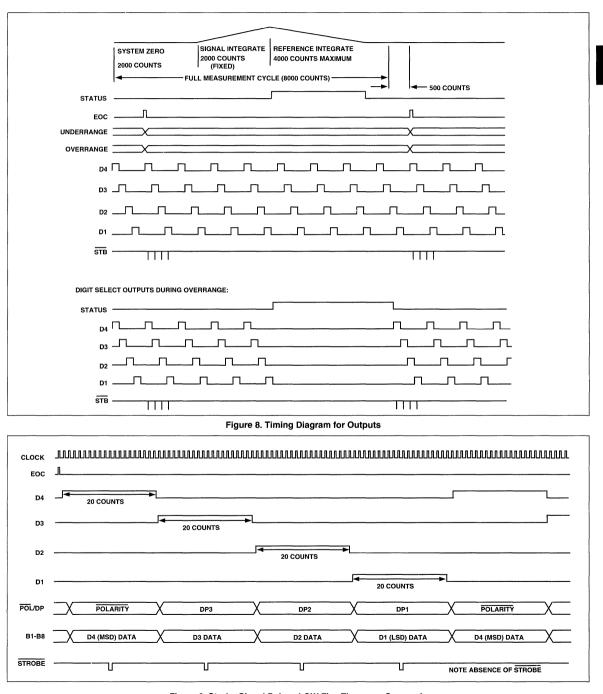
Figure 9. Strobe Signal Pulses LOW Five Times per Conversion
