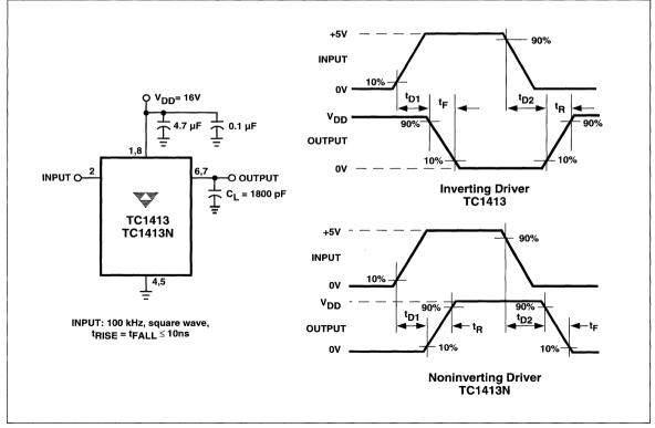
Figure 1. Switching Time Test Circuit
