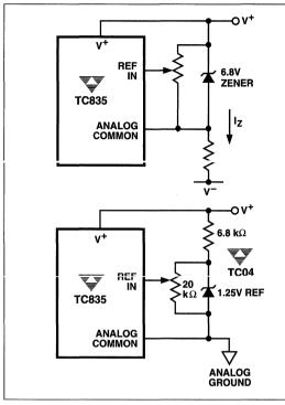
Figure 5 Using an External Reference
