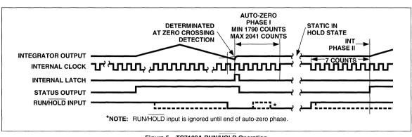
Figure 5 TC7109A RUN/HOLD Operation
