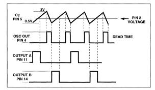
The 5K potentiometer sets a reference voltage at pin 2. When ramp voltage of pin 5 reaches this reference voltage, output drive pulse is active ON. Varying the discharge resistor will vary the dead time. Increasing the discharge resistor will effect an increase in the dead time.
