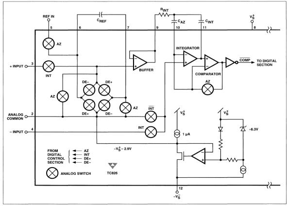
Figure 4 TC826 Analog Section
