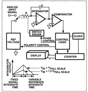
Figure 2. Basic Dual-Slope Converter
