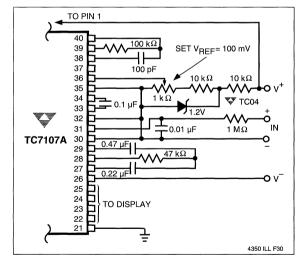
Figure 26 TC7107A With a 1.2 V External Band-Gap Reference.  $(V_{IN} \text{ Tied to Common.})$
