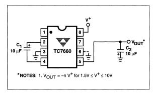
Figure 3. Simple Negative Converter
