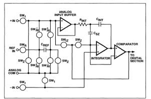
Figure 3A Analog Circuit Function Diagram
