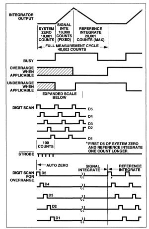
Figure 7 Timing Diagrams for Outputs
