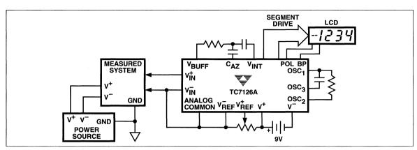
Figure 5 Common-Mode Voltage Removed in Battery Operation With VIN = Analog Common
