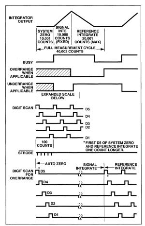
Figure 7. Timing Diagrams for Outputs
