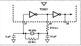
Figure 11. Suggested Crystal Oscillator Circuit
