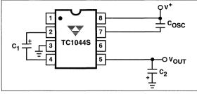
Figure 7. Lowering Oscillator Frequency
