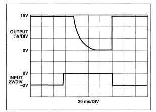
Figure 4 **Recovery From Positive Saturation**
