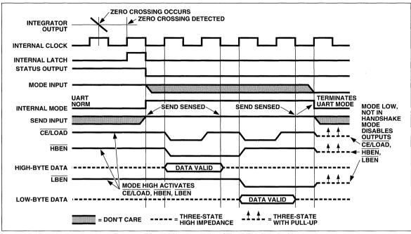
Figure 7 TC7109A Handshake With SEND INPUT Held Positive
