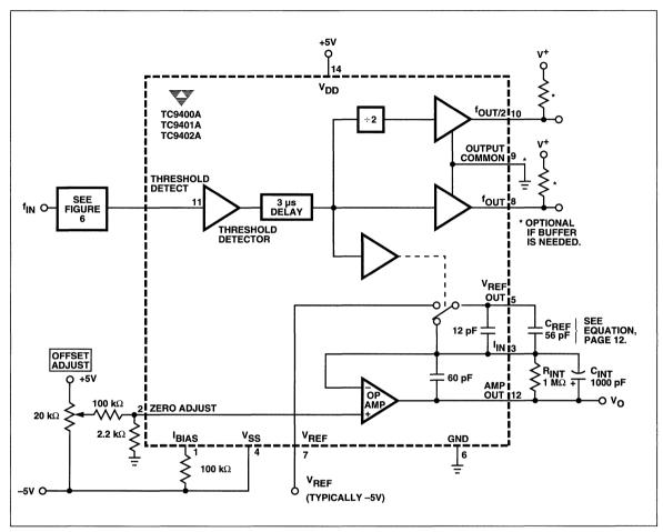
Figure 7 DC - 10 kHz F/V Converter
