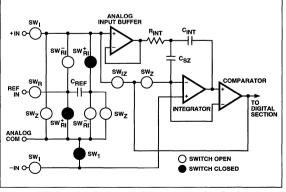
Figure 3D Reference Voltage Integration Cycle
