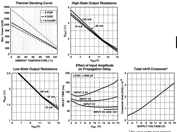
\* The values on this graph represent the loss seen by the driver during one complete cycle. For a single transition, divide the value by 2.
