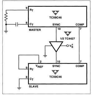
Figure 4 Master/Slave Parallel Operation
