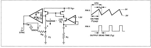
The oscillator frequency  $(F_O) = \frac{1}{T_{CHG} + T_D}$
