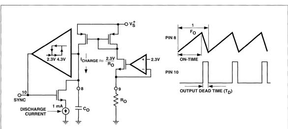
Figure 6 **Oscillator Circuit**
