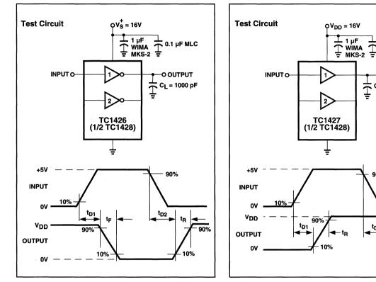
Figure 1. Inverting Driver Switching Time
