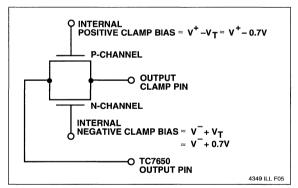
Figure 3 Internal Clamp Circuit
