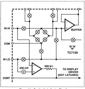
Figure 14 Continuity Indicator Circuit
