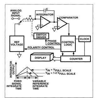
Figure 2. Basic Dual-Slope Converter
