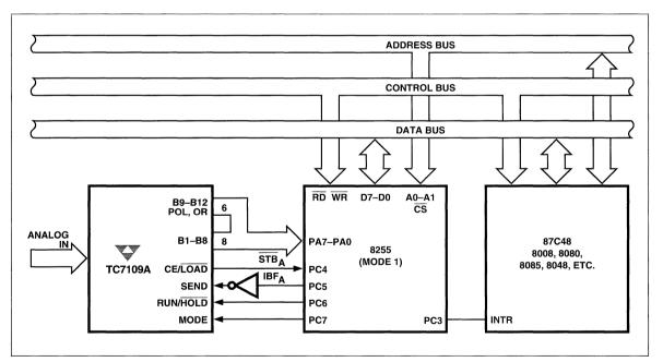
Figure 19 TC7109A Handshake Interface to MCS-48, -80, -85 Microcomputers
