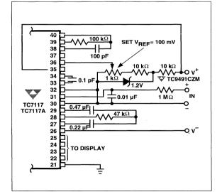
Figure 14 TC7117/TC7117A With a 1.2V External Band-Gap Reference ( $V_{IN}$  Tied to Common)
