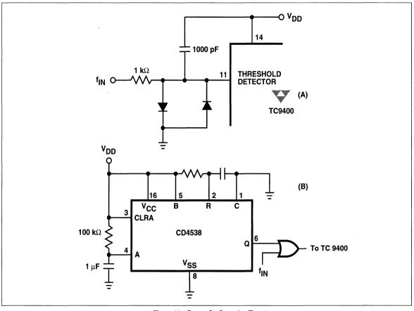
Figure 11 Power-On Operation/Reset
