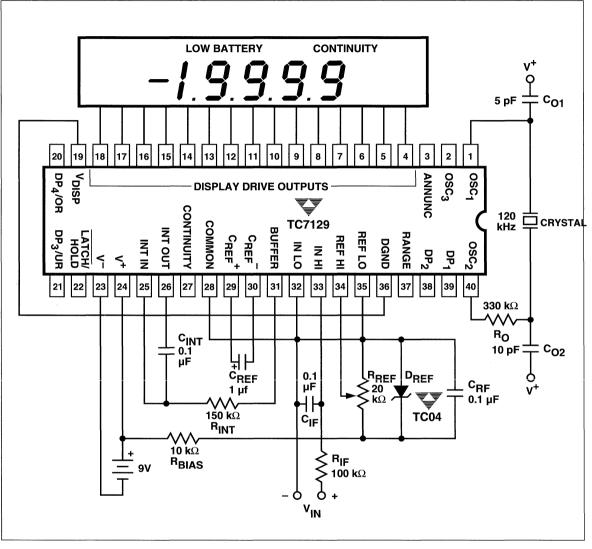
Figure 1 Standard Circuit
