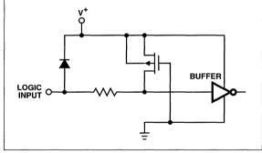
Figure 2 Digital Logic Input
