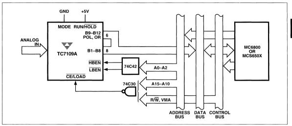
Figure 18 TC7109A Direct Interface to MC6800 Bus
