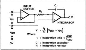
Figure 8 Common-Mode Voltage Reduces Available Integrator Swing  $(V_{COM} \neq V_{IN})$
