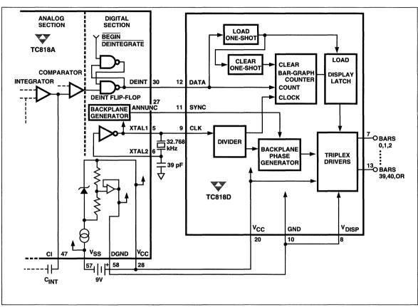
Figure 2 Interface Between TC818A and TC818D
