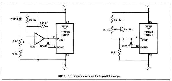
Figure 27. Temperature-Compensating Circuits
