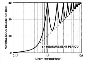
Figure 2 Normal-Mode Rejection of Dual-Slope Converter
