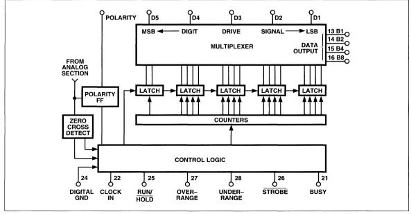
Figure 6. Digital Section Functional Diagram
