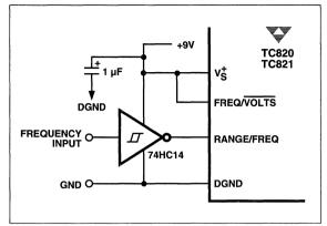
Figure 20. Frequency Counter External Buffer
