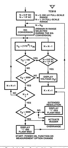
Figure 9 Auto-Range Operation; Voltage Measurement
