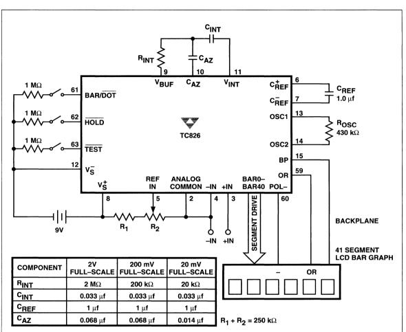
Figure 1 Typical TC826 Circuit Connection
