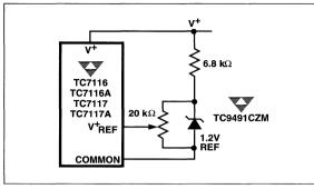
Figure 4 Using an External Reference
