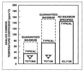
Figure 9 Analog Common Temperature Coefficient
