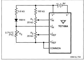
Figure 20 Positive Temperature Coefficient Resistor Temperature Sensor
