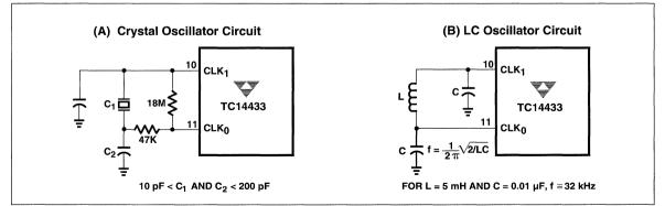
Figure 9. Alternate Oscillator Circuits
