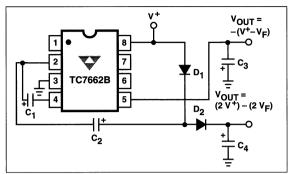
Figure 10. Combined Negative Converter and Positive Doubler
