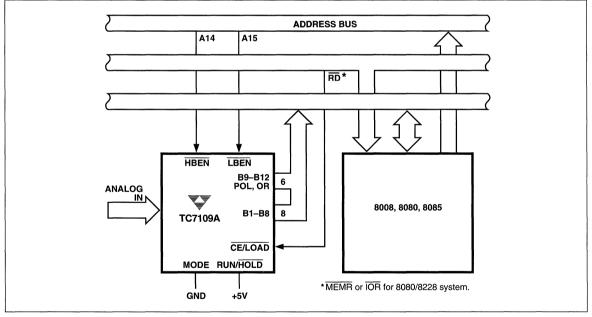
Figure 17 TC7109A Direct Interface to 8080/8085
