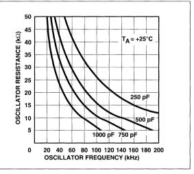
Figure 7 Oscillator Frequency vs Oscillator Resistance
