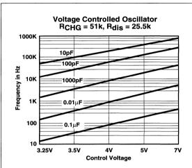
Figure 8 Frequency vs Control
