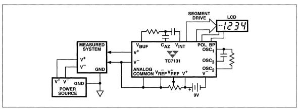
Figure 7 Common-Mode Voltage Removed in Battery Operation With V<sub>IN</sub> = Analog Common
