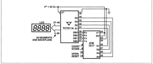
Figure 3. LCD Display Interface to 4-Digit Counter
