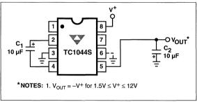
Figure 3. Simple Negative Converter
