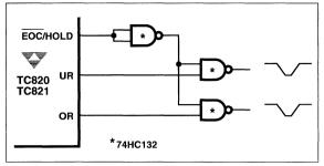
Figure 11. Generating Underrange and Overrange Pulses
