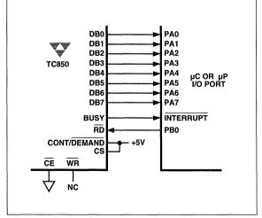
Figure 8 Interface to Typical µP I/O Port or Single-Chip µC
