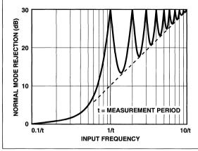
Figure 2 Normal-Mode Rejection of Dual-Slope Converter
