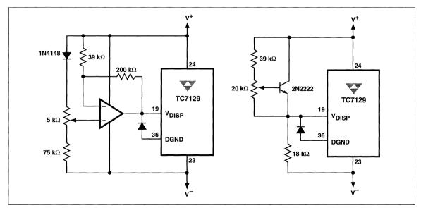
Figure 7 Temperature Compensating Circuits
