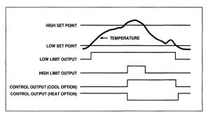
TC620/621 Input vs. Output Logic
