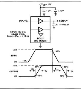
Test Figure 2. Noninverting Driver Switching Time Test Circuit
