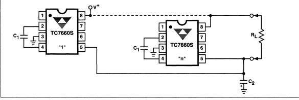
Figure 4. Paralleling Devices Lowers Output Impedance
