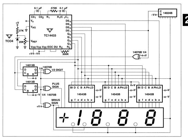
Figure 11. 3-1/2 Digit Voltmeter with LCD Display
