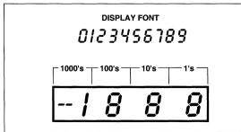
Figure 4 Display Font and Segment Assignment
