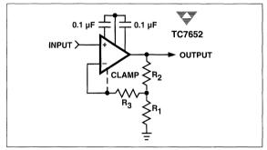
Figure 1 Noninverting Amplifier With Optional Clamp
