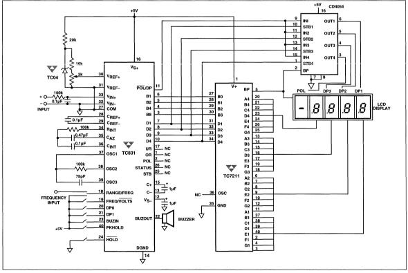
Figure 18. TC831 Interface to LCD Display
