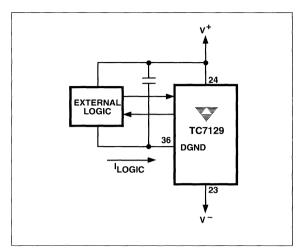
Figure 5 External Logic Referenced Directly to DGND
