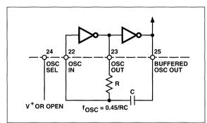
Figure 10 TC7109A RC Oscillator
