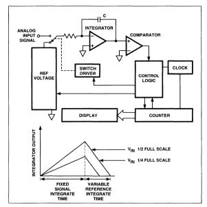
Figure 2 Basic Dual-Slope Converter
