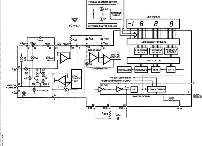
Figure 5 **TC7107A Block Diagram**
