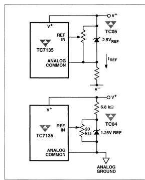
Figure 5. Using an External Reference Voltage
