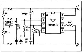
Figure 11. Splitting a Supply in Half
