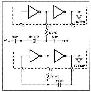
Figure 8 Oscillator Circuits
