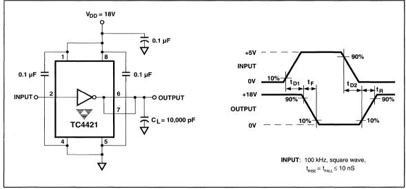
Figure 1. Switching Time Test Circuit
