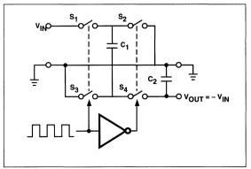
Figure 2. Idealized Negative Voltage Capacitor
