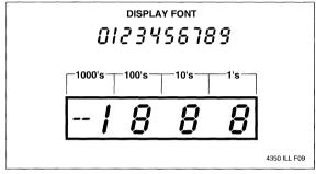
Figure 4 Display Font and Segment Assignment
