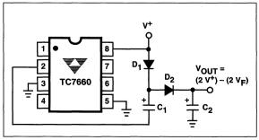
Figure 8. Positive Voltage Multiplier
