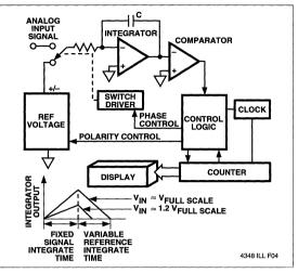
Figure 2 Basic Dual Slope Converter
