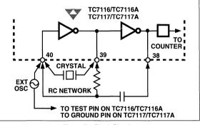
Figure 7 Clock Circuits
