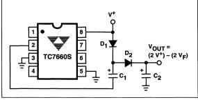
Figure 8. Positive Voltage Multiplier
