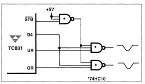
Figure 10. Generating Underrange and Overrange Pulses
