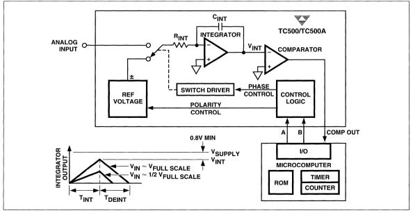
Figure 2. Basic Dual-Slope Converter
