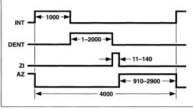
Figure 4 Conversion Timing During Normal Operation
