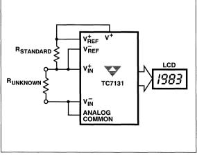
Figure 11 Low Parts Count Ratiometric Resistance Measurement
