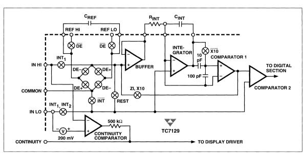
Figure 13 Integrator Block Diagram
