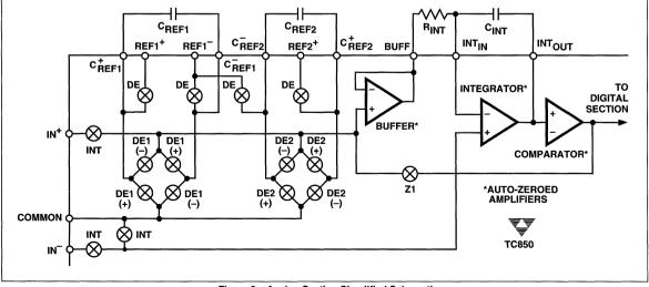
Figure 3 Analog Section Simplified Schematic
