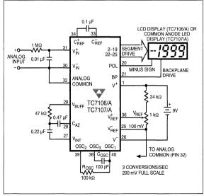
Figure 1 TC7106/A/7/A Typical Operating Circuit
