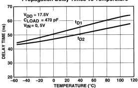
Propagation Delay Times vs Temperature
