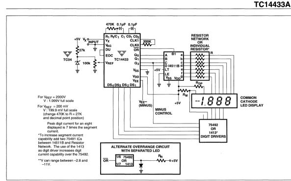
Figure 14. 3-1/2 Digit Voltmeter with Low Component Count Using Common Cathode Displays
