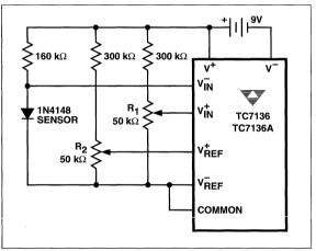
Figure 13 Temperature Sensor
