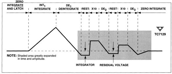
Figure 11 Integrator Waveform
