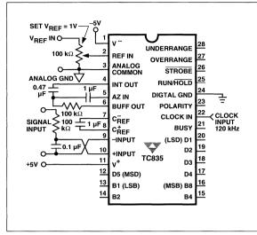
Figure 1 Test Circuit
