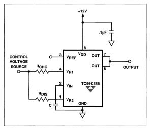
Figure 7 Voltage Controlled Power Oscillator
