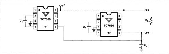
Figure 4. Paralleling Devices Lowers Output Impedance
