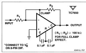
Figure 5 Inverting Amplifier With Optional Clamp
