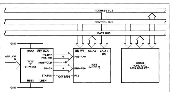
Figure 14 Full-Time Parallel Interface to MCS-48, -80, -85 Microcomputers
