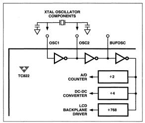
Figure 8 System Clock Generation
