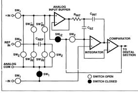
Figure 3E Integrator Output Zero Phase
