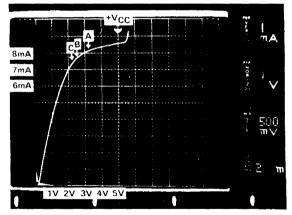
Figure 14 TC7107A Output Current vs Output Voltage
