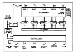
Figure 6 Digital Section Functional Diagram
