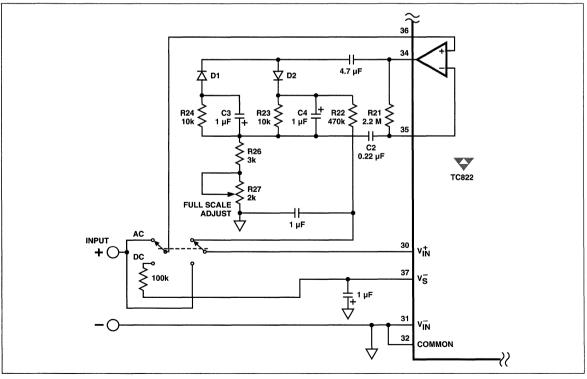
Figure 11 Low Cost AC-to-DC Converter
