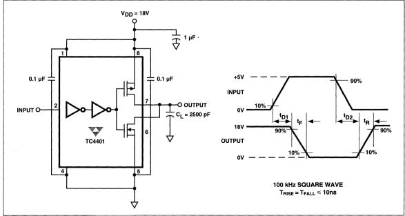
Figure 1. Switching Time Test Circuit
