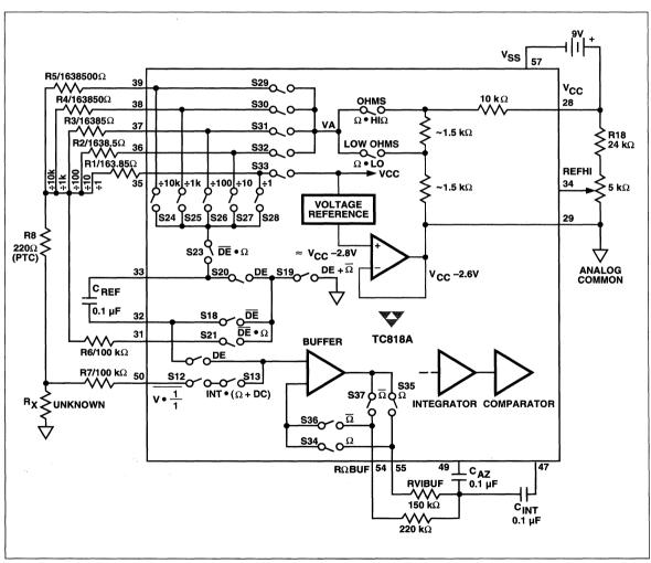
Figure 3 Ratiometric Resistance Measurement Functional Diagram
