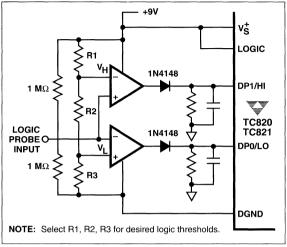
Figure 22. Window Comparator Logic Probe
