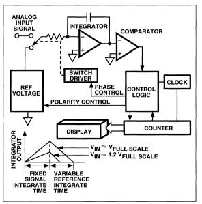
Figure 1 Basic Dual-Slope Converter
