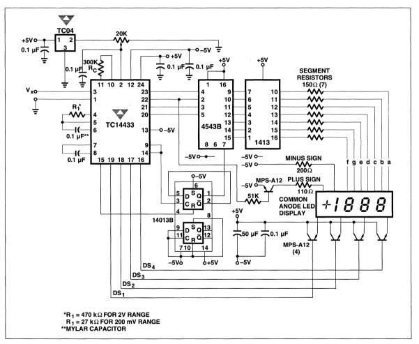
Figure 10. 3-1/2 Digit Voltmeter Common-Anode Displays, Flashing Overrange
