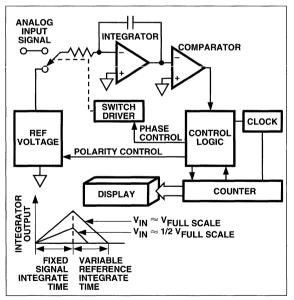
Figure 4 Basic Dual-Slope Converter
