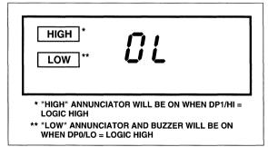
Figure 7. LCD During Logic Probe Operation
