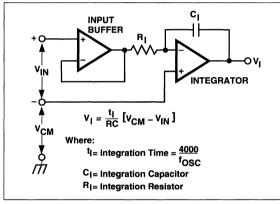
Figure 9. Common-Mode Voltage Reduces Available Integrator Swing (V<sub>COM</sub>  $\neq$  V<sub>IN</sub>)
