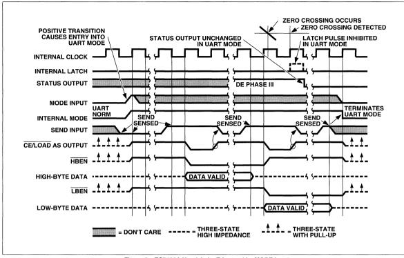
Figure 9 TC7109A Handshake Triggered by MODE Input
