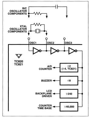
Figure 17. System Clock Generation
