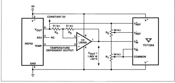
Figure 14 Integrated Circuit Temperature Sensor
