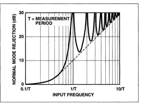
Figure 3. Normal-Mode Rejection of Dual-Slope Converter
