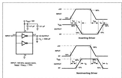
Figure 1. Switching Time Test Circuit
