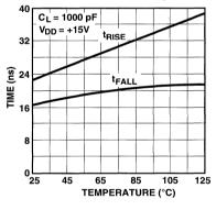
Delay Time vs Temperature
