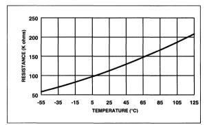
TC620 Sense Resistors vs. Trip Temperature
