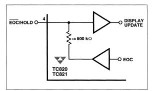
Figure 10. EOC/HOLD Pin Schematic
