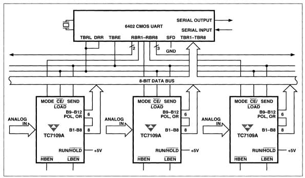
Figure 21 Handshake Interface for Multiplexed Converters
