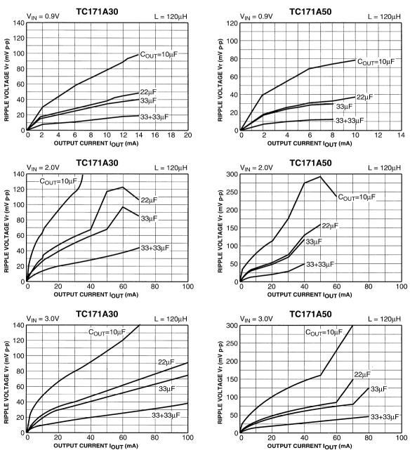
11) Ripple Voltage vs. Output Current ( $T_A = 25^{\circ}C$ )
