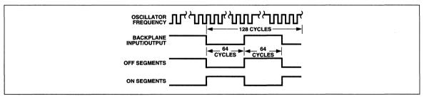
Figure 2: LCD Display Waveforms
