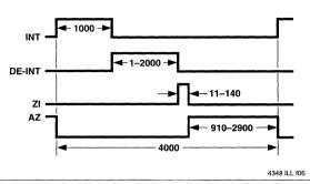
Figure 4a Conversion Timing During Normal Operation
