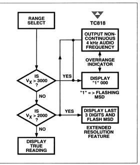
Figure 8 Manual Range Selection; Voltage Measurement
