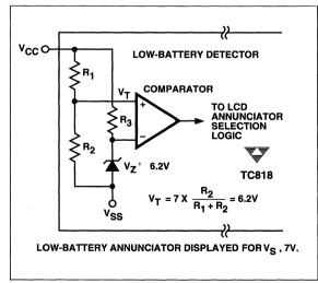
Figure 11 Low-Battery Detector
