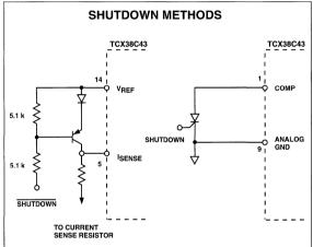
Shutdown can be accomplished by either pulling  $I_{SENSE}$  above 1 volt or pulling COMP, pin 1 to GND. This will set the PWM latch so that the output will remain low until the next clock pulse after the shutdown condition is removed.
