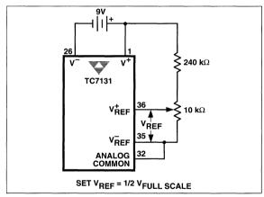
Figure 9 TC7136A Internal Voltage Reference Connection
