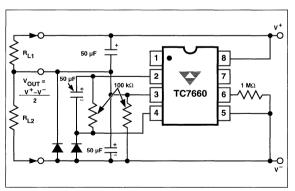
Figure 11. Splitting a Supply in Half
