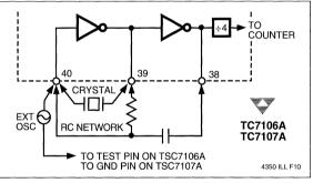
Figure 6 Clock Circuits
