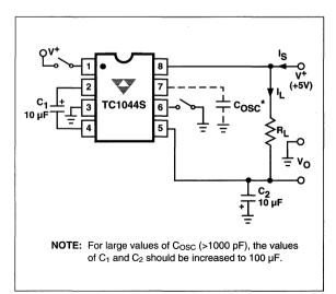
Figure 1. TC1044S Test Circuit
