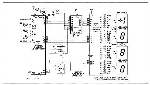
Figure 15. TC7212A Interface to TC14433 3-1/2 Digit ADC
