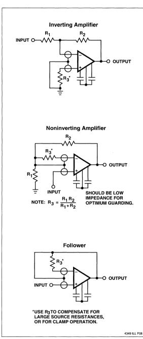
Figure 6 Input Guard Connection
