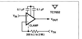
Figure 4 Low Offset Comparator
