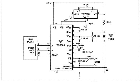
The comparator output stays low during the Integration phase (A=1, B=0) whenever the input polarity is negative. In those cases where the input polarity is negative AND very near zero, the zero-crossing occurs before the comparator has had a chance to go positive. Thus, no negative edge will be generated and the microprocessor will not be interrupted.
