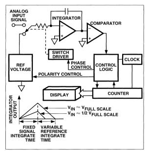
Figure 4. Basic Dual-Slope Converter
