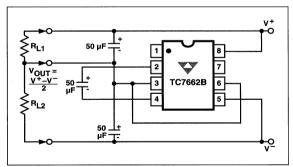
Figure 11. Splitting a Supply in Half
