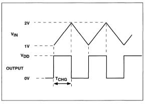
Figure 3 VIN and Output Waveform
