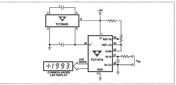
Figure 12b. Negative Power Supply Generation for TC7107A ADC
