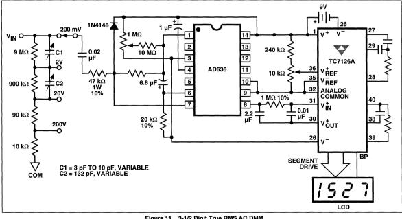
Figure 11 3-1/2 Digit True RMS AC DMM
