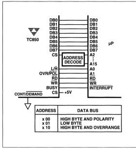
Figure 7 Interface to Typical  $\mu$ P Data Bus
