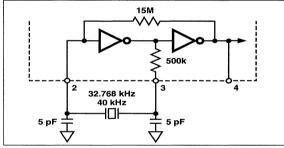
Figure 7 Crystal Oscillator Circuit
