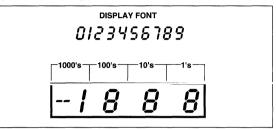
Figure 6 Display FONT and Segment Assignment
