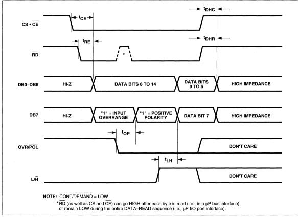
Figure 10 Bus Output Timing, Demand Mode
