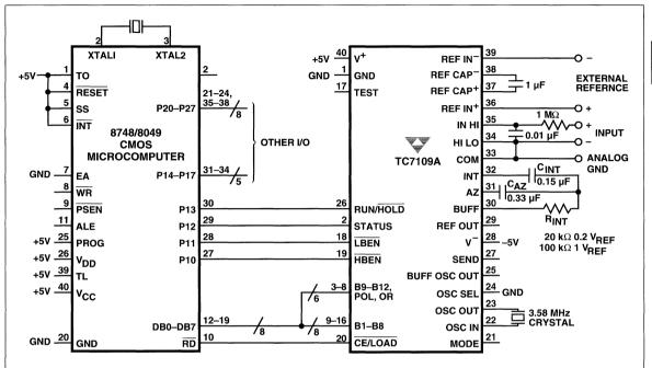
Figure 2 TC7109A Parallel Interface With 8048/8049 Microcomputer
