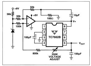
Figure 12. Regulating the Output Voltage
