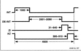
Figure 4b Conversion Timing During Overrange Operation
