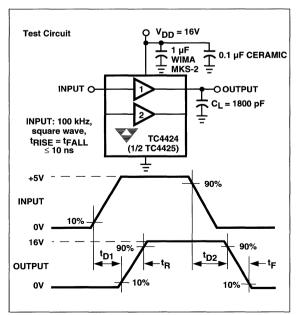
Figure 2 Noninverting Driver Switching Time
