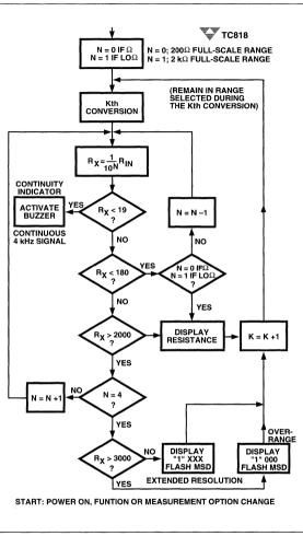
Figure 10 Auto-Range Operation; Resistance Measurement
