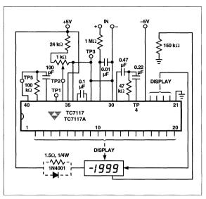
Figure 18 Diode or Resistor Limits Package Power Dissipation
