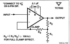
Figure 4 Noninverting Amplifier With Optional Clamp
