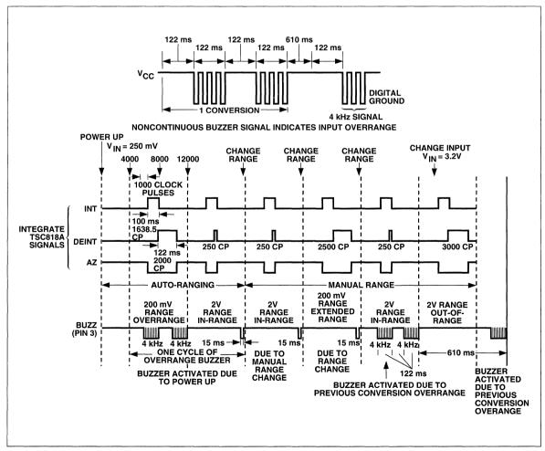
Figure 15 TC818 Timing Waveform for Buzzer Output
