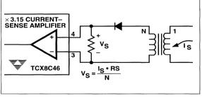
Figure 3 Transformer Isolated Current Sense
