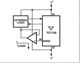
Figure 6 External Logic Referenced to DGND With Buffer
