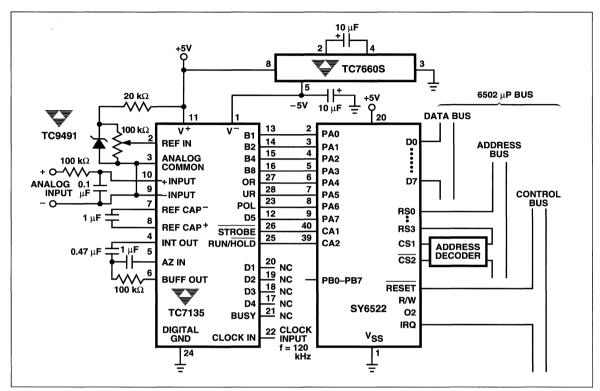
Figure 13. TC7660S Supplies -5V for Converters in Microprocessor-Controlled Data Acquisition Systems
