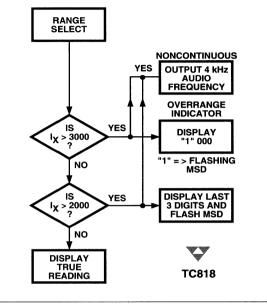
Figure 7 Manual Range Selection; Current Measurement
