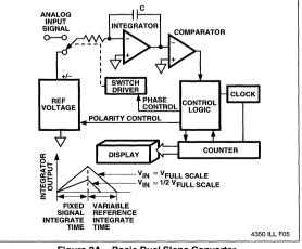
Figure 2A Basic Dual Slope Converter
