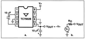
Figure 3. Simple Negative Converter and its Output Equivalent
