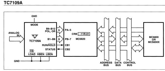
Figure 16 Full-Time Parallel Interface to MC6800 or MCS650X Microprocessor
