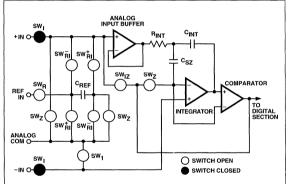
Figure 3C. Input Signal Integration Phase
