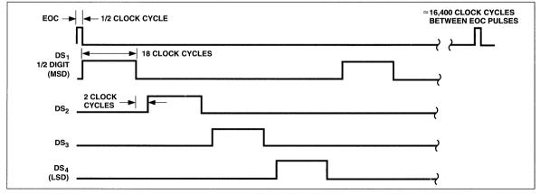
Figure 12. Digit Select Timing Diagram
