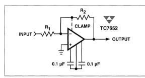
Figure 2 Inverting Amplifier With Optional Clamp
