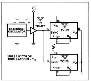
Figure 5 External Clock Synchronization
