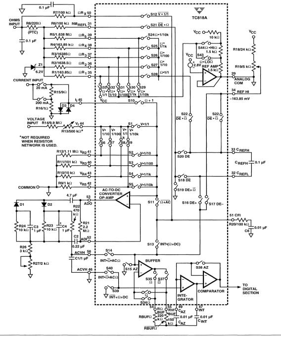
Figure 1 TC818A Analog Section
