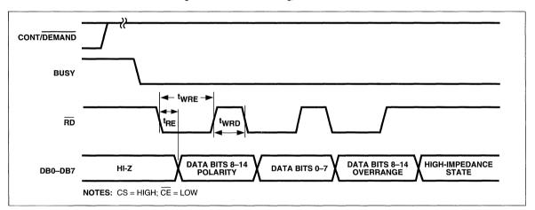
Figure 12 Bus Output Timing, Continuous Mode
