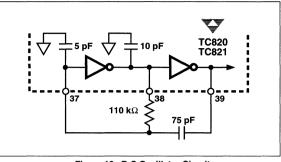
Figure 16. R-C Oscillator Circuit
