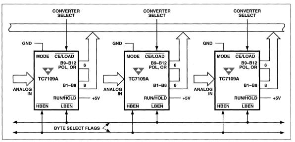
Figure 13 Three-Stating Several TC7109A's to a Small Bus
