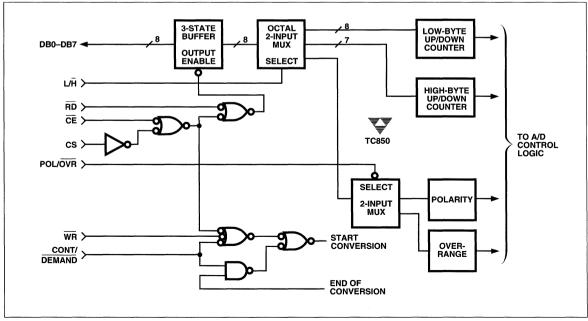
Figure 5 Bus Interface Simplified Schematic
