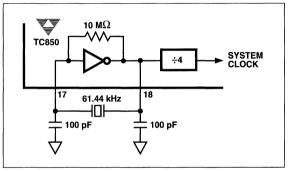
Figure 6 Crystal Oscillator Schematic
