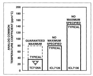
Figure 7 Analog Common Temperature Coefficient
