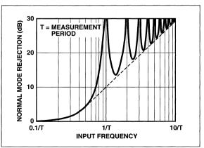
Figure 3. Normal-Mode Rejection of Dual-Slope Converter
