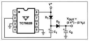
Figure 9. Positive Voltage Multiplier
