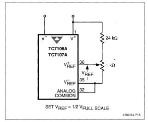
Figure 11 Internal Voltage Reference Connection
