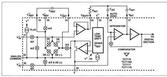
Figure 3 Analog Section of TC7116/TC7116A and TC7117/TC7117A
