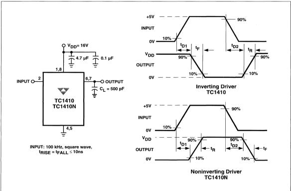
Figure 1. Switching Time Test Circuit
