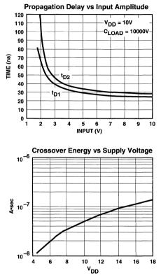
**NOTE:** The values on this graph represent the loss seen by the driver during a complete cycle. For the loss in a single transition, divide the stated value by 2.
