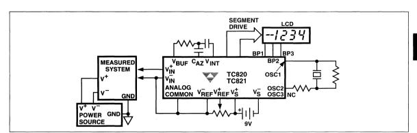
Figure 8. Common-Mode Voltage Removed in Battery Operation With VIN<sup>-</sup> = Analog Common
