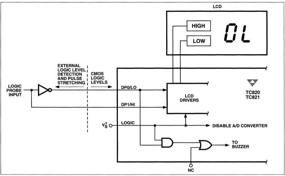
Figure 6. Logic Probe Simplified Schematic
