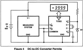
gure 4 DC-to-DC Converter Permits Ground Referenced Measurements
