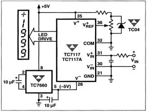
Figure 10 Negative Power Supply Generation With TC7660
