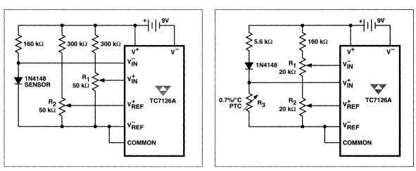
Figure 12 Temperature Sensor
