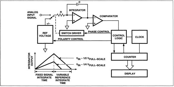
Figure 2 Basic Dual Slope Converter
