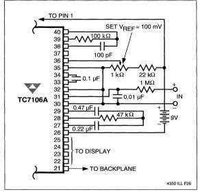
Figure 22 TC7106A Using the Internal Reference: 200 mV Full-Scale, 3 Readings-per-second (RPS).
