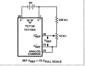
Figure 10 TC7136A Internal Voltage Reference Connection
