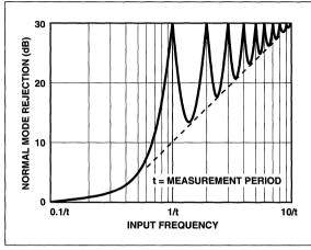
Figure 2 Normal-Mode Rejection of Dual-Slope Converter
