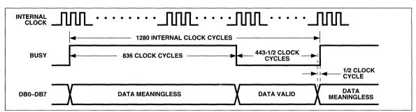
Figure 11 Conversion Timing, Continuous Mode
