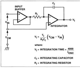
Figure 5 Common-Mode Voltage Reduces Available Integrator Swing. ( $V_{COM} \neq V_{IN}$ )
