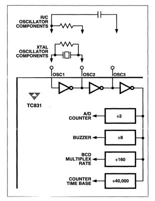
Figure 13. System Clock Generation
