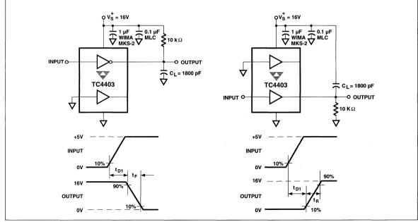
Figure 1 Switching Time Test Circuits
