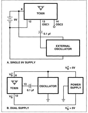
Figure 9 External Oscillator Connection
