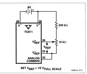
Figure 10 TC811 Internal Voltage Reference Connection
