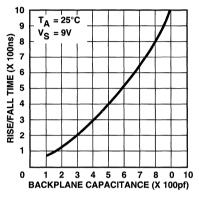
Figure 11 Backplane Driver Rise/Fall Time vs. Capacitance
