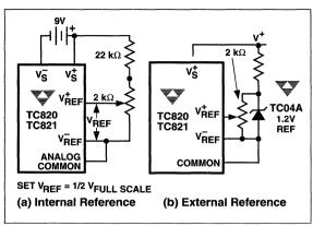
Figure 18. Reference Voltage Connections
