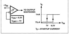
The typical turn on threshold is 9.2 V for operation of this family of PWM Controllers. When supply voltage at pin 15 drops below 7 V, after normal operation above 9.2 V, lockout occurs and both output drives to pin 11 and 14 are terminated.
