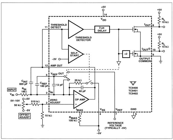
Figure 1 10 Hz to 10 kHz V/F Converter
