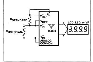
Figure 15. Low Parts Count Ratiometric Resistance Measurement
