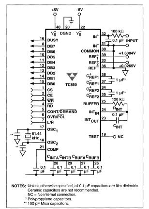
Figure 1 Standard Circuit Configuration
