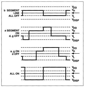
Figure 19 Typical Display Output Waveforms
