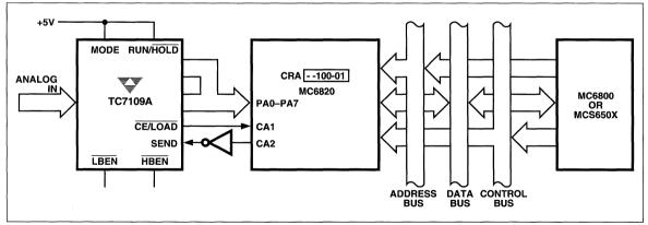
Figure 20 TC7109A Handshake Interface to MCS-6800, MCS650X Microprocessors
