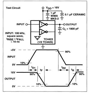
Figure 1 Inverting Driver Switching Time
