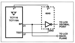
Figure 5 Simple Inverter for Fixed Decimal Point
