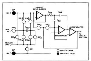
Figure 3C Input Signal Integration Phase
