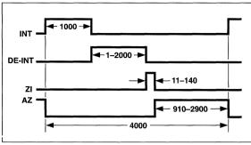
Figure 4 Conversion Timing During Normal Operation
