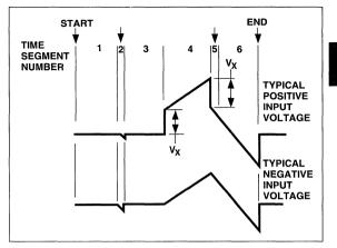
Figure 7. Integrator Waveforms at Pin 6
