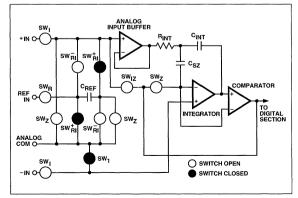
Figure 3D. Reference Voltage Integration Phase
