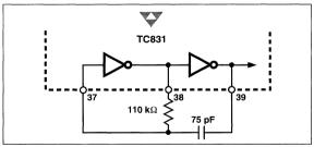
Figure 12. R-C Oscillator Circuit
