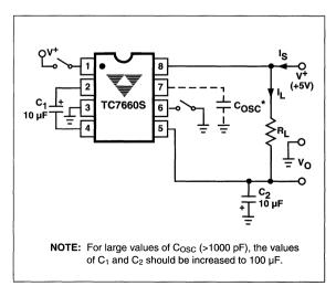
Figure 1. TC7660S Test Circuit
