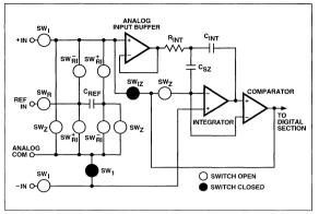
Figure 3E. Integrator Output Zero Phase
