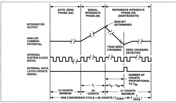
Figure 5 TC826 Conversion Has Three Phases
