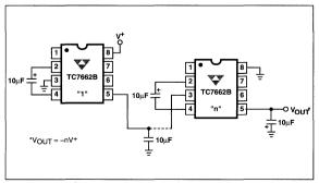
Figure 6. Cascading Devices for Increased Output Voltage
