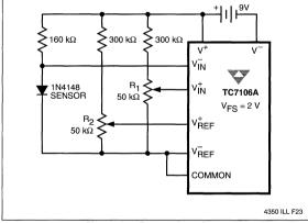
Figure 19 Temperature Sensor
