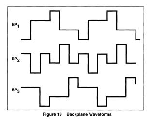
The ANNUNCIATOR DRIVE output (pin 3) is a squarewave running at the backplane frequency (100 Hz or 83.3 Hz), with a peak-to-peak voltage equal to DGND voltage. Connecting an annunciator to pin 3 turns it ON; connecting it to its backplane turns it OFF.
