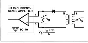
Figure 3 Transformer Isolated Current Sense
