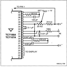
Figure 25 TC7106A/TC7107A: Recommended Component Values for 2.00 V Full-Scale
