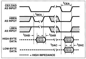
Figure 6 TC7109A Direct Mode Output Timing
