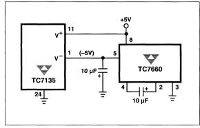
Figure 9. Negative Supply Voltage Generator
