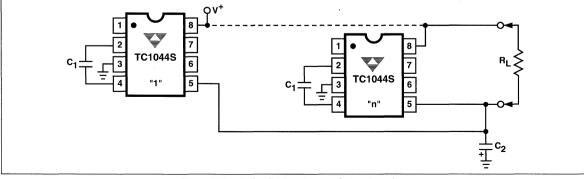
Figure 4. Paralleling Devices Lowers Output Impedance
