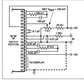
Figure 12 TC7117/TC7117A Internal Reference (200 mV Full Scale, 3 RPS, V<sub>IN</sub> Tied to GND for Single-Ended Inputs.)
