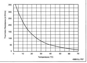
**Typical Thermistor Resistance vs Temperature**
