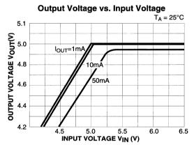
Output Voltage vs. Input Voltage  $T_A = 25^{\circ}C$
