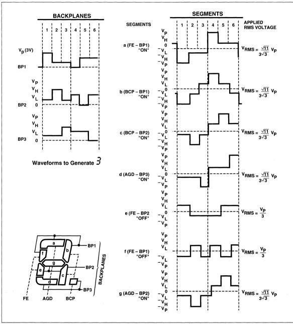
Figure 13 Triplex LCD Drive Waveforms
