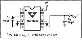
Figure 3. Simple Negative Converter
