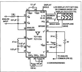
Figure 1 Typical TC7116/A/7/A Operating Circuit
