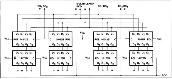
Figure 13. Demultiplexing for TC14433 BCD Data
