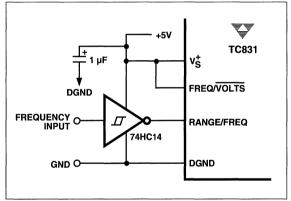
Figure 16. Frequency Counter External Buffer
