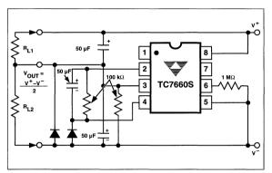
Figure 11. Splitting a Supply in Half
