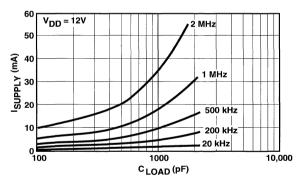
Supply Current vs Capacitive Load
