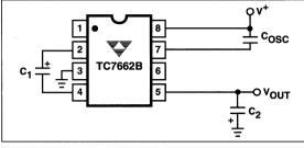
Figure 8. Lowering Oscillator Frequency
