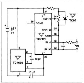
Figure 3 Powering the TC7129 From a Low-Voltage Battery
