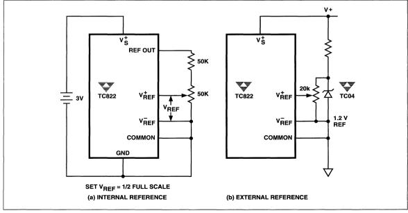
Figure 9 Internal and External Reference Applications
