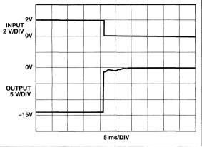
Figure 3 Recovery From Negative Saturation
