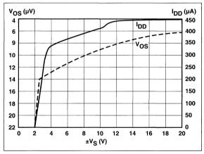
Figure 2 V<sub>OS</sub> and I<sub>DD</sub> vs Supply Voltage
