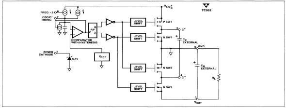
Pin 1, which is used as a test pin on the 7662, is a voltage reference zener on the TC962. This zener (6.4V at 5 mA) has a dynamic impedance of  $12\Omega$  and is intended for use where the TC962 is supplying current to external regulator circuitry and a reference is needed for the regulator circuit. (See applications section.)
