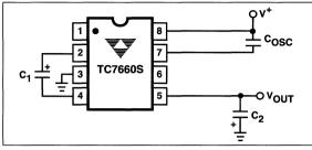
Figure 7. Lowering Oscillator Frequency
