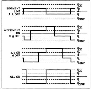
Figure 25. Typical Display Output Waveforms
