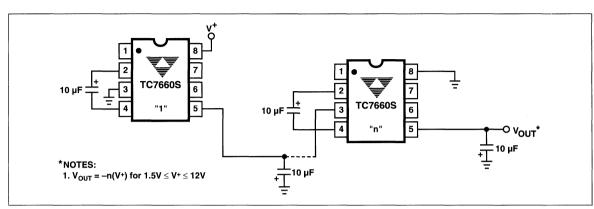
Figure 5. Increased Output Voltage by Cascading Devices
