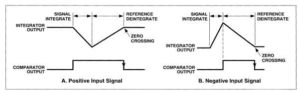
Figure 1. Comparator Output
