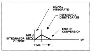
Figure 2A Dual-Slope ADC Cycle
