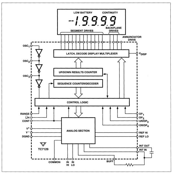
Figure 12 Functional Diagram
