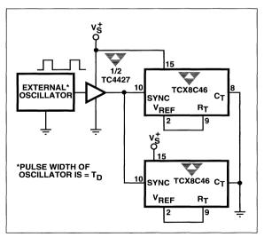
Figure 5 External Clock Synchronization
