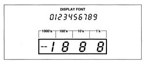
Figure 6 Display FONT and Segment Assignment
