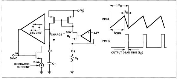
Figure 6 Oscillator Circuit
