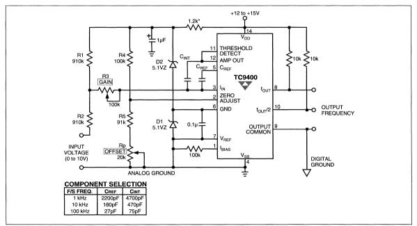
Figure 5 Voltage to Frequency
