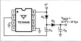
Figure 8. Positive Voltage Multiplier
