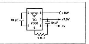
Figure 6 Splitting +15V With the 7660 at >95% Efficiency
