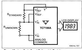
Figure 17 Low Parts Count Ratiometric Resistance Measurement
