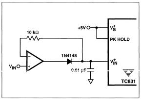
Figure 17. External Peak Detector
