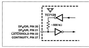
Figure 15 Input/Output Pin Schematic
