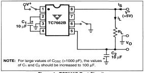
Figure 1. TC7662B Test Circuit
