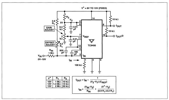
Figure 4 Fixed Voltage — Single Supply Operation
