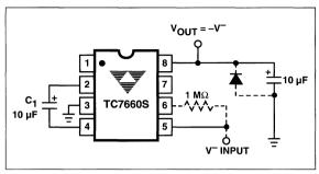
Figure 10. Positive Voltage Multiplier
