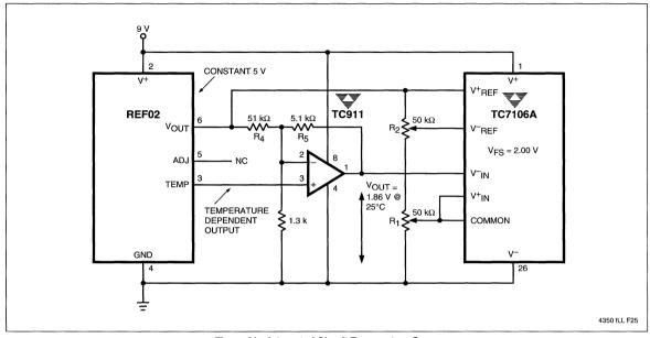
Figure 21 Integrated Circuit Temperature Sensor
