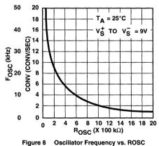
FOSC is divided by 32 to provide an internal system clock, FYSY. Each conversion requires 80 internal clock cycles. The internal system clock is divided by 8 to provide the LCD backplane drive frequency. The display flash rate during an input out-of-range signal is set by dividing FSYS by 320.
