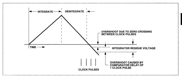
Figure 10 Accuracy Errors in Dual-Slope Conversion
