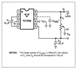
Figure 1. TC7660 Test Circuit
