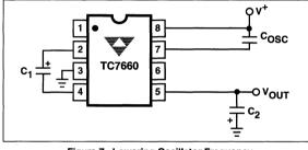
Figure 7. Lowering Oscillator Frequency
