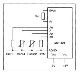
Figure 9.8: Referencing with Precision Resistors
