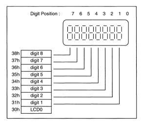
Figure 8.2: Allocation of the LCD Digits in the Memory
