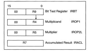
Figure 4.2: 8 x 8 Bit Multiplication : Register Use
