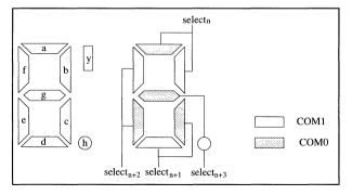
Figure 8.4: Allocation of the Segments, 2 MUX Mode
