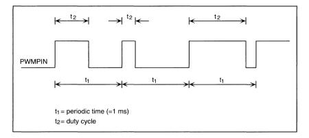
Figure 7.3: PWM Modulation
