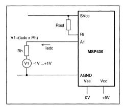
Figure 9.5: Current Source for Level Shifting
