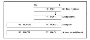
Figure 4.1: 16 x 16 Bit Multiplication : Register Use
