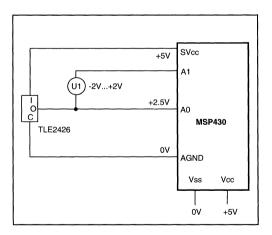
Figure 9.3: Virtual Ground IC for Level Shifting
