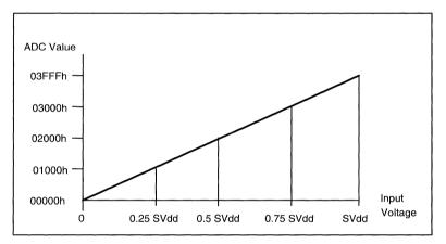
Figure 9.2: Complete ADC Range
