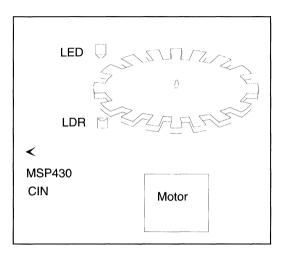
Figure 7.5: Measuring the Revolutions of a Toothed-Wheel
