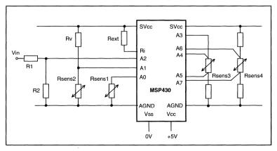
Figure 9.11: Possible Sensor Connections to the MSP430
