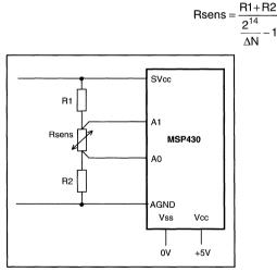
Figure 9.6: 4-Wire Circuitry with Voltage Supply
