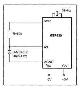
Figure 3.0: Battery Check
