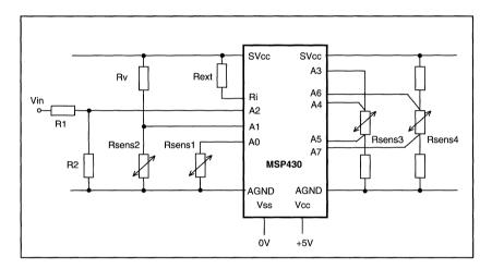
Figure 9.1: Possible Sensor Connections to the MSP430
