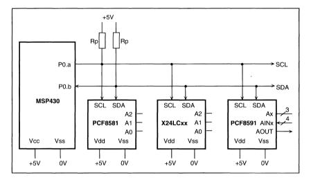
Figure 6.5: I2C-Bus Connections
