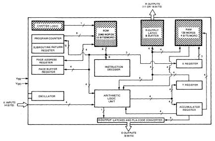
FIGURE 7 - TMS 1100/1300 LOGIC BLOCKS
