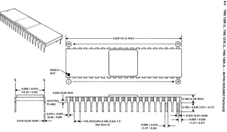
NOTES: a. Each pin centerline is located within 0.010 inch (0.26 millimeters) of its true longitudinal position. b. All linear dimensions are shown in inches (and parenthetically in millimeters for reference only). Inch dimensions govern.
