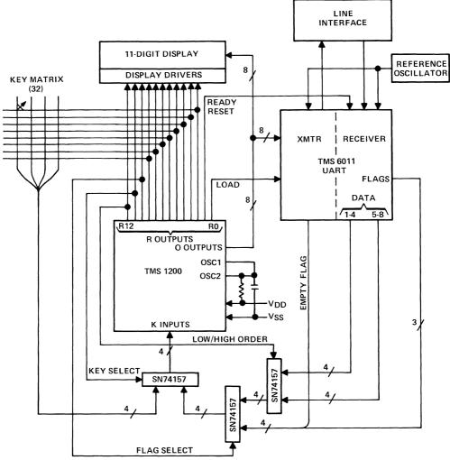
NOTE: Discrete components for level shifting and other functions are not shown.
