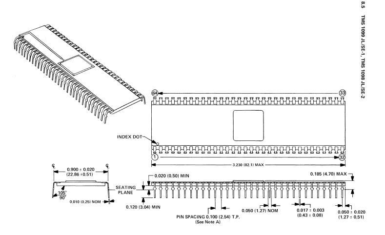
NOTES: a. Each pin centerline is located within 0.010 inch (0.26 millimeters) of its true longitudinal position. b. All linear dimensions are shown in inches (and parenthetically in millimeters for reference only). Inch dimensions govern.
