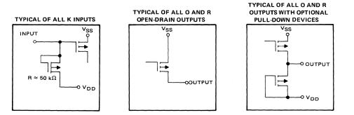
The O outputs have nominally 60  $\Omega$  on-state impedance; however, upon request a 130- $\Omega$  buffer can be mask programmed (see note  $[\ddagger]$  section 4.3).
