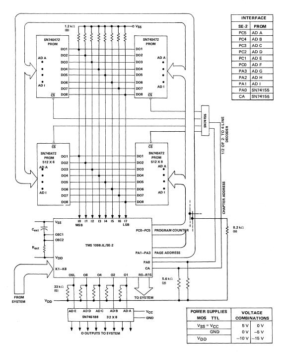
FIGURE 11 - BLOCK DIAGRAM OF TYPICAL APPLICATION - PROTOTYPING SYSTEM WITH SE-2
