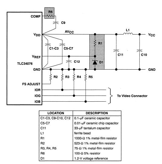
Figure B–1. Typical Connection Diagram and Components (Shaded Area is Optional)
