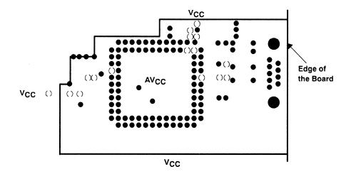
Figure B-3. Typical Split Power Plane (Solder Side)
