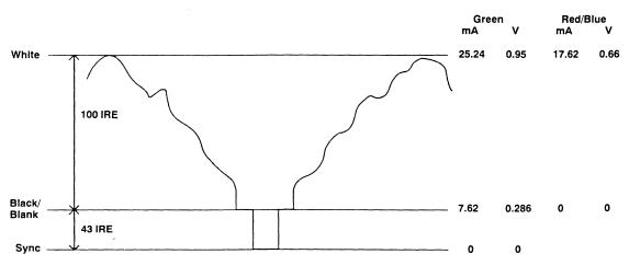
Figure 2-8. 0-IRE, 8-Bit Composite Video Output
