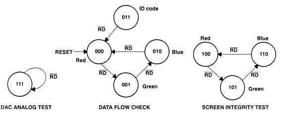
Figure 2–11. Test Register Control Word State Diagrams
