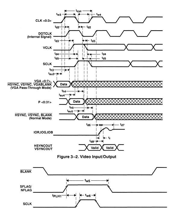
Figure 3–3. SFLAG/NFLAG Timing (When SSRT Function is Enabled)
