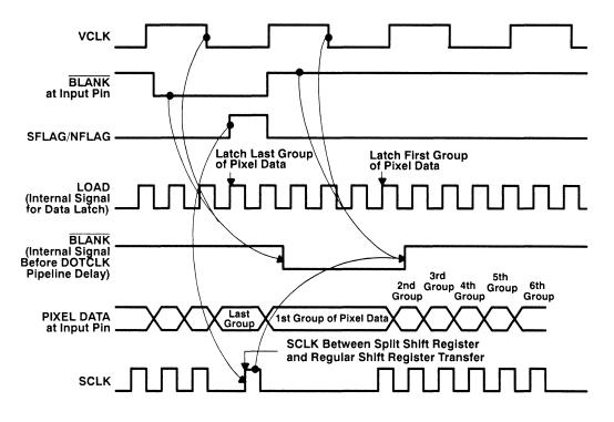
Figure 2–5. SCLK/VCLK Control Timing (SSRT Enabled, SCLK Frequency = 4 × VCLK Frequency)
