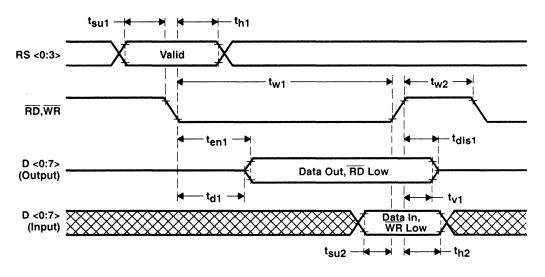
Figure 3–1. MPU Interface Timing
