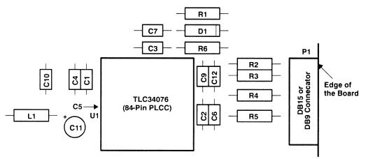
Figure B-2. Typical Component Placement (Component Side)
