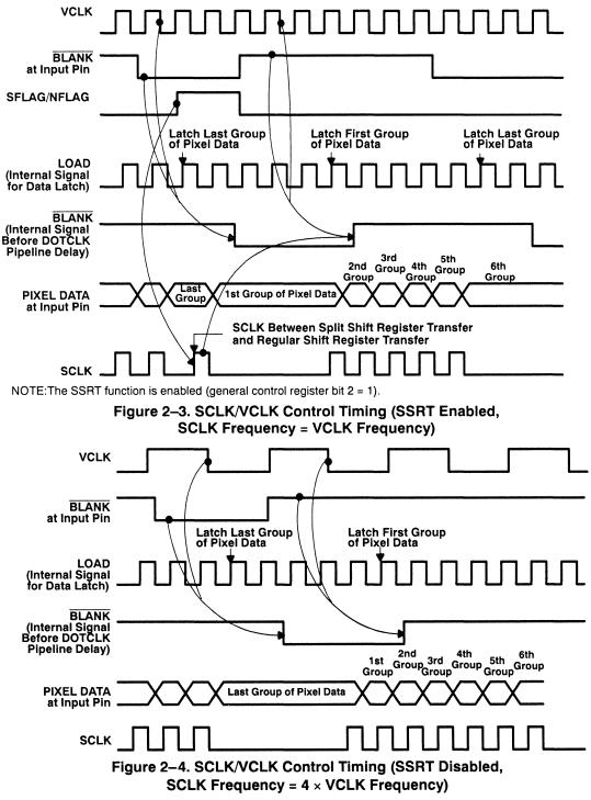
NOTE: Either the SSRT function is disabled (general control register bit 2 = 0), or the SFLAG/NFLAG input is held low if the SSRT function is enabled (general control register bit 2 = 1).
