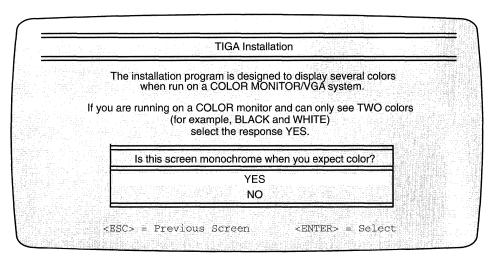
Some VGA boards require that the monitor be connected to the VGA board at boot-up. If the monitor is not connected, the system may boot the VGA in the monochrome mode. This problem may occur in single monitor systems. Step 11 and Step 12 help you to determine whether this condition exists and provide a suggested remedy.
