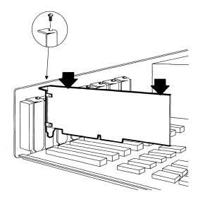
Do not force the SDB20 into the slot. Avoid touching any board component while installing the board.
