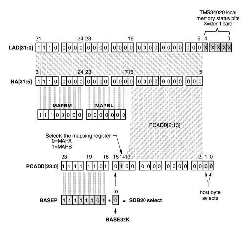
During a PC bus cycle, the SDB20 logic compares the upper eight bits of the PC address bus (PCADD[16:31]) to the contents of the BASEP register.
