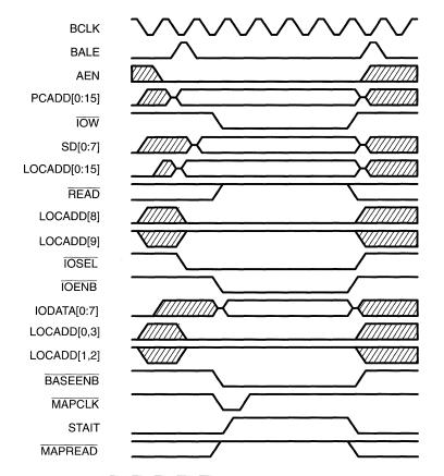
**Note:** The NOWS, REFRESH, and BUSRDY signals are not shown in this figure. However, they are all held high during the write cycle. For all I/O cycles, BUSRDY is held high to prevent wait-states from being inserted into the cycle.
