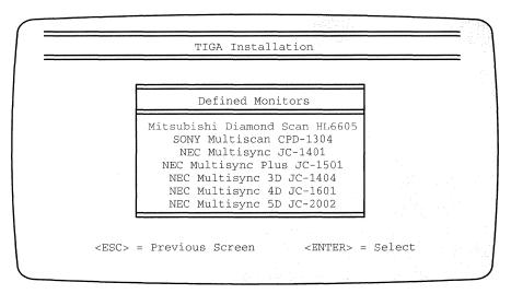
**Step 10:** Select the model number of the monitor that you are using. If the monitor you are using is not on this list, press it accept the default selection.
