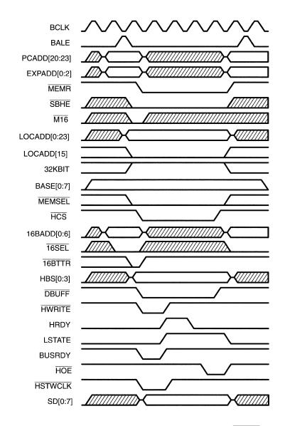
**Note:** Although they are not shown in this figure, the NOWS, SDBENB, READ, 16BITEN, and 16XF signals are held high; the BASE32K signal is held low.
