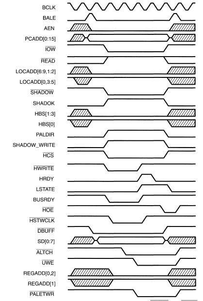
**Note:** Although they are not shown in this figure, the NOWS and READ signals are held high; the SHADENB and VGAENB signals are held low.
