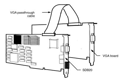
The SDB20 supports VGA passthrough for greater than or equivalent bus addressing. This means that the SDB20 must be installed in a 16-bit slot when the VGA adapter resides in a 16-bit slot, and in an 8-bit or 16-bit slot when used with an 8-bit VGA adapter.
