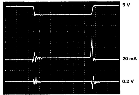
b) SN74S00 load: C_L = 50 \text{ pF}
