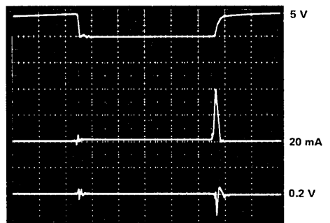
j) SN74ALS00A load: C_L = 50 \text{ pF}
