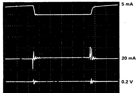
d) SN74LS00 load: C_L = 50 \text{ pF}
