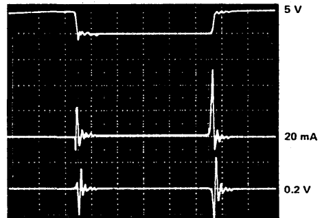
f) SN74AS00 load: C_L = 50 \text{ pF}
