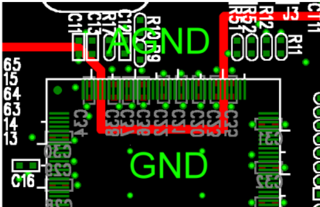
Figure 8. Reference Ground Partitions under the VT6202
