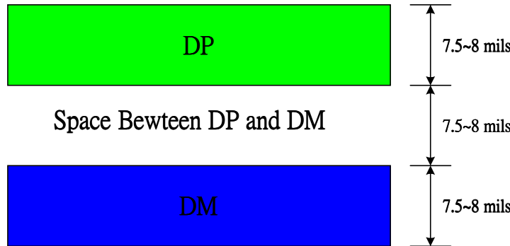
Figure 11. USB Differential Signal Routing
