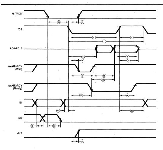
Figure 70. Non-Multiplexed /DS Interrupt Acknowledge Cycle
