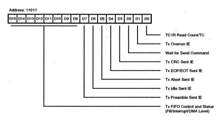
Figure 46a. Transmit Interrupt Control Register
