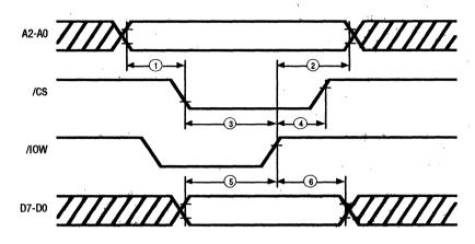
Figure 44. CPU Write Cycle
