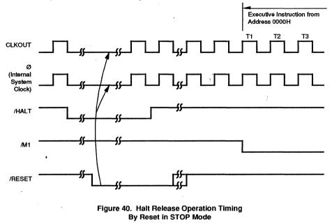
**Start-up Time at Time of Restart (STOP Mode).** When the MPU is released from the halt state by accepting an interrupt request, it executes an interrupt service routine Therefore, when an interrupt request is accepted, it starts generating clock on the CLKOUT pin, after a start-up time, by the internal counter [(2<sup>14</sup>+2 5) TcC (TcC Clock Cycle)]. This obtains a stabilized oscillation for operation.
