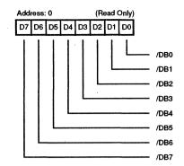
Figure 4. Current SCSI Data Register
