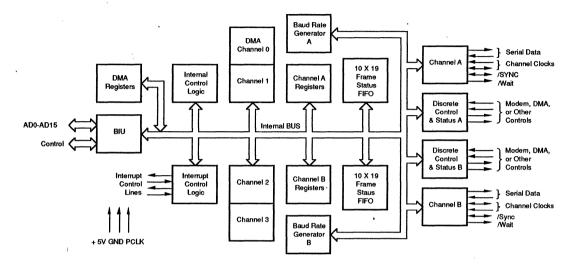
Figure 3. Block Diagram of ISCC Architecture
