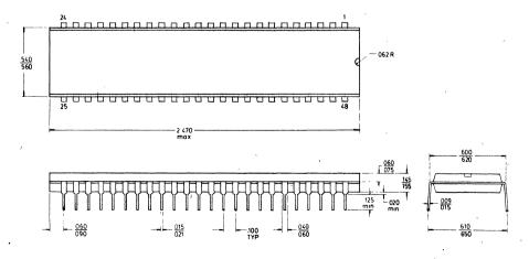
48-Pin Plastic Dual-In Line Package (PDIP)
