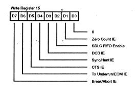
Figure 9. Write Register Bit Functions (Continued)
