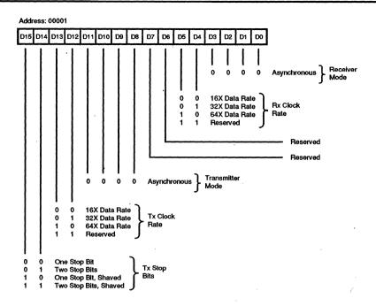
Figure 9. Channel Mode Register, Asynchronous Mode
