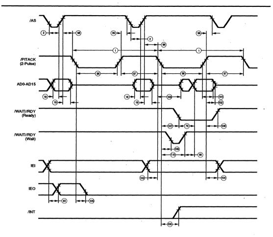
Figure 73. Multiplexed Double-Pulse Intack Cycle
