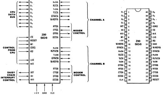
Figure 5. Pin Functions
