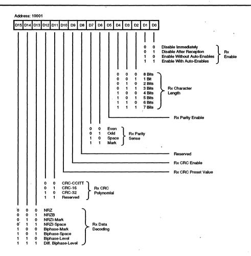
Figure 36. Receive Mode Register
