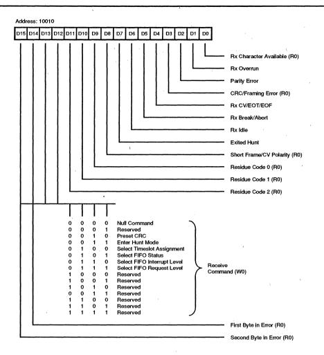
Figure 37. Receive Command Status Register
