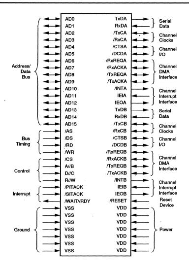
Figure 2. Pin Functions
