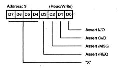
Figure 9. Target Command Register
