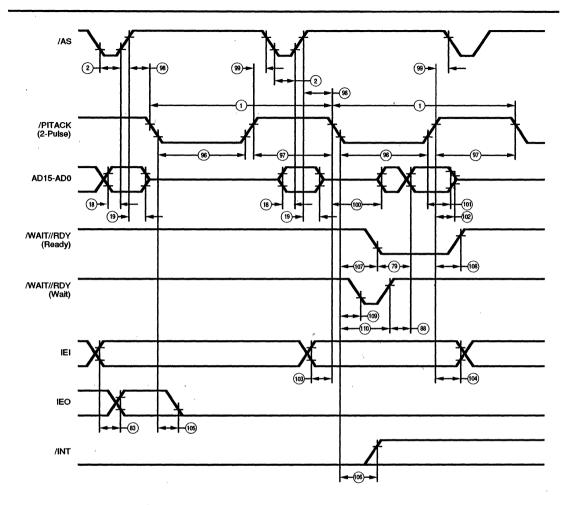
Figure 73. Multiplexed Double-Pulse Intack Cycle
