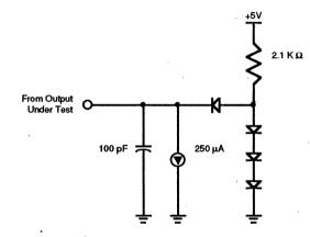
Figure 25. Standard Test Load
