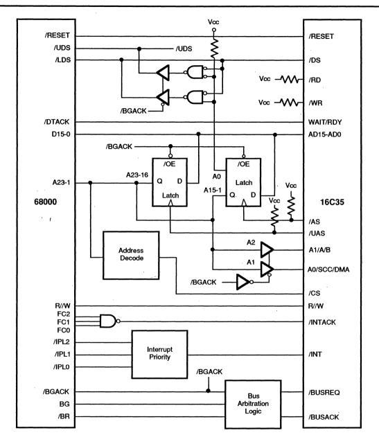
Figure A-3. ISCC Interface to a 68000 Microprocessor
