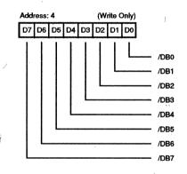
Figure 25. Select Enable Register
