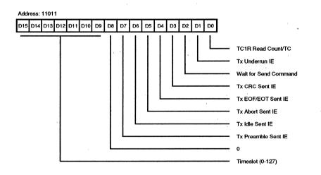
Figure 46b. Transmit Interrupt Control Register
