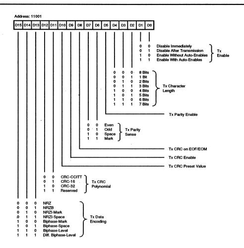
Figure 44. Transmit Mode Register
