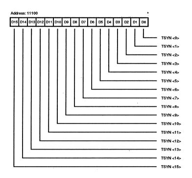
Figure 47. Transmit Sync Register
