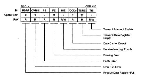
† /DCD0 - Depending on the condition of /DCD0 Pin.
