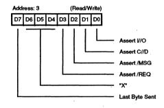
Figure 23. Target Command Register
