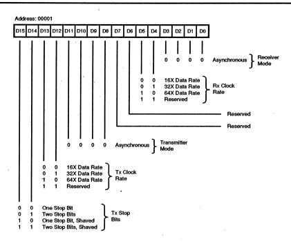
Figure 9. Channel Mode Register, Asynchronous Mode
