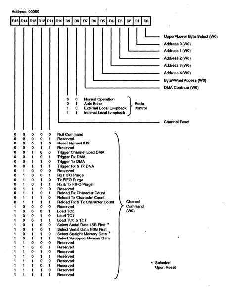
Figure 7. Channel Command/Address Register
