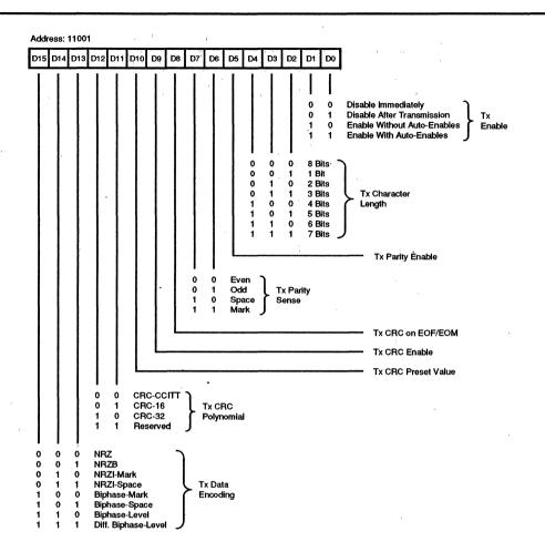
Figure 44. Transmit Mode Register
