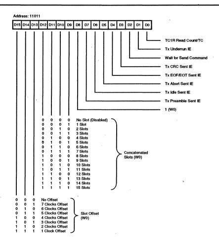
Figure 46c. Transmit Interrupt Control Register
