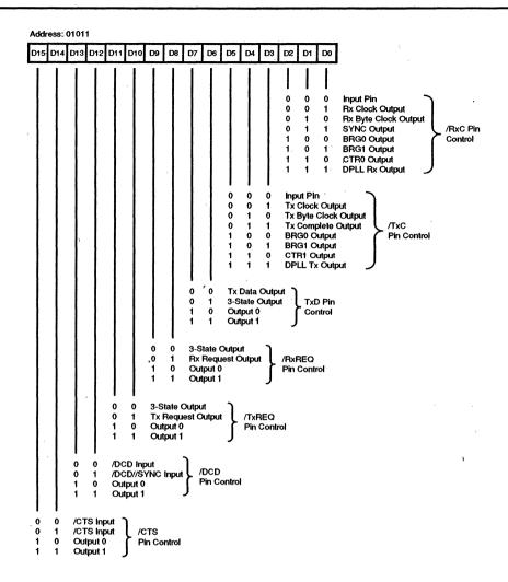
Figure 30. I/O Control Register
