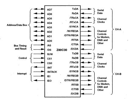
Figure 7. Z80C30 Pin Functions
