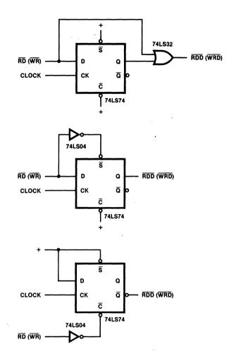
Figure 4. Delaying  $\overline{RD}$  or  $\overline{WR}$
