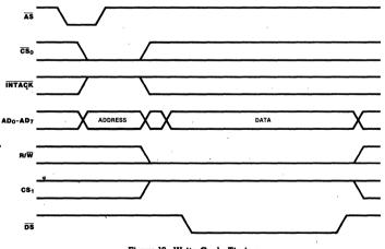
Figure 16. Write Cycle Timing
