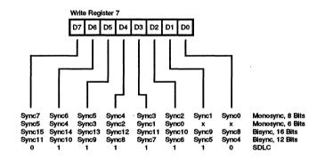
Figure 18. Write Register Bit Functions (Continued)
