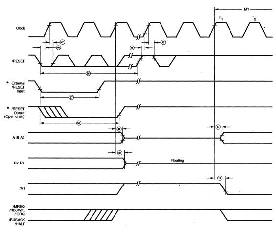
\* 84C13/15 Only Reset Output is Enabled
