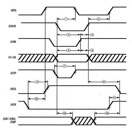
Figure 46. DMA Write (Non-Block Mode) Target Send Cycle
