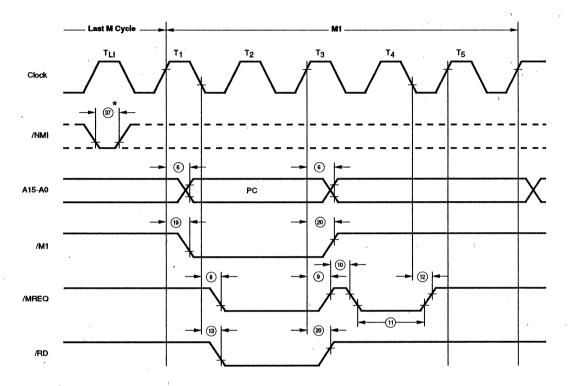
\* Although /NMI is an asynchronous input, to guarantee its being recognized on the following machine cycle, /NMI's falling edge must occur no later than the rising edge of the clock cycle preceding the last state of any instruction cycle ( $T_{U}$ ).
