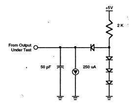
Figure 54. Standard Test Load
