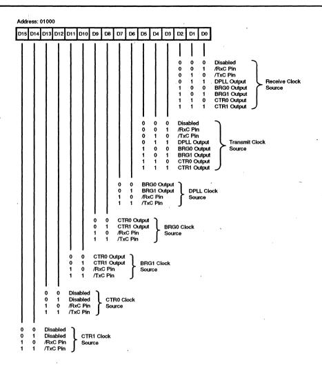
Figure 27. Clock Mode Control Register
