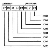
Figure 11. Select Enable Register
