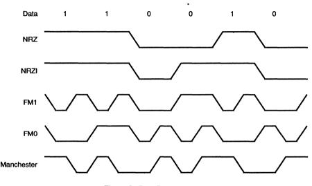
Figure 2. Data Decoding Formats
