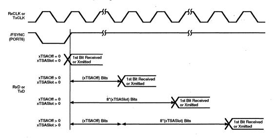
Figure 1. Start of Received or Transmitted Data in a TSA Application
