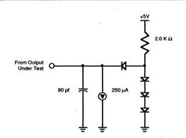
Figure 27. Standard Test Load
