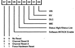
Figure 17. Write Register Bit Functions (Continued)
