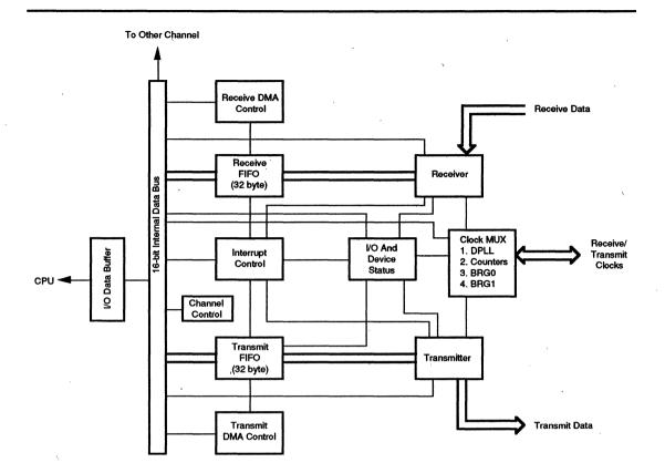
Figure 2. At The Heart of the dual-channel communications board is the Z16C30 Universal Serial Controller chip, which supports 10 different protocols and eight encoding formats. In the upper portion of the diagram, serial data from the receiver is placed in a 32-byte FIFO buffer prior to being placed onto the 16-bit internal bus under DMA control. Similarly, data to be transmitted from the bus is placed in the FIFO transmit buffer and then sent in serial form by the transmitter.
