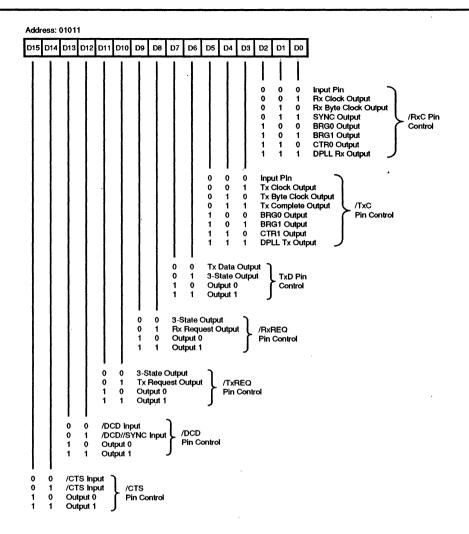
Figure 30. I/O Control Register
