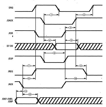
Figure 48. DMA Read (Non-Block Mode) Target Receive Cycle
