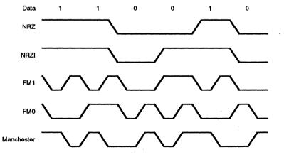
Figure 14. Data Encoding Methods
