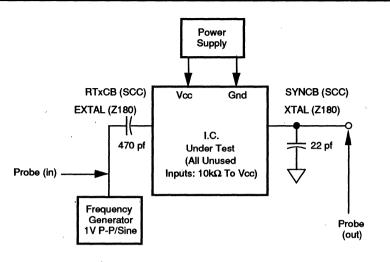
Figure 6. Gain Measurement
