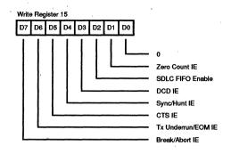
Figure 10. Write Register Bit Functions (Continued)
