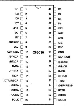
Figure 2. Z85C30 DIP Pin Assignments
