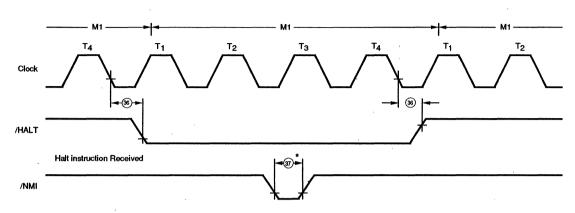
\* Although /NMI is an asynchronous input, to guarantee its being recognized on the following machine cycle, /NMI's falling edge must occur no later than the rising edge of the clock preceding the last state of any instruction cycle (T<sub>1</sub>).
