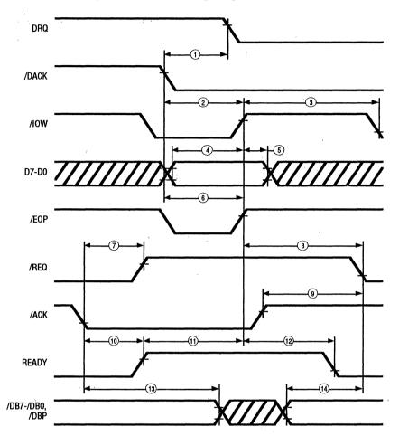
Figure 50. DMA Write (Block Mode) Target Send Cycle
