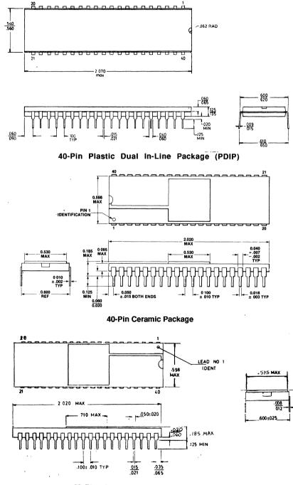
40-Pin Ceramic Dual In-Line Package (DIP)
