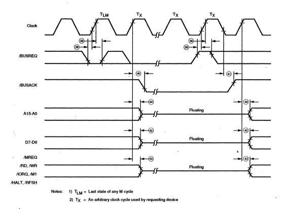
Figure 46. BUS Request/Acknowledge Cycle (See Table A) Halt acknowledge cycle. Figure 47 shows the timing for Halt acknowledge cycle.
