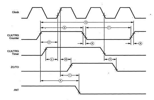
Figure 55. Counter/Timer Timing (See Table E)
