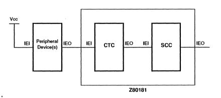
Figure 77. Peripheral Device as Part of the Daisy Chain
