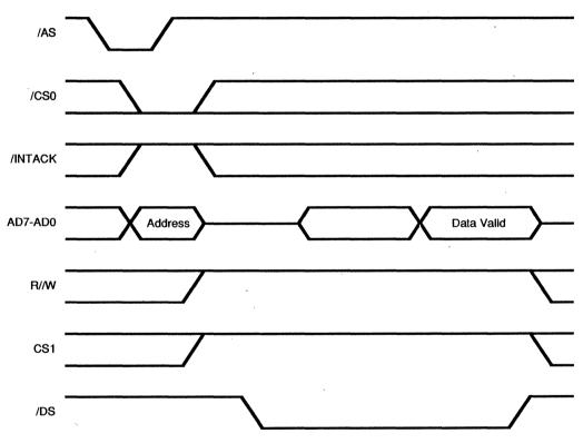
Figure 22. Read Cycle Timing
