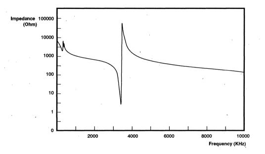
Figure 5. Ceramic Resonator Reactance
