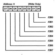
Figure 5. Output Data Register
