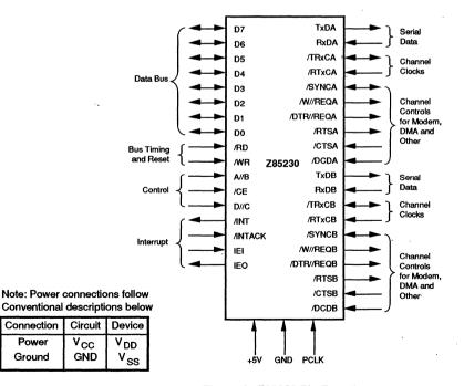
Figure 4. Z85230 Pin Functions
