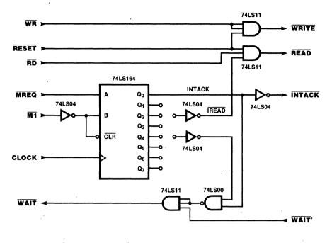
Figure 5. Z80A/Z80B CPU to Z8500/Z8500A Peripheral Interrupt Acknowledge Interface Logic
