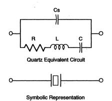
Figure 4. Quartz Oscillator
