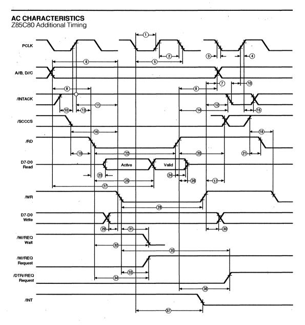
Figure 60. Read/Write Timing
