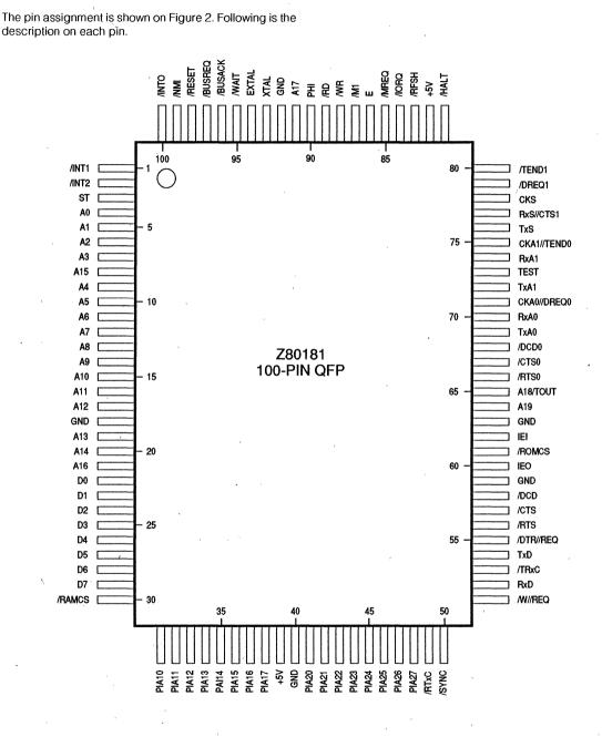
Figure 2. Z80181 Pin-out Assignment
