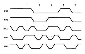
Figure 11. Data Encoding Methods
