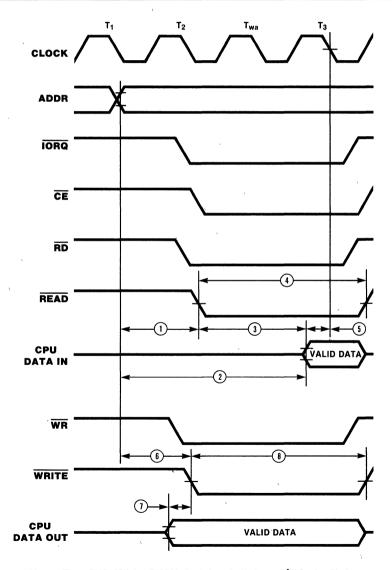
Figure 3b. Z80B CPU to Z8500A Peripheral Minimum I/O Cycle Timing
