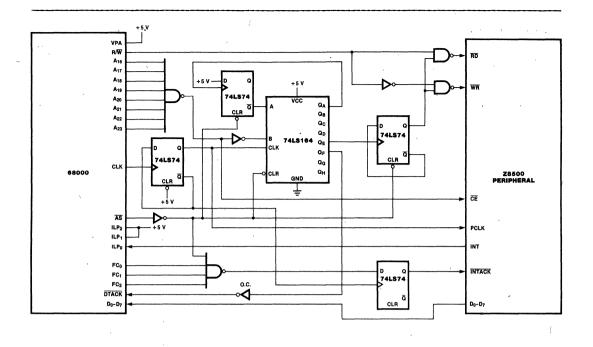
Figure 7. Hardware Diagram for DIACK Interface
