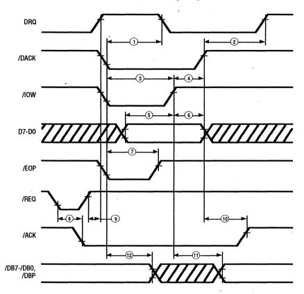
Figure 47. DMA Write (Non-Block Mode) Initiator Send Cycle
