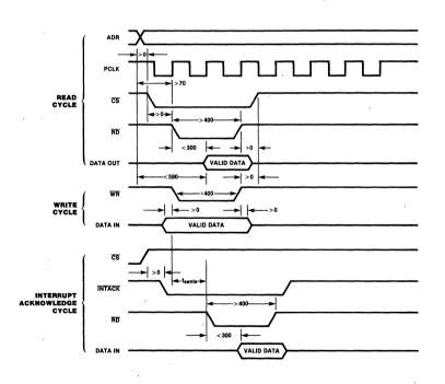
Figure 2. Z8500 Interface Timing (4 MHz)
