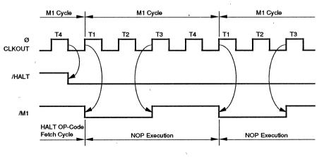
Figure 31. Timing of RUN Mode (at Halt Instruction Command Execution)
