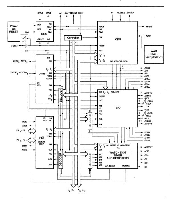
Figure 5(b). Block Diagram for 84C13/C15 IPC
