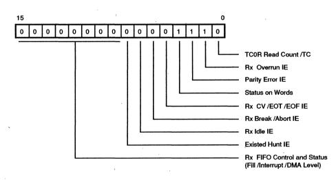
Figure 9. Receive Interrupt Control Register
