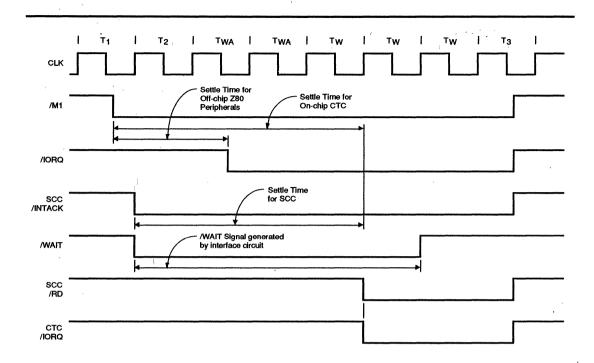
Figure 78. Interrupt Acknowledge Cycle Timing
