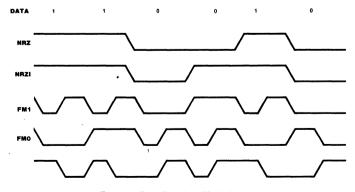
Figure 6. Data Encoding Methods
