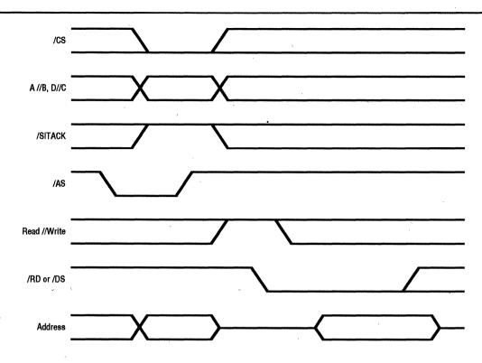
Figure 4. The USC/Ethernet Interface handles reading and writing of data through the two serial channels. Here, after the controller acknowledges a network request, raw IEEE 802.3 data is read from an Ethernet serial link.
