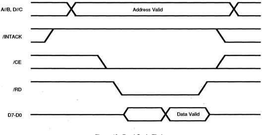
Figure 19. Read Cycle Timing
