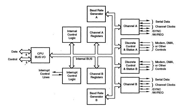
Figure 7. Block Diagram of SCC Architecture
