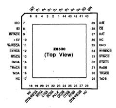
Figure 2c. Chip Carrier Pin Assignments, Z8530
