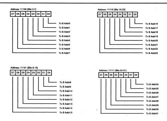
Figure 26. Transmit DMA Address Register Channel B
