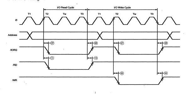
**Figure 62. CPU Timing** (/IOC = 0) (I/O Read Cycle, I/O Write Cycle)
