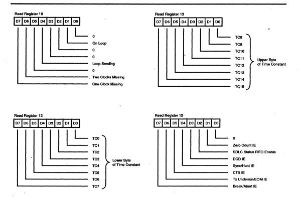
Figure 19. Read Register Bit Functions (Continued)
