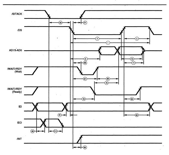
Figure 70. Non-Multiplexed /DS Interrupt Acknowledge Cycle
