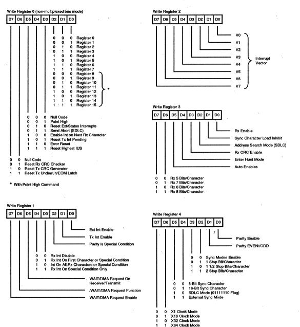
Figure 18. Write Register Bit Functions
