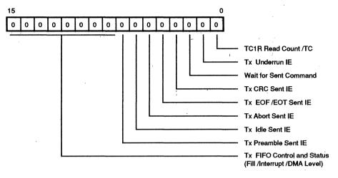
Figure 10. Transmit Interrupt Control Register
