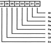
All Sent Residue Code 2 Residue Code 1 Residue Code 0 Parity Error Rx Overrun Error CRC/Framing Error End of Frame (SDLC)
