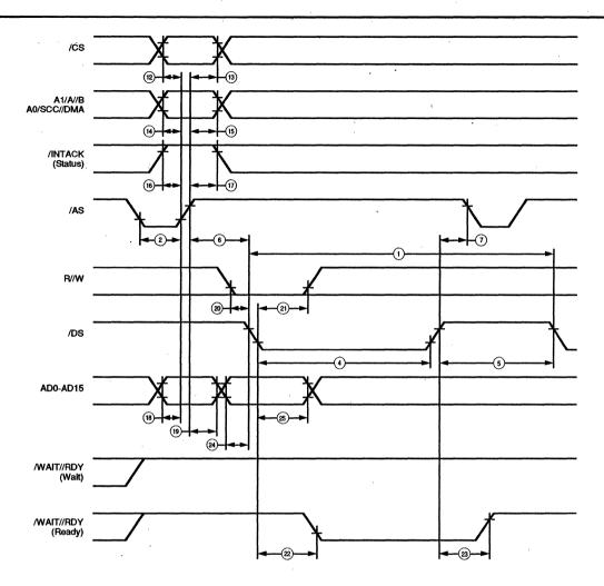
Figure 29. Multiplexed /DS Write Cycle
