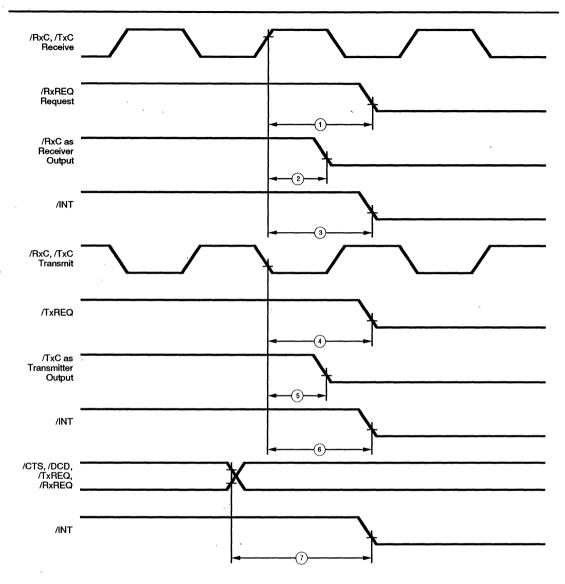
Figure 76. Z16C30 System Timing
