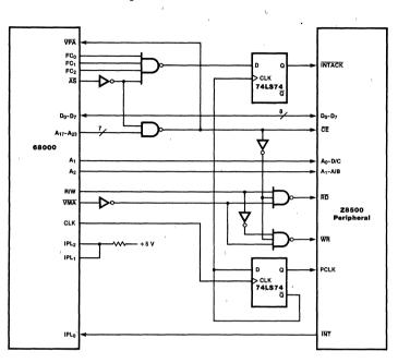
Figure 4. Interface Using the VPA Cycle
