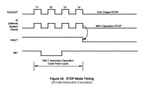
In STOP Mode, the on-chip CGC unit is stopped at T4 Low state of HALT instruction execution. Therefore, clock output (CLKOUT), operation of Watch Dog Timer, CPU, PIO, CTC, SIO are stopped.
