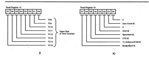
Figure 49. SCC Read Register Bit Functions (Continued)
