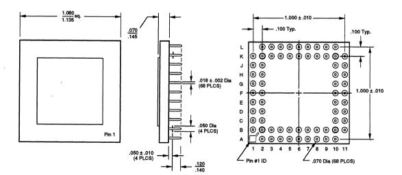
68-Pin Pin Grid Array (PGA)
