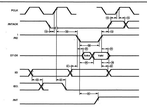
Figure 28. Z85C30 Interrupt Acknowledge Timing Diagram
