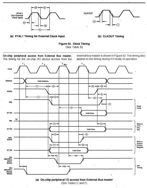
Figure 53. On-chip Peripheral Timing from External Bus master
