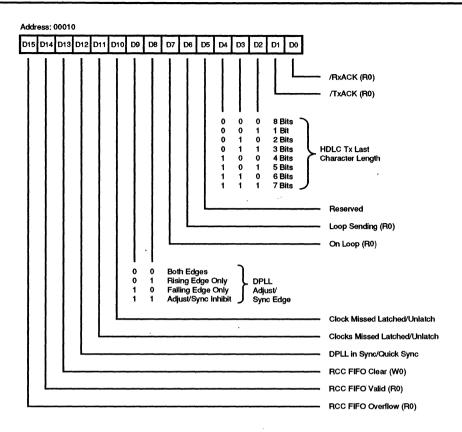
Figure 21. Channel Command/Status Register
