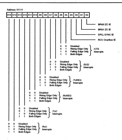
Figure 34. Status Interrupt Control Register
