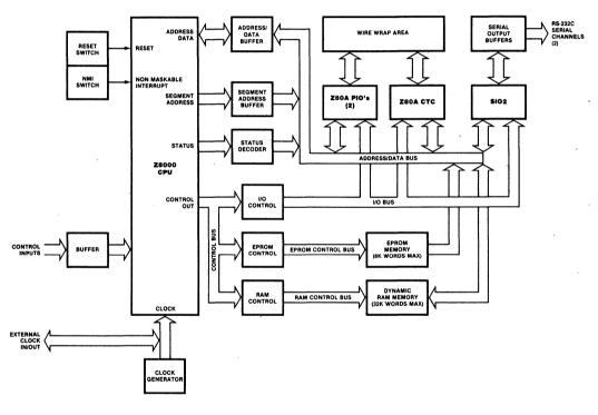
Figure 3. Block Diagram of Z8000 DM
