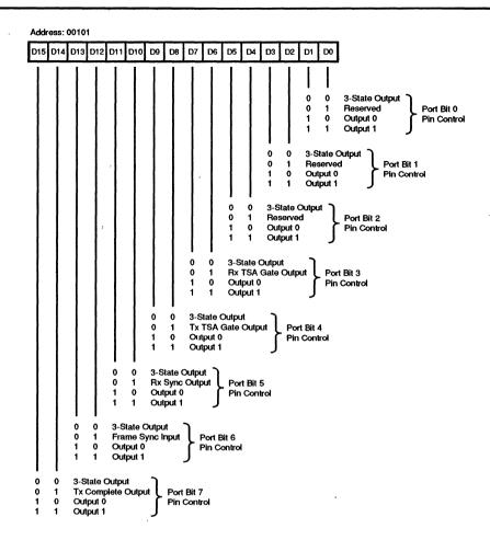
Figure 24. Port Control Register
