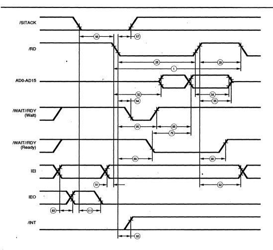
Figure 71. Non-Multiplexed /RD Pulsed Interrupt Acknowledge Cycle
