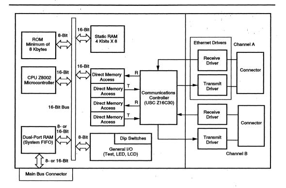
Figure 1. Dual-Channel Communications Board for an IBM 80386 PC consists of four main sections: The communications controller (a Z16C30 Universal Serial Controller), an interface to the PC's bus, buffer memory, and two communications channels. In this application, Channel A drives an Ethernet interface and Channel B, drives a laser printer through an RS-232 port.
