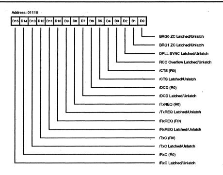
Figure 33. Miscellaneous Interrupt Status Register
