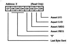
Figure 42. Target Command Register
