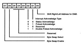
Figure 8. Bus Configuration Register (BCR)
