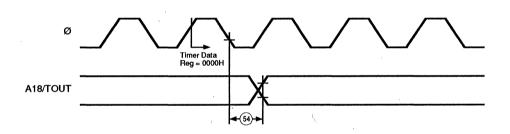
Figure 66. Timer Output Timing
