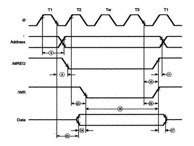
Figure 3. Z180 Memory Write Cycle Timing (One Wait State)
