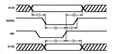
Figure 68. CPU Write Cycle
