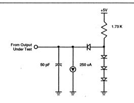
Figure 3. Standard Test Load
