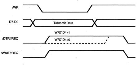
Figure 13. DMA Request on Transmit Deactivation Timing
