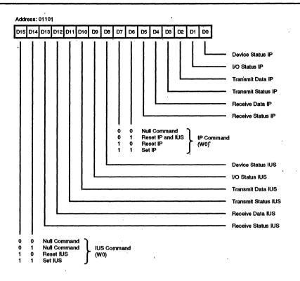
Figure 32. Daisy-Chain Control Register
