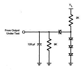
Figure 43. Standard Test Load
