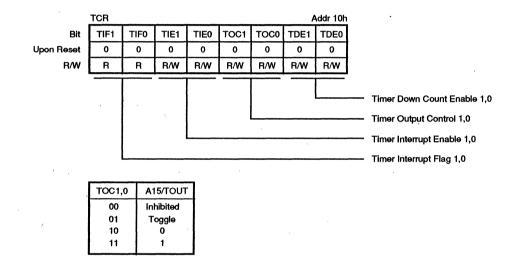
Figure 27. Timer Control Register
