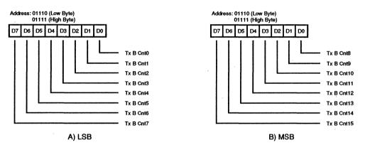
Figure 22. Transmit DMA Count Register Channel B
