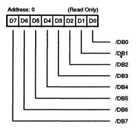
Figure 39. Current SCSI Data Register
