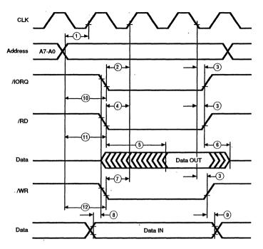
Figure 75. Read/Write External BUS Master Timing
