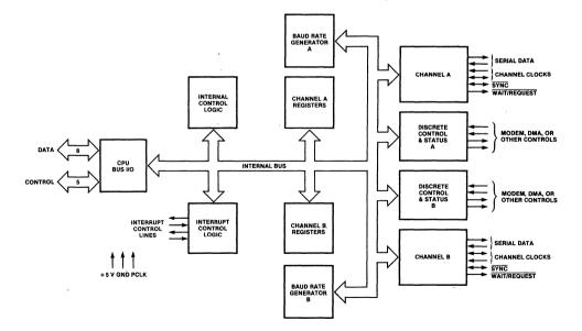
Figure 8. Block Diagram of SCC Architecture
