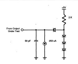
Figure 54. Standard Test Load
