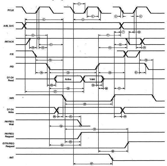
Figure 25. Z85230 Read and Write Timing Diagram
