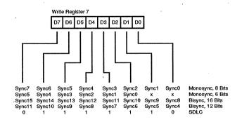
Figure 9. Write Register Bit Functions (Continued)
