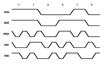
Figure 7. Data Encoding Methods
