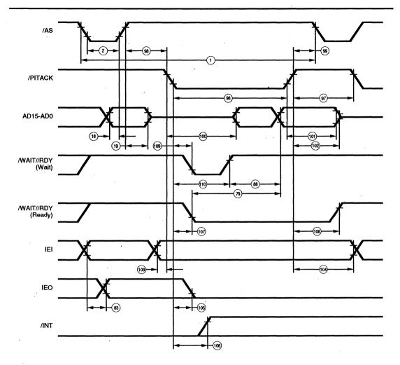
Figure 69. Multiplexed Pulsed Interrupt Acknowledge Cycle
