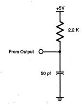
Figure 56. Open-Drain Test Load
