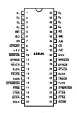
Figure 2a. DIP Pin Assignments, Z8530
