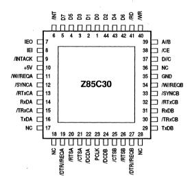
Figure 4. Z85C30 PLCC Pin Assignments
