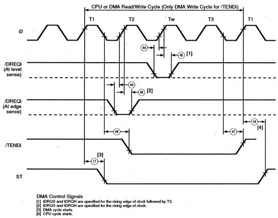
Figure 63. DMA Control Signals
