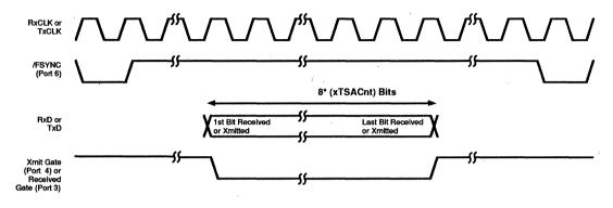
Figure 2. Length of Received or Transmitted Data in a TSA Application
