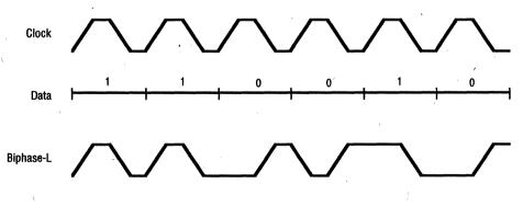
Figure 2. Manchester II (Biphase-Level) Data Encoding
