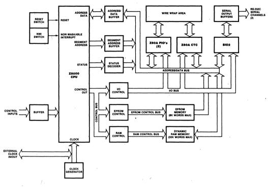
Figure 2. Block Diagram of Z8000 DM
