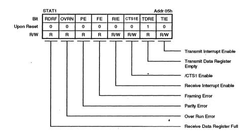
Figure 12. ASCI Status Register (Ch 1)
