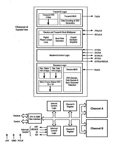
Figure 1. ESCC Block Diagram
