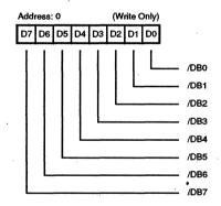
Figure 18. Output Data Register
