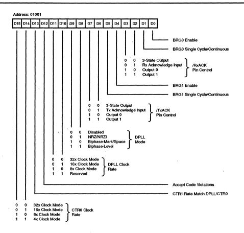
Figure 28. Hardware Configuration Register
