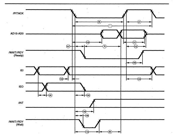
Figure 72. Non-Multiplexed /RD Interrupt Acknowledge Cycle
