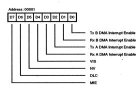
Figure 13. Interrupt Control Register
