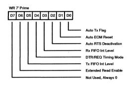
Figure 12. Write Register 7' (7 prime)
