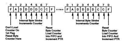
Figure 17. SDLC Byte Counting Detail
