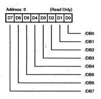
Figure 26. Current SCSI Data Register
