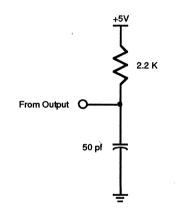
Figure 24. Open-Drain Test Load
