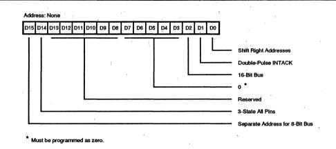
Figure 53. Bus Configuration Register
