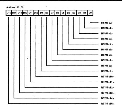
Figure 39. Receive Sync Register
