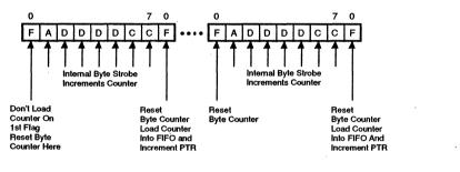
Figure 16. SDLC Byte Counting Detail
