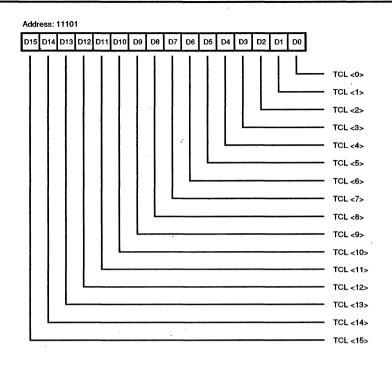
Figure 48. Transmit Count Limit Register
