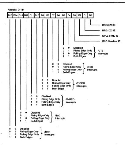
Figure 34. Status Interrupt Control Register
