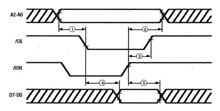
Figure 45. CPU Read Cycle
