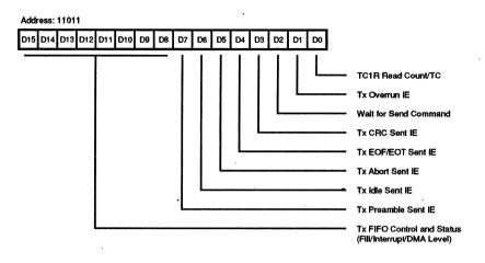
Figure 46. Transmit Interrupt Control Register
