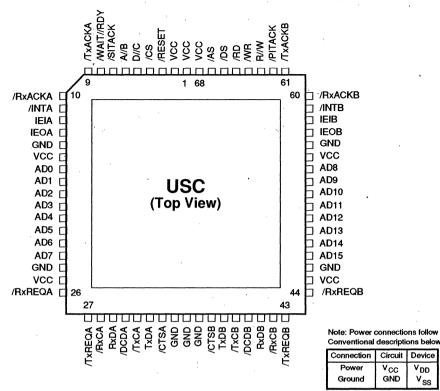
Figure 3. Pin Assignments
