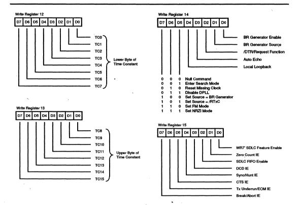
Figure 18. Write Register Bit Functions (Continued)
