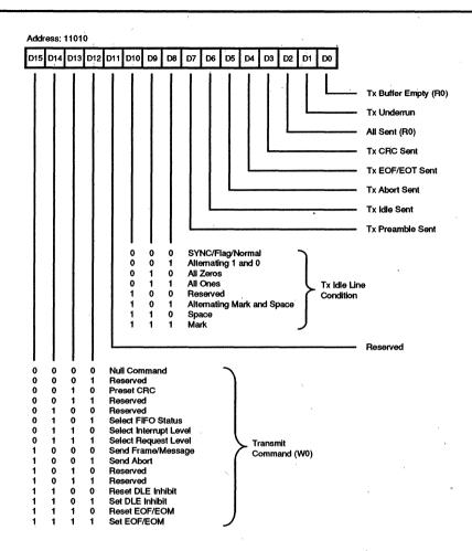
Figure 45. Transmit Command/Status Register
