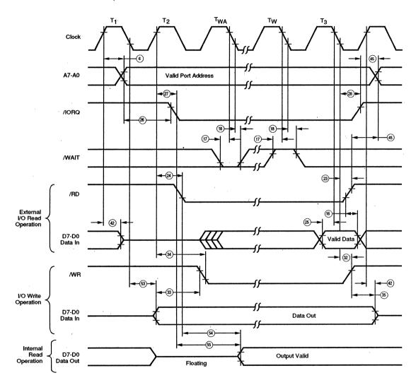
Note:  $T_{WA}$  = One wait cycle automatically inserted by CPU
