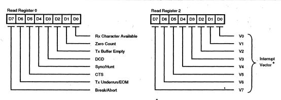
\* Modified if VIS bit in Write register 9 is set.
