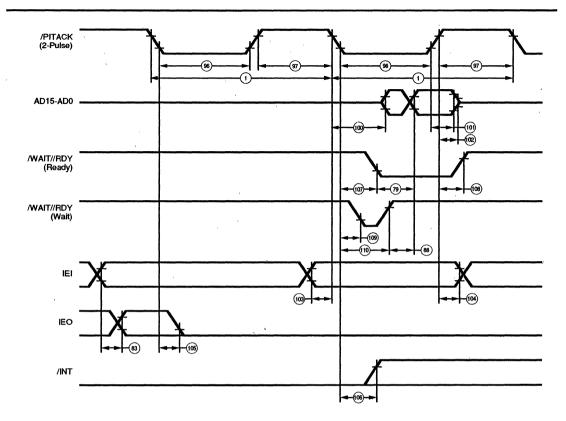
Figure 74. Non-Multiplexed Double-Pulse Intack Cycle
