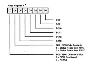
Can only be accessed if the SDLC FIFO enhancement is enabled (WR15 bit D2 set to 1)
