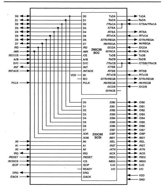
Figure 1. Z85C80 SCSCI Block Diagram
