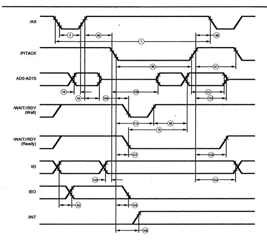
Figure 69. Multiplexed Pulsed Interrupt Acknowledge Cycle
