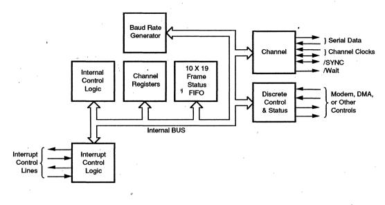
Figure 4. SCC Block Diagram
