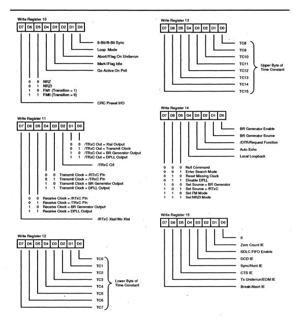
Figure 17. Write Register Bit Functions (Continued)
