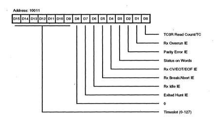
Figure 38b. Receive Interrupt Control Register
