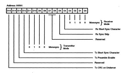
Figure 13. Channel Mode Register, Monosync Mode
