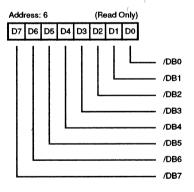
Figure 13. Input Data Register
