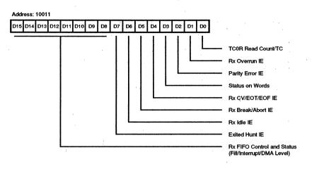
Figure 38. Receive Interrupt Control Register
