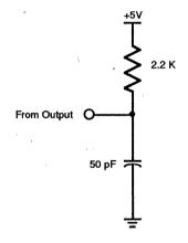
Figure 26. Open-Drain Test Load
