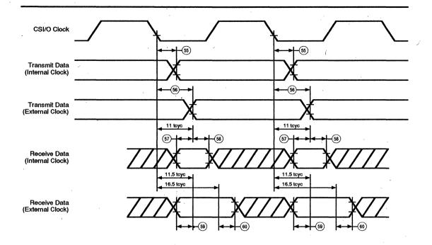
Figure 68. CSI/O Receive/Transmit Timing
