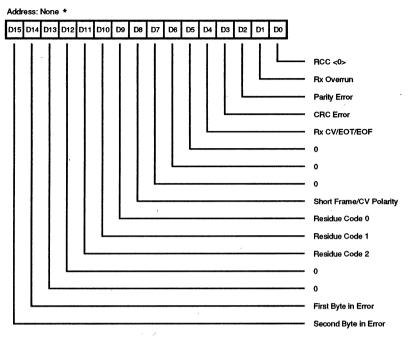
\* Refer to Figure 22 (Channel Control Register) Bits 6-7 for Access Method
