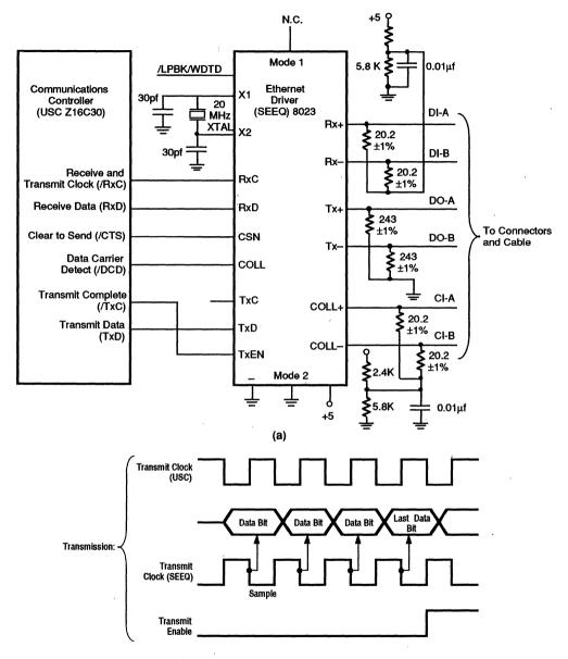
Note: /Transmit Clock Pin of USC is Programmed to be used as a Signal to Flag the End of Transmit.
