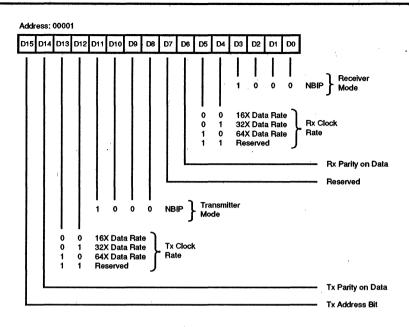
Figure 17. Channel Mode Register, NBIP Mode
