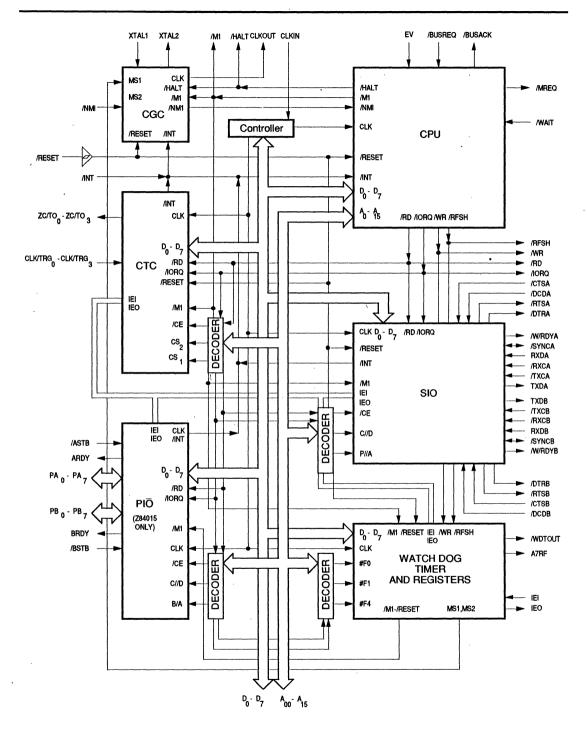
Figure 5(a). Block Diagram for 84013/015 IPC
