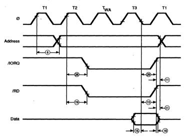
Figure 7. Z180 I/O Read Cycle Timing (/IOC = 0)
