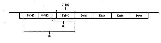
Figure 4. Detecting 5 - or 7-Bit Synchronous Characters
