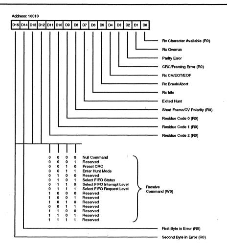
Figure 37. Receive Command Status Register
