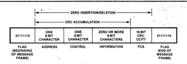
Figure 1. Fields of the SDLC Transmission Frame
