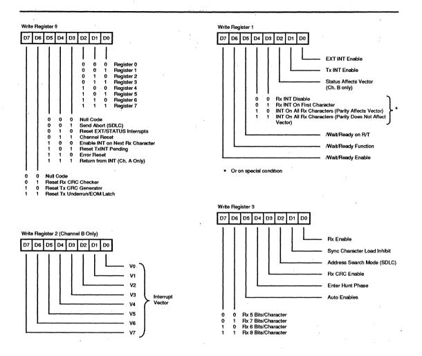
Figure 21. SIO Write Registers
