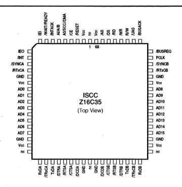
Figure 2. Pin Assignments
