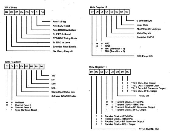
Figure 18. Write Register Bit Functions (Continued)
