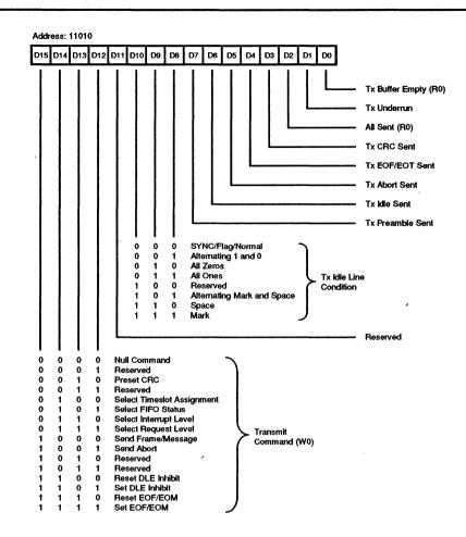
Figure 45. Transmit Command/Status Register
