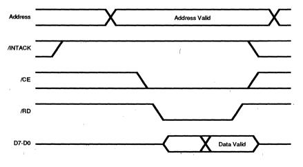
Figure 10. SCC Read Cycle Timing
