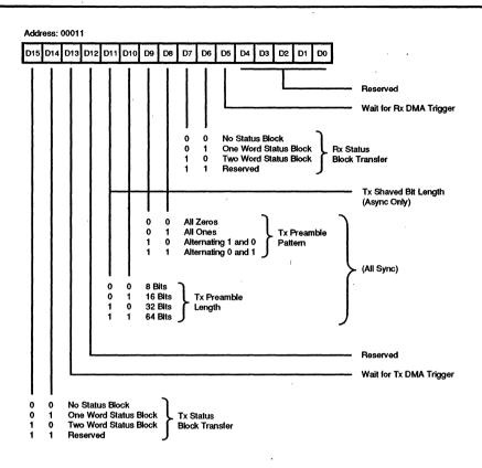
Figure 22. Channel Control Register
