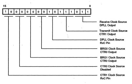
Figure 3. Clock Mode Control Register
