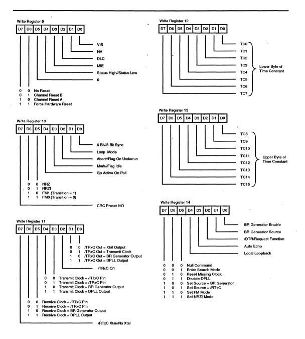
Figure 9. Write Register Bit Functions (Continued)
