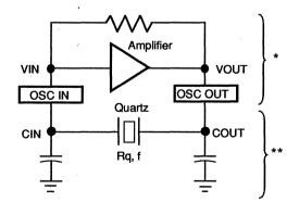
Inside chip, feedback resistor biases the amplifier in the high gm region.
