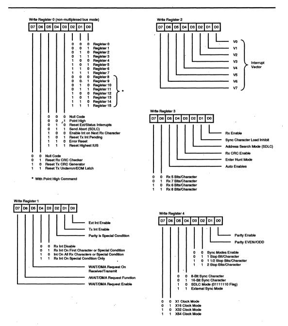
Figure 10. Write Register Bit Functions
