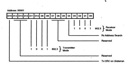
Figure 18. Channel Mode Register, 802.3 Mode
