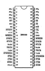
Figure 2b. DIP Pin Assignments, Z8030
