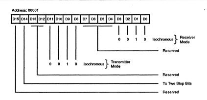
Figure 11. Channel Mode Register, Isochronous Mode
