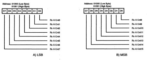
Figure 19. Receive DMA Count Register Channel A
