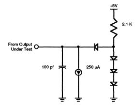
Figure 23. Standard Test Load
