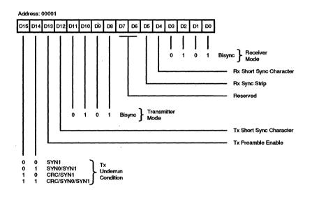
Figure 14. Channel Mode Register, Bisync Mode
