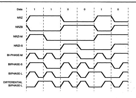
Figure 5. Data Encoding
