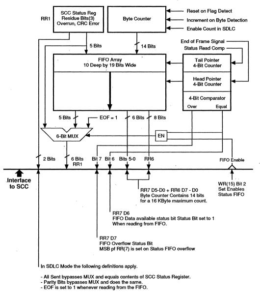
Figure 15. SDLC Frame Status FIFO
