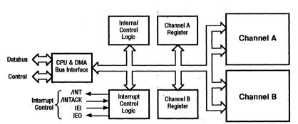
Figure 1. SCC Block Diagram
