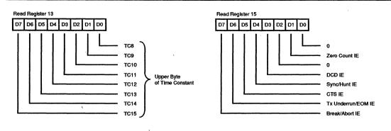
Figure 18. Read Register Bit Functions (Continued)
