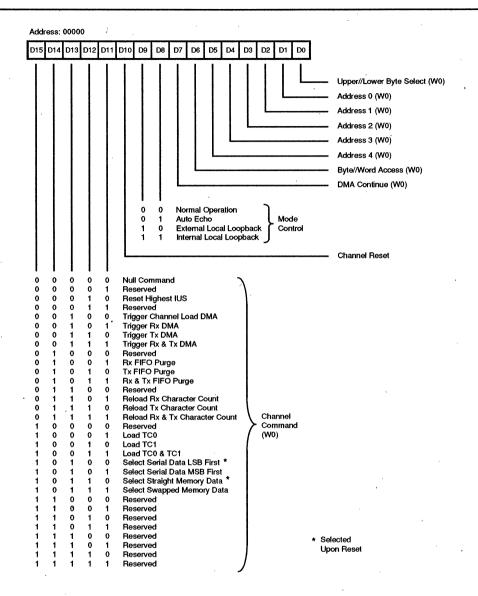
Figure 7. Channel Command/Address Register
