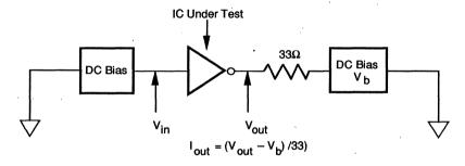
Figure 7. Transconductance (gm) Measurement
