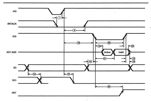
Figure 32. Z80C30 Interrupt Acknowledge Timing Diagram
