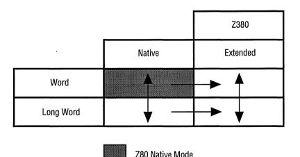
Figure 3-1. Z380<sup>™</sup> CPU Operation Modes
