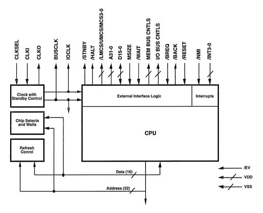
Figure 1. Z380 Functional Block Diagram
