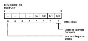
Figure 6-1. Interrupt Enable Register
