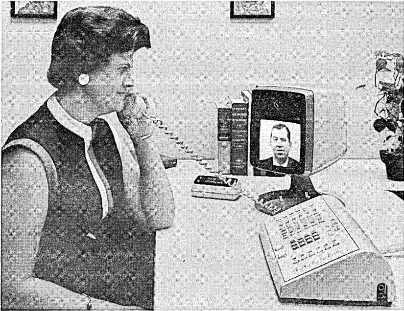
Fig. 1—A modern PBX or centrex attendant position, arranged to handle Picturephone service.
