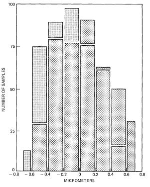
Fig. 5-Data on groove opening variations.
