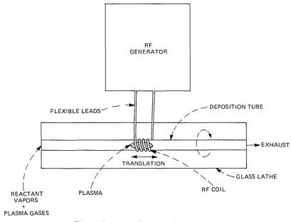
Fig. 1—Apparatus for preparing preforms.
