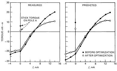
Fig. 12-Predicted and measured effect of optimized parameters.
