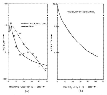
Fig. 2—(a)Visibility function for Checkered Girl and Teri using a two-dimensional one neighbor masking function. (b) Visibility function for noise added to  $H_1$  as a function of max ( $|H_2|$ ,  $|H_4|$ ).
