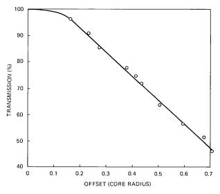
Fig. 11—Measured transmission vs. transverse offset.
