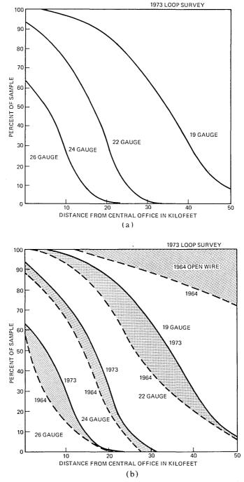
Fig. 7—(a) Gauge distribution. (b) Gauge distributions, 1973 vs 1964 surveys.
