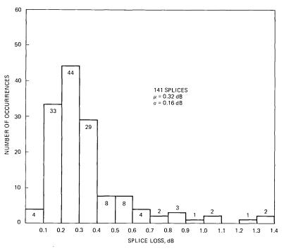
Fig. 8—12  $\times$  12 array splice, connector 48 to inverted connector 49.
