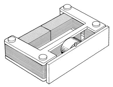
Fig. 11-Ringer motor with straight armature.
