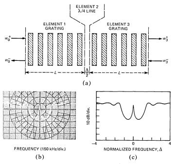
Fig. 2—(a) Diagram of a grating resonator in the external transmission configuration. (b) The transmission spectrum at ~145.5 MHz for a resonator on YZ-LiNbO<sub>3</sub> using Tidiffused gratings with  $\Lambda = 12 \ \mu m$  and  $L = 6.48 \ mm$ . (c) The calculated transmission spectrum for the device in (b) using  $\kappa = 3.74 \ mm$  and  $\alpha = 0.036 \ mm$ <sup>-1</sup>.
