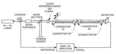
Fig. 6-Loss measurement setup.
