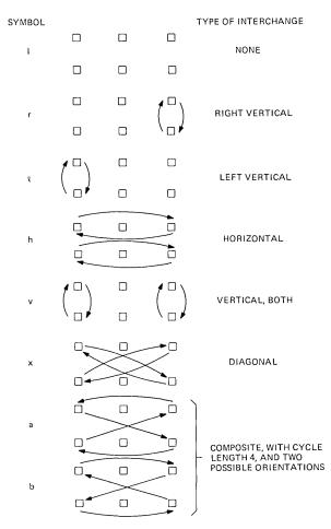
Fig. 14—Possible interchanges of outer switches.
