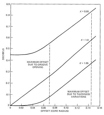
Fig. 6-Splice loss as a function of offset.
