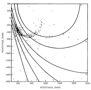
Fig. 21—Nonloaded loop input impedances at 3 kHz. RL circles based on 500-type telephone set impedances (900 ohm + 2.16  $\mu F$  cable termination at the central office).
