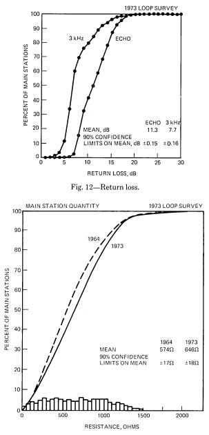
Fig. 13—Calculated resistance to main station.
