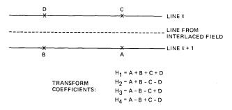
Fig. 1—Definition of Hadamard coefficients. A, B, C, D are the pel positions, and  $H_1$ ,  $H_2$ ,  $H_3$ ,  $H_4$  are the Hadamard coefficients.
