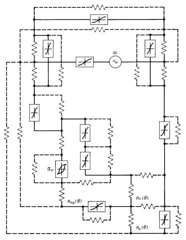
Fig. 14—Lumped element model of P-ringer motor.
