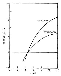
Fig. 15-P-type ringer motor measured torque curves.
