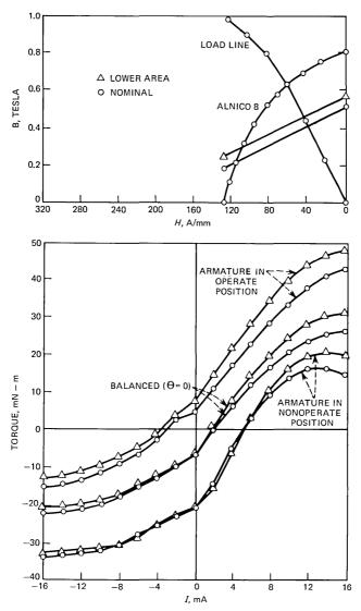
Fig. 6—Typical program output showing the predicted effect of decreasing the crosssectional area of a magnetic shunt member.
