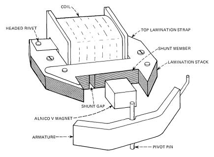
Fig. 2-Rocking-armature motor.
