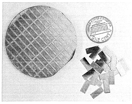
Fig. 7-Laser-scribed silicon wafer.
