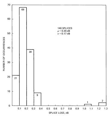
Fig. 7—12  $\times$  12 array splice, connector 48 to connector 49.
