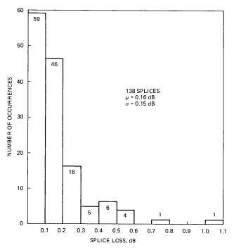
Fig. 9—12  $\times$  12 array splice, connector 48 to connector 50.
