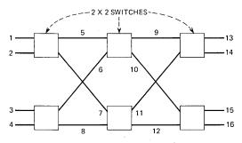
Fig. 10—Simple 3-stage Clos network.
