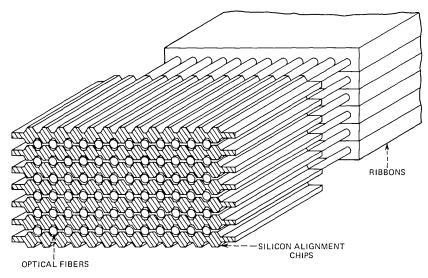
Fig. 1—Schematic of a multifiber array connector.
