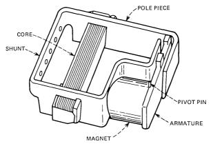
Fig. 13—P-type ringer motor.
