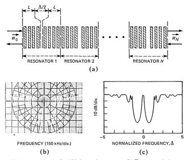
Fig.3—(a) Diagram of cascade of N identical resonators. (b) The transmission spectrum at 145.5 MHz of a cascade of three identical resonators with  $\Lambda = 12 \,\mu$ m and L = 3.84 mm. (c) The calculated transmission spectrum for the device in (b) using  $\kappa = 3.55$  cm<sup>-1</sup> and  $\alpha = 0.027$  cm<sup>-1</sup>.
