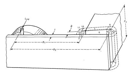
Fig. 18—Flux paths at gap B.
