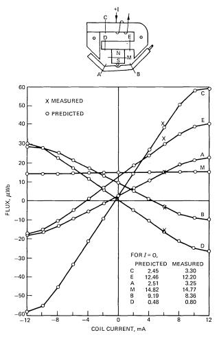
Fig. 7—Flux versus coil current, predicted and measured.
