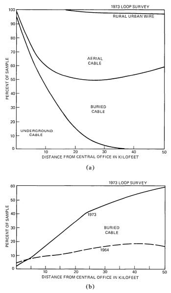
Fig. 8—Type of construction. (a) Distribution. (b) Buried cable.
