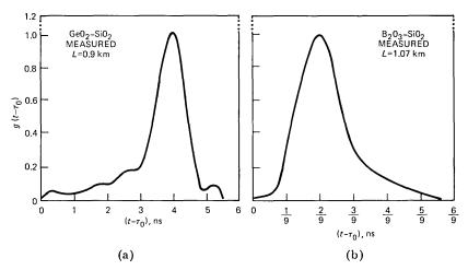
Fig. 1—Measured (deconvolved) impulse responses for (a) a GeO<sub>2</sub>–SiO<sub>2</sub> fiber with  $\alpha < \alpha_{opt}$ ; (b) a B<sub>2</sub>O<sub>3</sub>–SiO<sub>2</sub> fiber with  $\alpha \approx \alpha_{opt}$ .
