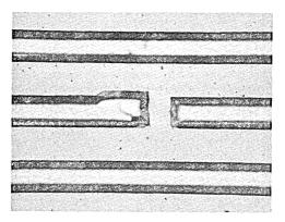
Fig. 3—Bridged groove on a silicon chip.
