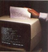
Try this on your favorite CRT! With the 2621P, you just hit a key and in seconds you have hard copy of your CRT display. The built-in thermal printer prints upper and lower case at up to 120 cps.
