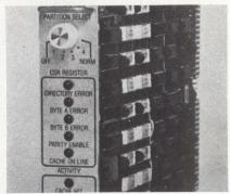
Series 8000 provides plug compatible cache memory for DEC's PDP-11/34, /35, and /40. The cache has 4k x 25 memory that can store 8k bytes of data. Address map partition maximizes system enhancement by adding memory flexibility. A parity error circuit with LED indicators is incorporated and a Unibus addressable CSR allows cache to be turned on and off from the front panel. Diagnostic software is included. Minntronics Co, Inc, 2599 White Bear Ave, St Paul, MN 55109.
