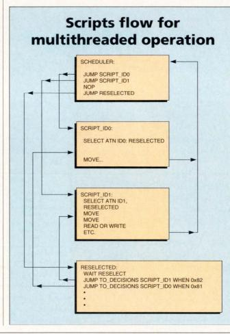
SCSI Scripts make it easy to have more than one task active at a time. The main driver running the host computer keeps track of I/O requests in a table or scheduler. Each time an application program requests a new I/O instruction, the main driver enters a Scripts Jump instruction into the scheduler. Each time an I/O is completed, the main driver replaces the I/O request with an NOP instruction.
