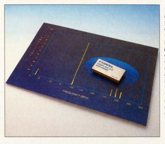
The ADS-930, a 16bit, 500-kHz converter from Datel, offers several features geared toward signal processing applications. The device offers an SNR of 87 dB and -90 dB harmonics. An onboard FIFO provides smoother operation with DSP chips while reducing the number of DSP interrupt instruction cycles necessary.
