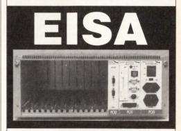
Shown here is a modular EISA industrial computer, with a passive backplane providing six EISA bus master slots, one slot-specific slot and four AT slots.
