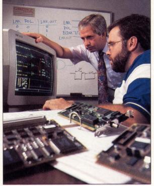
At Cabletron Systems, Bob Lapointe, manager of PC networking products (standing) and senior hardware engineer, Paul Sprague, work toward implementing their design for a LAN controller as a full ASIC. The Cabletron design team put four PALs, a bunch of external logic, plus added functionality into a Xilinx XC3030 FPGA and then migrated to an S-MOS gate array with the help of Viewlogic's Retargeter tool.
