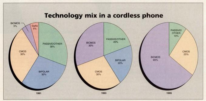
Today, a cellular phone makes use of a number of different technologies—some expensive. By 1995, the aim is to bring down the cost of the phone by manufacturing the bulk of the radio frequency/power devices in BiCMOS, and the digital logic in CMOS.
