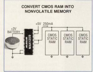
The MAX1259 output makes it possible to backup several CMOS RAM chips.
