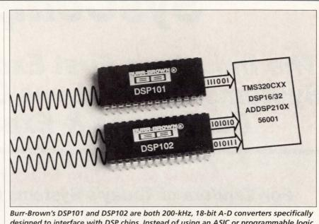
designed to interface with DSP 102 are both 200-KHZ, 18-bit A-D converters specifically designed to interface with DSP chips. Instead of using an ASIC or programmable logic to implement the interface, designers can connect the DSP101/102 directly to a DSP. The parts interface with the serial ports on DSP chips from Analog Devices, AT&T, Motorola, and Texas Instruments.
