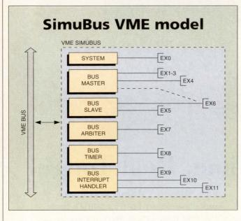
According to Logic Automation, a designer using SimuBus can see a broad range of interactions between a board under development and the rest of the system. The SimuBus model contains extensive error checks on the simulation in progress, including set-up, hold and pulse widths on all bus transactions.
