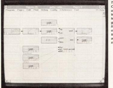
The Gellix CASE tool lets users put control programs together by graphically linking precompiled routines in a hierarchical structure. real-time response. For process control applications normally requiring response times in the 10- to 100-ms range, this is seldom a problem. In real-time, event-driven systems, however, the company points out that attention must be paid to CPU and I/O speeds.
