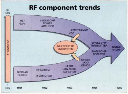
By 1995, a single RF chip is all that will be required for the transmitter/receive section of a cellular phone. This road map shows how Texas Instruments aims to get there.
