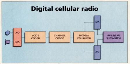
The basic building blocks of a cellular telephone include voice converters, a voice coder, channel codec, modem/equalizer, more converters, and a radio frequency subsystem. The functions of voice and channel coding, as well as modem equalization, are performed with a digital signal processor or an ASIC.
