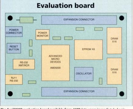
The Eval29200 evaluation board available from AMD lets users immediately begin prototyping Am29200-based designs. An on-board monitor allows quick access by a debugger running on a host development system.
