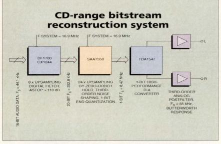
A 192× oversampled bitstream CD system can be designed using the Signetics SAA7350 in conjunction with an 8× oversampling filter, 1-bit D-A converter and third-order Butterworth filters.
