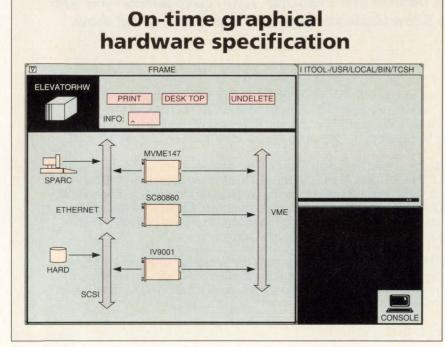
Graphical hardware descriptions of the mixed multiprocessor architecture provide documentation and the necessary information for users to quickly build pSOS+/Unison or VMEexec applications. The transparent multiprocessing of the operating systems works with these descriptions to insure fast incremental enhancement without application changes or painful rebuilding.
