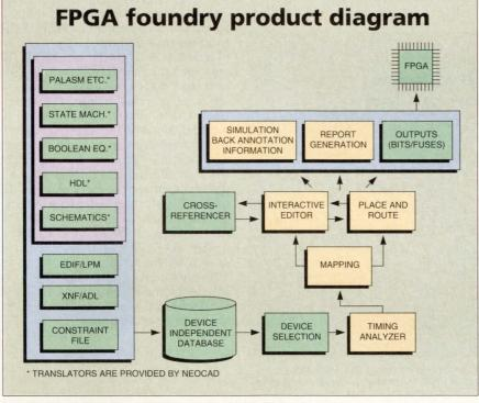
The device-independent FPGA Foundry design and layout toolset accepts designs in standard descriptions as well as vendor-specific netlist formats.
