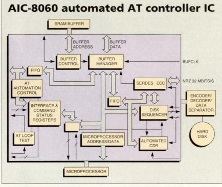
Offering several automation features, the AIC-8060 handles routine tasks across the AT bus. This frees the drive's microcontroller to concentrate more time on functions that are local to the disk drive, such as embedded servo control.
