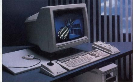
4,096 colors from a palette of 16.7 million. Shaded solids are rendered as flat or shaded surfaces using Phong or Gouraud shading algorithms. In addition, the 9300 supports rational cubic B-splines, which render curves according to their true mathematical definition, rather than as a series of vectors, and curved surfaces as true curves rather than a mosaic of polygons.
