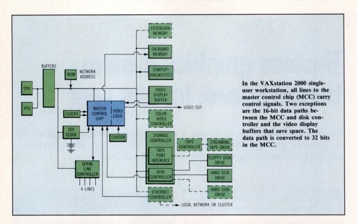
VAX station II, any 16 bits in a 1-Mpixel singleplane bit map—the bit map of the workstation's monitor—can be changed in 1.2  $\mu$ s. The bit-map transfer time is only 600 ns for any 32 bits moving over the CPU's native chip data path.
