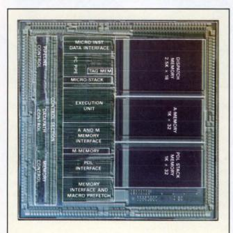
On the new dedicated Lisp processor, some 553,000 transistors are implemented in 1.25-micron CMOS design rules on the new dedicated Lisp processor. These transistors implement about 60 percent of the processor-chip circuits of a high-end Lisp workstation.
