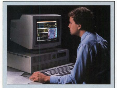
The Gate Array Worksystem from Tektronix provides Turnchip layout modules for specific gate array families. Users can enter schematics, select the gate array bonding package, view back annotation results, run simulations and view the automated layout in a multiwindow environment.
