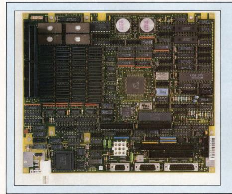
The basic hardware configuration of the VAX station 2000 is implemented on one  $10 ext{-} ext{-} ext{in.}$ system board, the largest that can fit into the desktop enclosure. Connectors are provided for daughter boards and for storage devices in the system and expansion enclosures. Communications, monitor and printer connectors on the rear edge of the system board protrude through openings in the rear panel.
