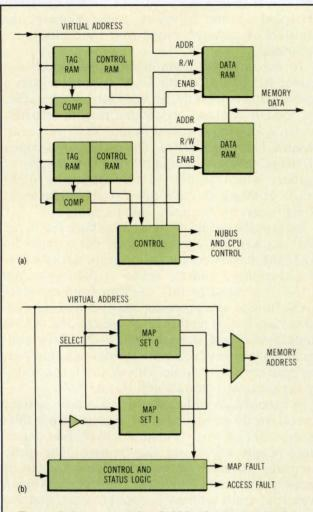
To maximize memory bandwidth, the mapper/cache module (a) contains a data cache divided into two parallel sections. Like the cache, the memory mapper (b) also is divided into two parallel operating sections to increase the hit rate.
