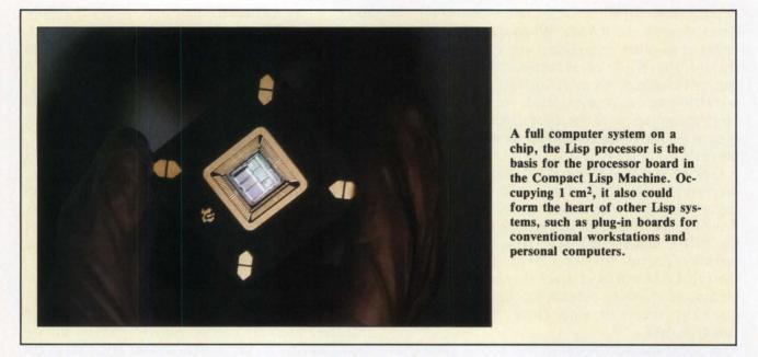
put is the goal here. A four-stage pipeline allows the execution of most microinstructions in a single clock cycle conservatively specified as 40 ns. The design goal for the chip is a 25-ns clock cycle.
