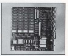
The board has five RS-232C ports, a Centronics port, a 16-bit bidirectional parallel printer port and a battery-backed clock/calendar. It offers 1 Mbyte (expandable to 5 Mbytes) of no-wait-state nonvolatile static RAM, a small computer systems interface initiator and a Shugart-compatible floppy controller. **Windrush Micro Systems**, Worstead Laboratories, N Walsham, Norfolk, England, NR28 9SA. **Circle 130**
