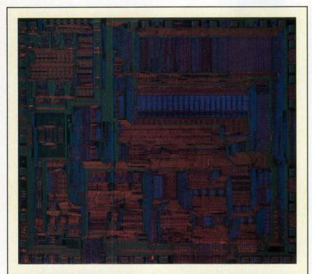
The Am79C30 Digital Subscriber Controller from Advanced Micro Devices is a high-integration device that supports the Link Access Protocol in the D channel and includes useful functions such as dual-tone multifrequency for dialing, codec and filter for audio processing, and an earpiece driver.
