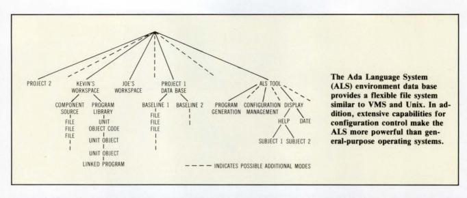
oriented file structures of VMS, Unix and most other multiuser file systems. The primary difference is that the ALS EDB has built-in configuration management controls.
