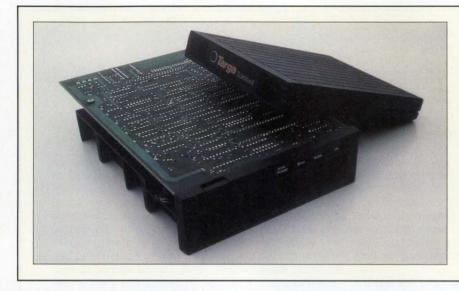
The Targa FD4500A nonvolatile cartridge RAM drives are electronically compatible with halfheight,  $5\frac{1}{4}$ -in. floppy drives and controllers. Cartridges with capacities of 360 and 720 kbytes are available. The drive can be used with an existing floppy controller in the system, and the system can boot from the cartridge drive just like from a floppy drive.
