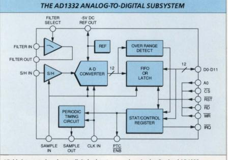
Highly integrated analog-to-digital subsystems, such as Analog Devices' AD1332, can pack all the necessary stages of an ac data-conversion system into a single chip not much bigger than an external sample-and-hold (S/H) unit. Such packages provide an important alternative to on-chip A-D converters for non-dc applications.
