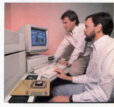
Paul Gifford (right), manager of systems engineering at Sequent Computer, and Steve Shovoly, engineer responsible for applicationspecific IC verification and procurement, use a Cadic STM5200 digital VLSI test system for ASIC design verification and characterization. Sequent, like many designers of complex ASICs, has turned to prototype testers because, according to Gifford, a foundry won't tell you how close you are to your operating margins.
