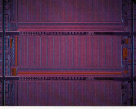
A BiCMOS device uses CMOS to implement the bulk of the logic, and employs bipolar transistors only where higher currents are necessary. In IDT's 64-kbit static RAM, for example, bipolar circuitry—shown in red—makes up a small fraction of the total chip area but contributes greatly to the device's 10-ns speed.
