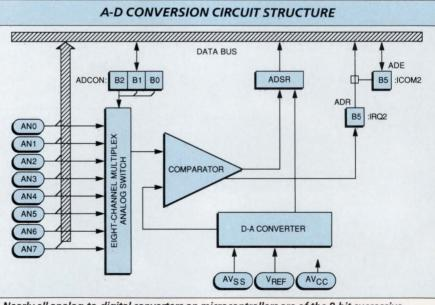
Nearly all analog-to-digital converters on microcontrollers are of the 8-bit successiveapproximation type, as shown in the M37450M2 device from Mitsubishi Electronics America. The converter selects each successive bit of the digital output based on the difference between the current output and the input.
