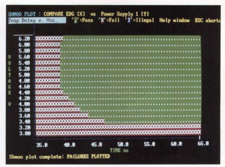
A Shmoo plot, an analysis tool included in prototype testers, lets users plot the interaction of any timing or voltage parameter against any other. A common application of a Shmoo plot is testing power-supply voltage (V<sub>cc</sub>) against propagation delay, as shown here on the Hilevel Topaz V system.
