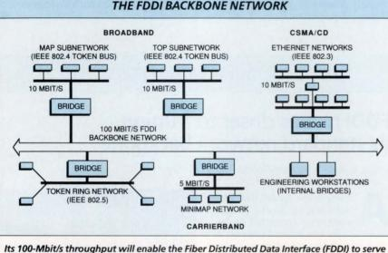
as the backbone support for many slower speed LANs, such as IEEE-802.3 twisted-pair or coax Ethernet, IEEE-802.5 token ring and IEEE-802.4 broadband coax MAP. Bridges betweeen the slower LANs and the fiberoptic backbone will be external for most applications, but will be built into devices such as larger computer systems.
