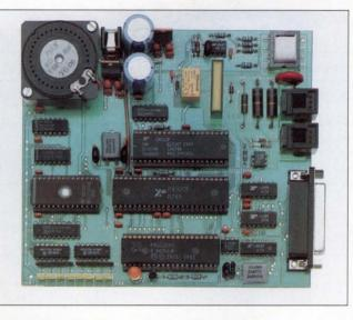
V.22bis-compatible chip sets such as Exar's XR-2400 give designers maximum flexibility by supplying complete modem functionality in two compact packages. The set consists of the XR-2401, a generalpurpose digital signal processor, and the XR-2402 analog front-end. Rather than use a dedicated controller, the chip set is designed to interface to popular off-the-shelf parts such as the 8051 and Z8.
