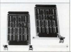
ports allow direct connection to the CPU without the need for terminal multiplexers. The board supports up to four graphics displays through the X Window System and features 512 kbytes of memory and a cache that contains 64 kbytes of external memory. The standard memory management unit that's normally part of the 68030 microprocessor is disconnected to increase performance in realtime applications.
