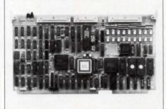
mum transfer rate of 5 Mbytes/s. Western Digital controller chips have been adopted on the device to provide the choice of either differential or single-ended SCSI bus options. Providing maximum asynchronous and synchronous transfer rates of 2 Mbytes/s and 5 Mbytes/s, respectively, the chips also support the disconnect/reconnect feature of SCSI. Single-piece price is \$1,195.
