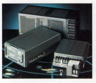
Although they don't offer the efficiency of switchers, industrial linear power supplies like Lambda's LN Series offer output ripple and noise as low as 5 mV peak-to-peak. Available in five single-ouput and five dual-output packages up to 48 V dc, this series meets MIL-STD-810 environmental conditions.
