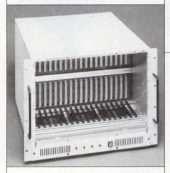
plies from 160 to 700 W. The enclosures feature a removable fan/cooling plenum, easy access to the J2/P2 sections of backplanes, light-emitting diodes to warn of power-supply trouble and interconnect I/O panels for system customization.
