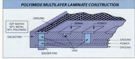
Using Microtec's additive process for constructing polyimide multilayer laminate boards, vias can be developed that start and stop between any combination of layers. Selected vias that go from the top to the bottom of the module are thermally conductive for better control of heat management.
