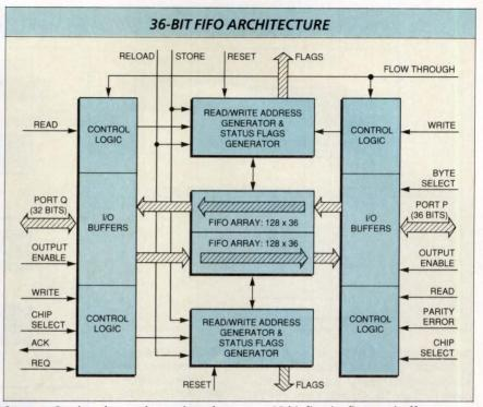
Saratoga Semiconductor plans to introduce a new 36-bit first-in, first-out buffer incorporating 36-bit-wide bidirectional ports. The proprietary architecture includes a variety of control logic functions, such as parity error and status flags.
