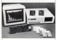
contains up to 96 kwords of zero-waitstate memory, interface circuitry for the I/O modules, and direct memory access capability for transfers to and from the PC's memory. A broad line of software is available for the DSPro line. DSP Library Plus offers a large selection of software routines that are callable from programs running on the PC.
