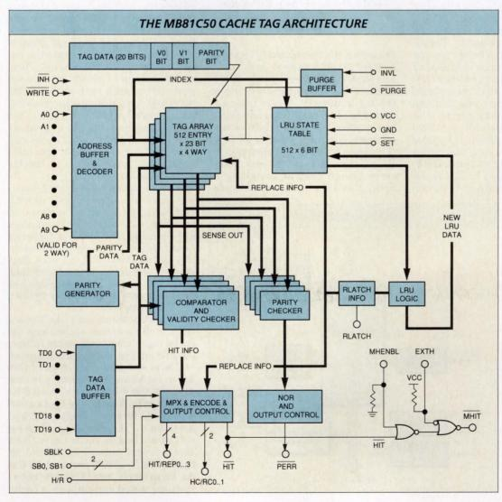
Fujitsu's MB81C50 cache tag is designed to be relatively processorindependent, unlike Texas Instruments' SN74ACT-2155. It's designed as a two- or fourway set-associative device, also unlike the TI device. Twenty of the cache tag's 23 bits are address bits. and the remaining three are for validity and parity.
