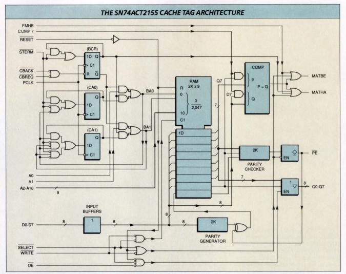
The SN74ACT2155 cache tag from Texas Instruments is designed to provide a direct interface with the Motorola 68030 microprocessor. It combines 2 kwords of 9-bit memory, a comparator and necessary cache logic. The interface and handshaking functions let it take advantage of the burst-mode capability of the processor. In addition, it has specific handshaking logic, including a pair of match outputs that speed cache operation.
