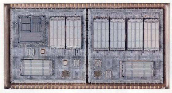
By connecting two of its 1-in.2 Programmable Silicon **Circuit Boards** through its multichip module interconnection technology, Mosaic Systems has developed a memory board that includes 1 Mbyte of cache memory, a 32-bit microprocessor and memory control chips.
