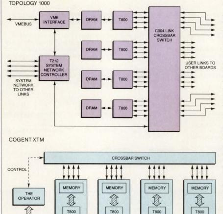
memory array and can communicate over the system bus as well as via serial direct memory access links that are part of the Transputer chip. Requests for data or for communications linkups are usually sent via the system bus. For data transfers between the local memories of different processors, the system establishes a DMA link by means of the crossbar switch.
