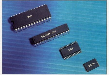
The very small outline package (VSOP) developed by Mitsibushi Electronics' Semiconductor Division for its 256-kbit CMOS static RAM has a footprint that's less than half the size of a standard SOP and is drastically smaller than a Skinny DIP or standard DIP. This reduced size lets designers pack much more memory into a system package.
