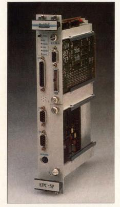
Even the PC's ISA bus has been added to the ranks of mezzanine buses. This EXMbus module from RadiSys implements the ISA interface in a form factor tailored for mezzanine service on VME boards. Others have built adapters to allow standard ISA boards to function in Multibus II systems.
