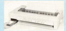
Automatic capping and an encapsulated ink cartridge make the Canon P-670 virtually maintenance free.
