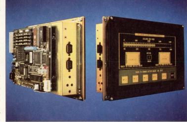
Meant for environments where standard PCs and CRTs would fail, this touch-sensitive 640x400 gray-scale electroluminescent display fronts for a full 20-MHz 80386 PC/AT processor. Computer Dynamics' DisplayPac EL mounts into a sealed enclosure, leaving its display accessible.
