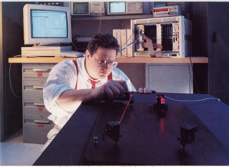
At Interferometrics Laboratories Todd Brackett, Control System Group Leader on NRL's Big Optical Array Project, adjusts the optics on a laser interferometer.
