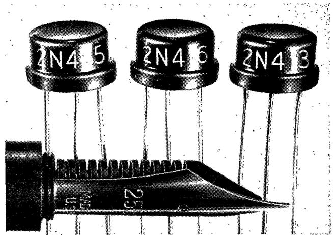
RAYTHEON MANUFACTURING CO., Newton, Mass., is now producing four new PNP germanium transistors, in a standardized package known as the JETEC 30, especially for computer use. These transistors have alpha frequency cut off at 4, 6, 11, and 17 megacycles. (See picture above.)
