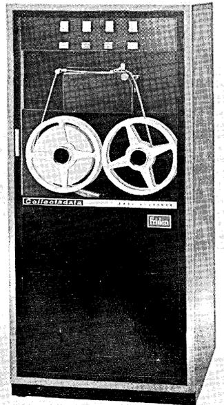
Model 3031 receives and punches into 8-channel tape information transmitted from the various points of origin. It contains tape handling mechanisms, control logic, and provides its own power and that of all transmitters on the same cable line.
