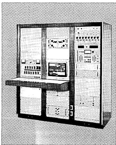
**CI-171** Test Console affords functional diagnostic test capabilities for all analog components. Features include cross bar address system, temperature controlled oven, primary resistor and capacitor standards, AC and DC load device, and advanced cable well design. Configurations for all commercially available analog computer components can be incorporated in the CI-171
