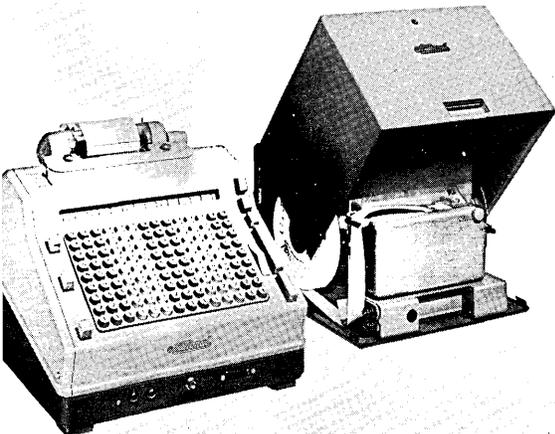
This machine translates information into machine language for computer use. The NCR tape-punching adding machine is programmed to operate the punched tape recorder automatically. An amount entered in the keyboard, adds into the machine total, prints on the adding machine tape, and is punched into the paper tape in code. An operator needs only to read printed tape to know what was recorded on punched tape. Corrections can be made before punched tape is sent off for processing.
