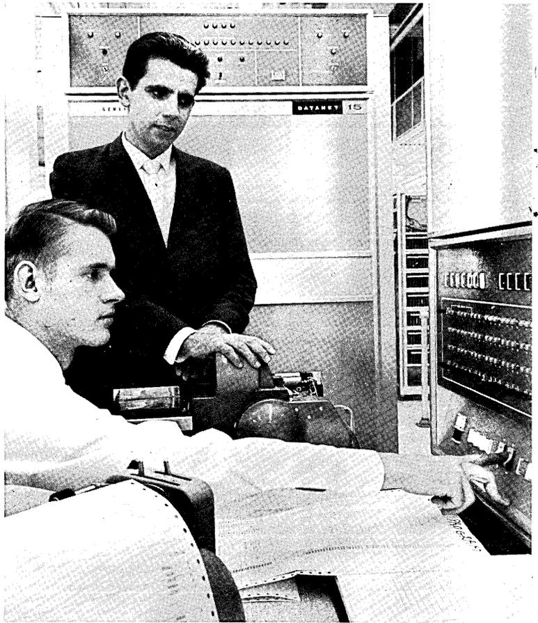
Datanet-15, data-transmission controller -- General Electric Company, Computer Department, Phoenix, Ariz. / The Datanet-15 has two basic channels, with 6- or 15-channel capability for queing. Digital data is sent or received on two-wire cable, telephone or telegraph facilities operating on-line with the GE-225 computer or its peripherals. Finger-tip controls and indicating lights are up out of the way of passing personnel.
