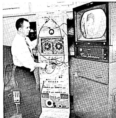
This equipment simulates the jitter (the smearing out of pulses in time) that would accumulate in a 4000 mile long pulse code modulation system. John Mayo of Bell Laboratories observes the effect of this jitter as it is automatically compensated for in the experimental high speed PCM system. The television picture on the screen is transmitted without distortion because of the "de-jitterizing" circuit.
