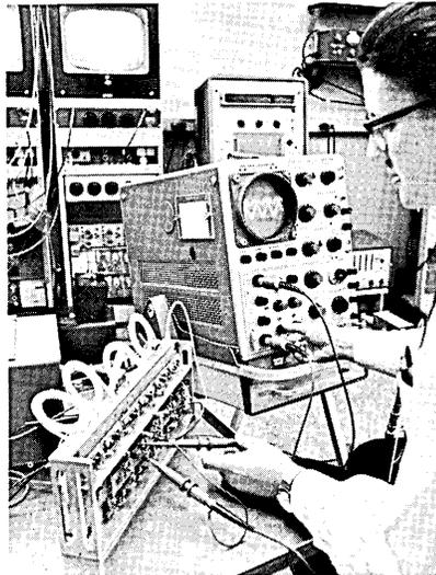
Veikko Saari of Bell Telephone Laboratories tests a laboratory model of a solid state coder. Such a device changes analog information to digital information for transmission over the experimental high speed PCM system.
