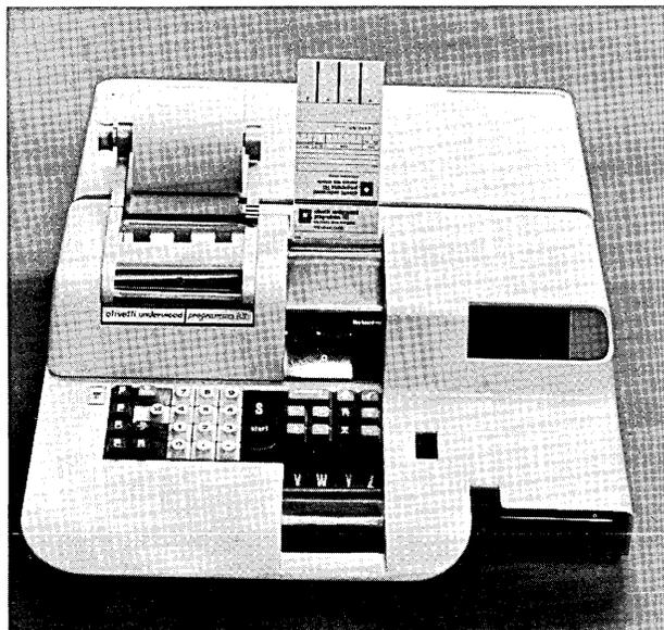
**PROGRAMMA 101** / Olivetti Underwood Corporation — The world's first desktop computer which can "write", store, and run programs while making logical decisions is about as large as a standard typewriter. Programs calling for as many as 120 instructions are stored on convenient magnetic cards (shown inserted). Results are printed out on a plain, paper tape (left). (For more information, designate #44 on the Readers Service Card.)
