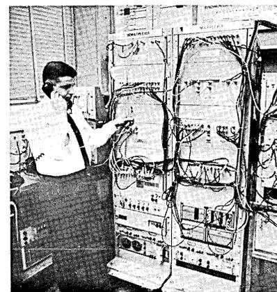
William Ballentine adjusts control on demultiplexer of experimental high speed PCM system designed at Bell Telephone Laboratories. The demultiplexer accepts a pulse stream of 224 million bits a second and separates the stream into component streams representing television, voice and data signals.
