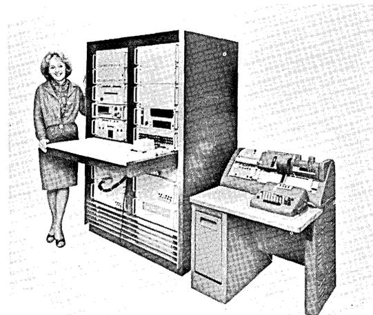
INTEGRATED CIRCUIT TESTER, MODEL 850A / Signetics Corporation — The 850A can test most of the integrated circuits on today's market including some of the recently introduced 16 terminal devices. The system is designed for easy input interfacing directly with a computer or with prepared magnetic tape, perforated tape and card-punch (shown at right of photo) programs. (For more information, designate #94 on the Readers Service Card.)
