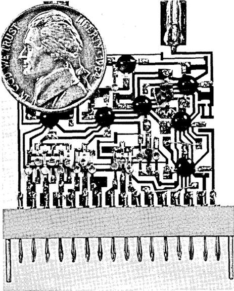
HYBRID THIN FILM CIRCUITS / The Bunker Ramo Corporation — Bunker-Ramo Hybrid Thin-Film capabilities include the fabrication of a computer circuit on a glazed aluminum oxide substrate. The substrate material facilitates dissipation of the unusually large amount of energy expended by the circuit — in this case, five watts. (For more information, designate #90 on the Readers Service Card.)
