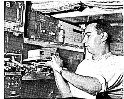
— The four principal units of the Eastern-IBM AIDS test installation are shelf-mounted in the Whisperjet's electronic equipment bay. Change of tape is accomplished by simply disengaging the top portion of the Tape Recorder containing tape reels from the bottom section containing tape drive and wiring.
