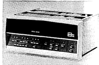
The PDC 808 has a 4,906 word 8-bit memory and 73 basic instructions. Memory is expandable to 16K words and processing is parallel with 24 microsecond ADD time. A flexible I/O section has DTL logic levels. Two priority interrupt lines and a third interrupt request line are standard. Many I/O options are available — including teletype, high speed tape reader and punch as well as magnetic tape.
