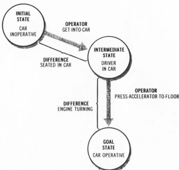
Fig. 3-4 Solution to the problem of starting the car
