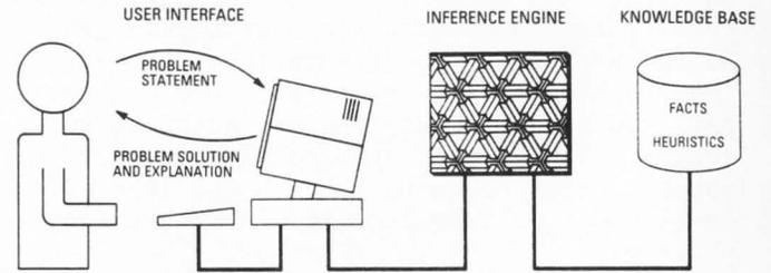
Figure 2: Main expert system components: user interface, inference engine, and knowledge base.
