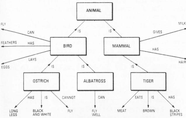
**Figure 4:** Knowledge representation using semantic networks. Knowledge is represented by the nodes, while interconnecting arcs (i.e. the lines) determine the relationship between nodes.
