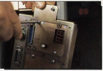
Photo 3. Remove the old rear panel switch plate.
