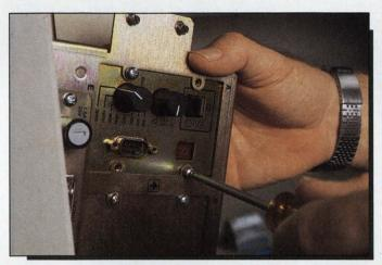
Photo 4. Install the replacement rear panel.
