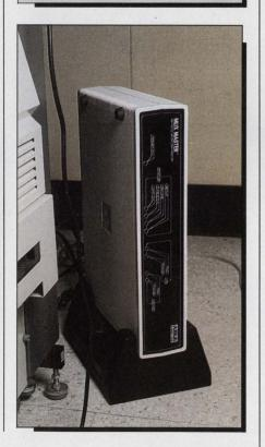
the configuration program by setting the number eight switch and hitting RETURN so the unit can autobaud your terminal (plugged into port zero). This menu-driven conversation is held just once and can be done from port zero of any convenient cluster controller (with the machine halted).
