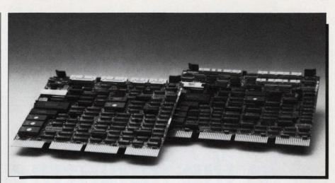
The DCV50 and DCV54 are Plessey Peripheral Systems' new disk controllers.
