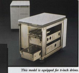
The DA 123 has a TRIMM-supplied backplane and shelving to hold four 54-inch drives.
