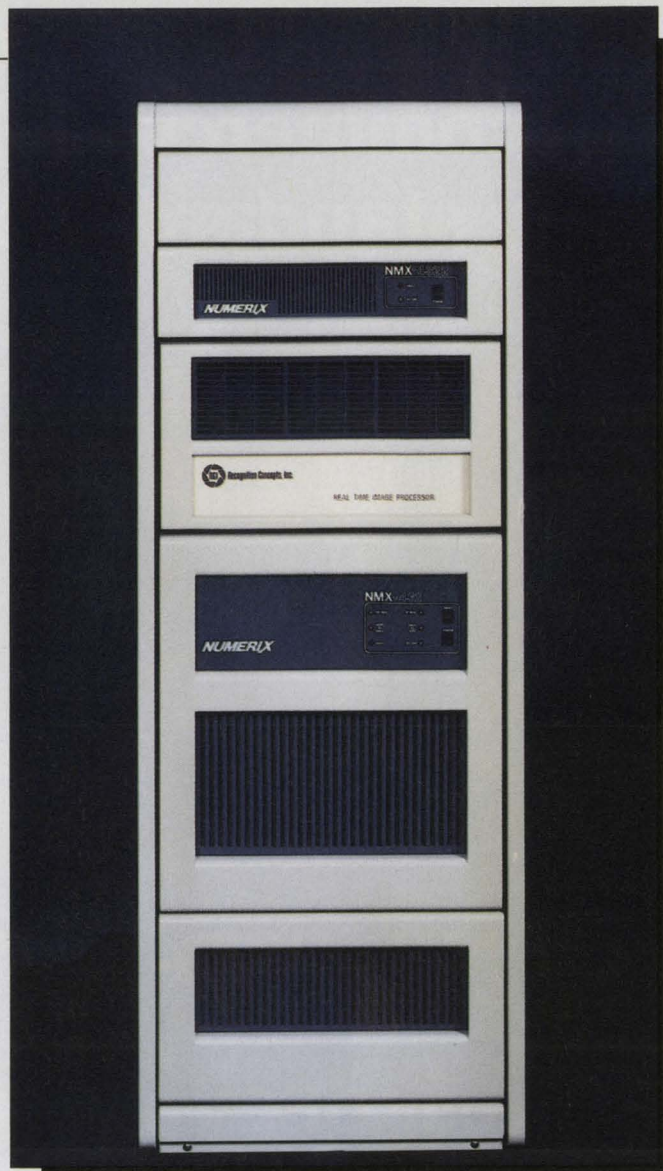
The Numerix VisiNET interface and RCI's Trapix image processor sit atop the NMX-432 attached vector processor.
