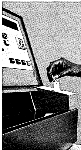
DPI Data Collection Terminal "turns on" when I.D. badge is inserted.
