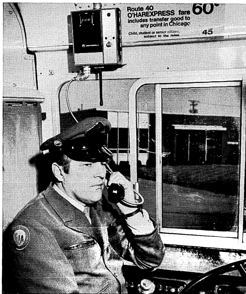
The dispatcher can respond to a crt-displayed "late run" message by dialing the bus and talking with its operator. The dispatcher already knows the bus's garage, run, and vehicle numbers and its location.
