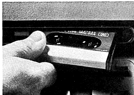
Plug-in mass storage: you can get up to 110,000 bytes per cartridge.
