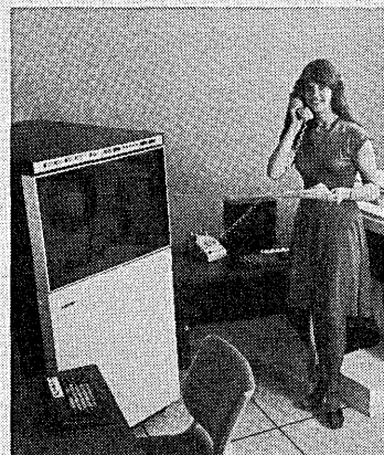
The 1303 provides medium range data entry capacity, with about triple the disc capacity of the 1301. It supports up to 16 keystations and the addition of edits, table look-ups, range checks and cross-footing. The 1303 also offers communications capabilities such as spooling , HASP and RJE .
