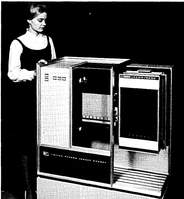
A random access memory from Potter Instruments used loops of mag tape in cartridges, each storing 3 to 40 million characters. Average access time was 168 milliseconds.
