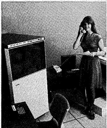
The 1303 provides medium range data entry capacity, with about triple the disc capacity of the 1301. It supports up to 16 keystations and the addition of edits, table look-ups, range checks and cross-footing. The 1303 also offers communications capabilities such as spooling , HASP and RJE .
