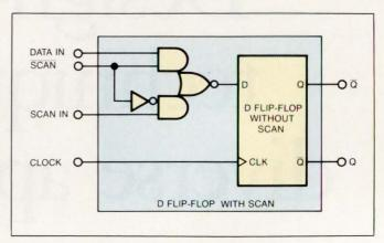
Fig 1—When you use the structured technique, your circuit overhead increases in proportion to the number of gates required to implement the scan capability within a sequential device. For example, it might take three or four extra gates to perform the scan function for a D-type flip-flop.
