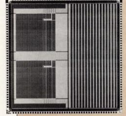
Fig A—This die photo of the LSA2002 structured array shows the relative size and placement of each building block. The gate array is on the right, and the two 3-port RAMs are on the left.
