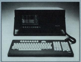
You can develop software for many microcontrollers on this 8-bit development system, the Echo from Arium. The system lets you test your software right on the target machine with the aid of an emulator and a personality board that control the execution of your programs and trap errors.
