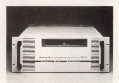
Storing 5.2G bytes on a VHS tape cassette, the VLDS sustains a data-input rate of 4M bytes/sec and features a bit-error rate of 1 error in 10<sup>12</sup> bits.
