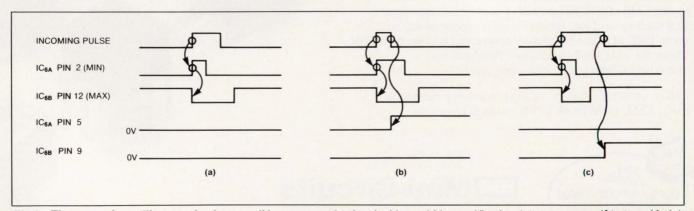
Fig 2—These waveforms illustrate the three possible outcomes of pulse checking: within specification (a), too narrow (b), too wide (c).
