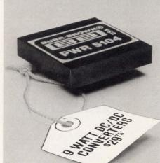
Low Price, High Performance. Our new PWR5104/05 DC/DC Converters are priced lower than anyone else we know, and the performance is better, too! Just \$29.75 each in 1000s buys you a full 9W of output power at ±12VDC or ±15VDC, and maximum ripple and noise of only 35mVp-p.
