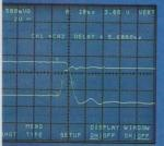
Now you can make automatic channel-to-channel propagation delay measurements with user-defined thresholds. Shown above is a propagation delay measurement from the mesial (midpoint) of the ECL rising edge on Channel 1 to the mesial point of a TTL falling edge on Channel 2. Display the waveform and read out the values on screen or over the bus.
