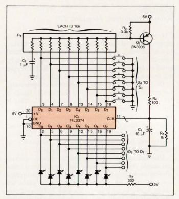
Fig 1—This single-IC circuit debounces a group of eight pushbutton switches, latches the last switch closure, and provides an LED indicator for the currently active circuit.
