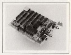
range and a 4- or 8-kHz sample rate. When you use a 4-kHz sample rate, the board requires 7.2M bytes to store one hour of digitized signal. \$345.
