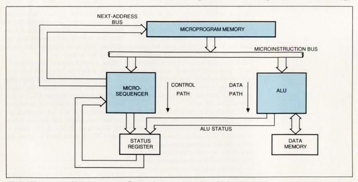
Fig 1—Microprogrammable processors generally comprise two major sections: the data path and the control path. The slowest path determines the processor's maximum execution speed.
