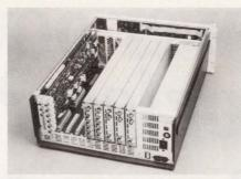
Capable of holding as many as eight modular instruments, the 680 mainframe lets you program simple test procedures from its menu-driven front panel.
