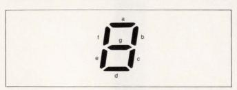
Fig 2—This standard character format lets you represent numbers by selectively illuminating the seven segments labeled a through g.
