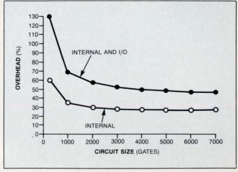
Fig 2—Although BIST techniques require more silicon overhead than do the other design-for-testability techniques, the percentage of circuit overhead required by the BIST circuitry decreases as you increase the size of the circuit.
