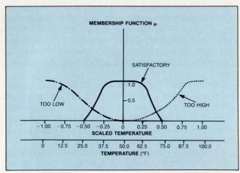
Fig 1—A typical fuzzy set's membership functions consist of a convex curve that describes satisfactory operating conditions and a concave curve that describes unsatisfactory conditions.
