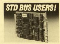
The 890 Z80A Multifunction CPU card is an integrated hardware/software solution for industrial control applications
