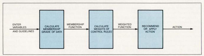
Fig 2—By following these steps, a fuzzy-logic controller can analyze a set of process variables, find the weighted average of all control rules in the process, and perform the same action that an expert operator would.
