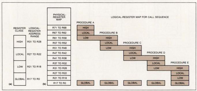
Fig 3—By referring to the logical-register-address ranges in a and following a 5-procedure call in b, you can understand how the overlapped register windows operate.
