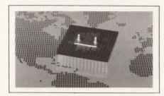
ate sine-wave frequencies from 1 Hz to more than 120 MHz. This monolithic device has TTL-compatible inputs, ECL-compatible outputs, and an internal oscillator that operates at frequencies as high as 300 MHz. You can program the output to 32-bit (almost 1 Hz) resolution, and you can change frequencies as often as every 110 nsec. The package is a 156-pin ceramic pin-grid-array device with heat-sink mounting studs. \$625 (100).
