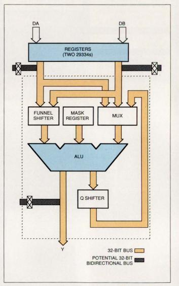
Fig 3—By separating the ALU and register file into the Am29332 ALU and Am29334 register file, Advanced Micro Devices offers you even greater data-movement flexibility than its 29203 can provide. The 4-port register file accepts two values and delivers two values in one machine cycle, and the feedback path between the ALU and register file is external to the ICs so you can connect these parts to best suit your architectural needs.
