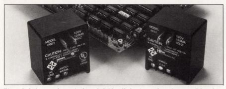
Five-volt designs are best suited to a hybrid wall plug-in supply such as one of these from James Electronics. A hybrid supply has a linear front-end to reduce and rectify the line voltage to an 8 to 9V range, followed by a switching regulator to translate the unregulated 8 to 9V to 5V.
