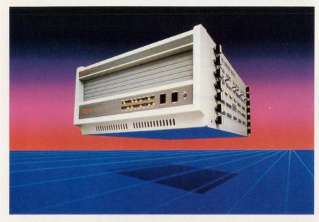
Microprogram development systems give you mastery over your evolving processor design. This Step-40 from Step Engineering accepts a variety of writable-control-store memory cards, logic-analyzer cards, and device-emulation cards to match the size and scope of your project requirements.
