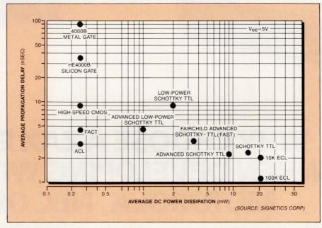
Fig 1—Illustrating the comparative speed and power characteristics of the various CMOS and bipolar logic families, it's clear that advanced CMOS logic offers speeds that rival those of bipolar devices with far less power consumption.
