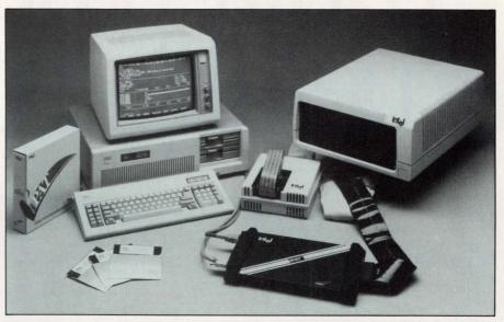
Using this cross-development system, you can develop your software on an IBM PC and debug it on the target machine with the aid of an emulator. Intel's Performance Analysis Tool (PAT), shown in the foreground, monitors the execution of your program on the target and allows the PC to display histograms showing the time spent in each routine.
