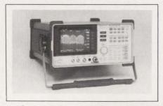
analyzers, cover a 1-kHz to 22-GHz frequency range. The HP 8562A provides tracking preselection from 2.75 to 22 GHz; the HP 8562B provides no preselection. The instruments have a 1-dB/division scale factor, and their synthesized tuners sport 100-Hz tuning steps. The analyzers' frequency response is  $\pm 1.2$  dB at 2 GHz and  $\pm 4.3$  dB at 22 GHz. The ratio of signal to harmonic distortion is 100 dB max; the ratio of signal to intermodulation distortion
