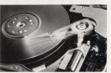
A servocontrolled, rotary voice-coil actuator gives this 53.3M-byte, half-height, 54-in. Winchester disk drive its high capacity and speedy (25-msec) average access time.
