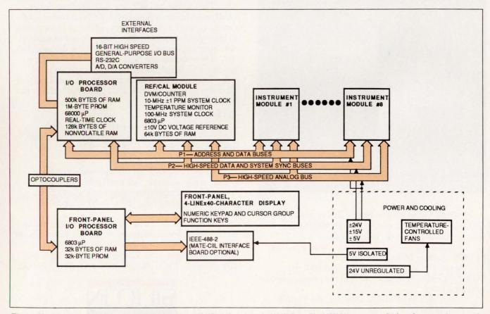
Fig 1—The high-speed modular intrumentation bus (HMIB) is based on the VME Bus. The HMIB's connector P1 has the same pinout as the VME Bus's connector P1. The HMIB's connector P2, however, differs from that of the VME Bus in that it adds an ECL and a high-speed TTL digital data bus, as well as system trigger and sync buses. The HMIB has an additional connector, P3, which is dedicated to analog signals.
