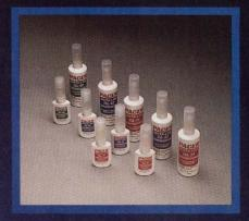
Our Insta-Lok grades are unique patented technology; structural cyanoacrylates offering the strength and durability of an anaerobic and the cure time of an instant adhesive. Unlike anaerobics, these compounds perform well on platings, stainless steel and plastic fasteners without the use of surface activators.
