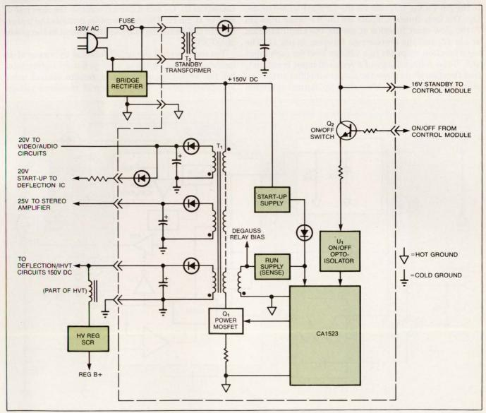
Fig 4—In a typical TV-receiver application, the switching transformer isolates the power line from the signal circuits of the receiver and provides the voltages required for the various circuit sections.
