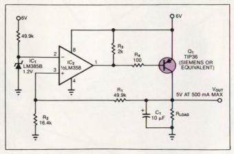
Fig 1—The low saturation voltage of  $Q_1$  lets this 5V regulator operate with input-output differentials as low as 0.1V.
