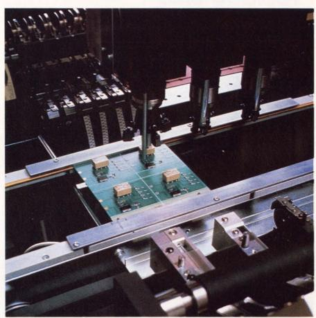
Not all components change when designed into SMT packages. These relays, for example, have identical mechanical and electrical specs to their through-hole counterparts. (Photo courtesy Omron)
