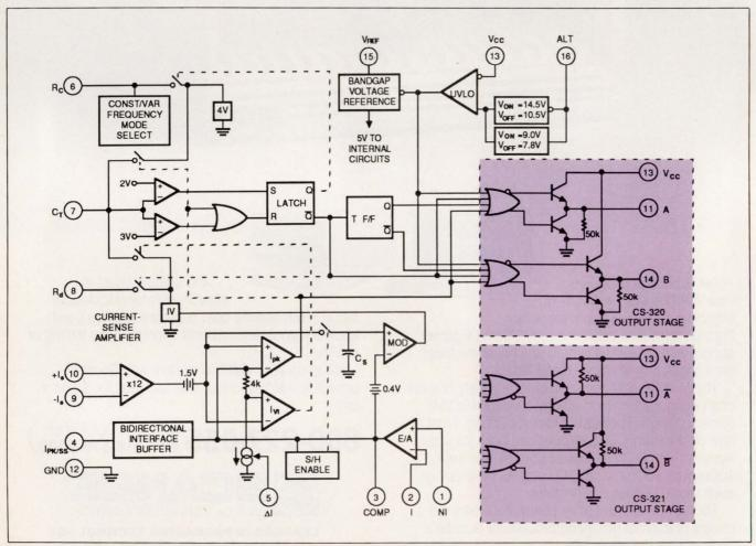
This power-supply-control IC provides three current-mode options: hysteretic, constant-off-time, and constant-frequency control. The IC's high-current totem-pole output is suitable for driving power MOSFETs.
