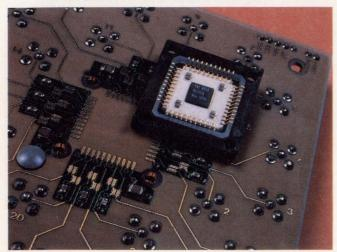
Fig 2—This gate array, a member of Triquint's Q-chip series, is a GaAs, ECL-compatible chip that blazes along at a 2-GHz flip-flop toggle frequency.
