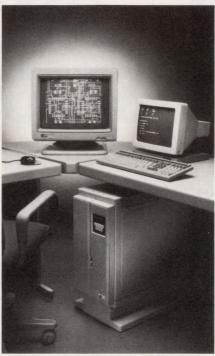
To lay out very dense pc boards, as well as those that include SMDs or other new-technology devices having nonstandard lead spacing, you can use the variable-grid router available for Calay's Design Automation workstations. This hardware router eliminates restrictions on grid size, letting you select grids of any resolution.
