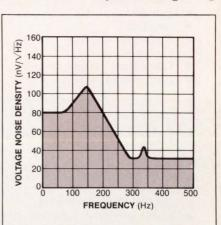
Fig 2—The 1/f noise of a chopper-stabilized op amp actually decreases at low frequencies, where a conventional op amp's noise increases at a 3-dB/octave rate.
