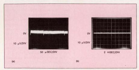
Fig 1—The noise of a chopper-stabilized op amp (a) is 10  $\mu$ V p-p with 16  $\mu$ V p-p switching spikes. The noise of a conventional OP-77 op amp (b) is on the order of 2  $\mu$ V p-p. For both cases, gain equals 1000.
