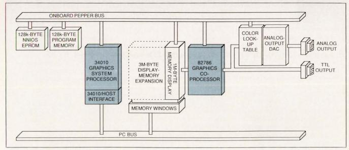
Fig 1—Combining the TI TMS34010 and the Intel 82786, the \$995 Pepper SGT board from Number Nine Computers uses the firm's proprietary software interface, NNIOS, to control communications among the two graphics engines, the host  $\mu P$ , and memory.
