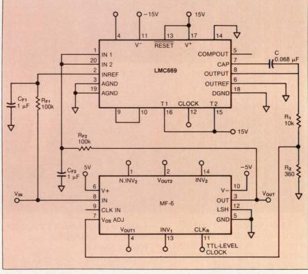
Fig 3—The LMC669 auto-zero circuit from National Semiconductor corrects the 250-mV offset of an MF-6 switched capacitor filter. The  $V_{\rm OS}$  of most inverting systems can be corrected in this manner.
