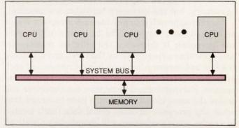
Fig 1—All processors share a single large memory and can read from or write to any location in the shared-global-memory architecture. This model requires that both the memory and the system bus have a very high bandwidth.
