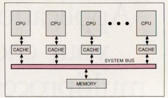
Fig 2—You can reduce bandwidth (and cost) in a multiprocessor system by providing each processor with a local high-speed cache. However, if more than one processor will access the same global data, you'll have to ensure that when any processor updates global data that's located in a cache, some mechanism will immediately update all other caches containing that data.
