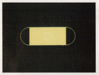
Fig 2—We solved the PLCC-pad problem (illustrated in Fig 1) by rounding the ends of the pad, but that forced us to change the pad's width from 25 to 26 mils. The Cadnetix pad editor only allowed even diameters for circles and arcs.
