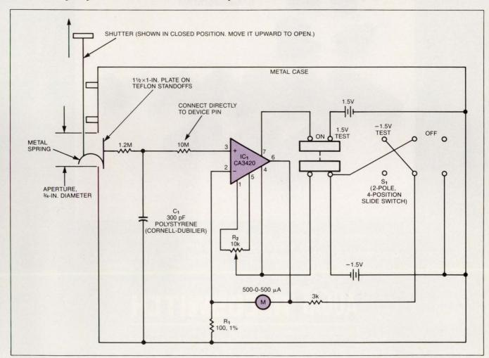
Fig 1—This voltmeter measures electrostatic potential as low as 1V without touching the voltage source. The full-scale input at 3.5 in., for example, is 5 kV.
