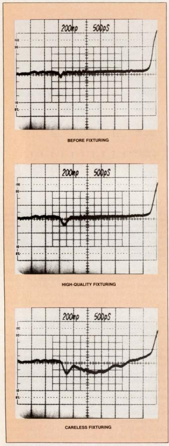
Fig 3—Signal quality can limit overall test system performance. In addition to clock-cycle rates and measurement-strobe resolution, you must take into account rise time, fall time, overshoot, undershoot, and ringing.
