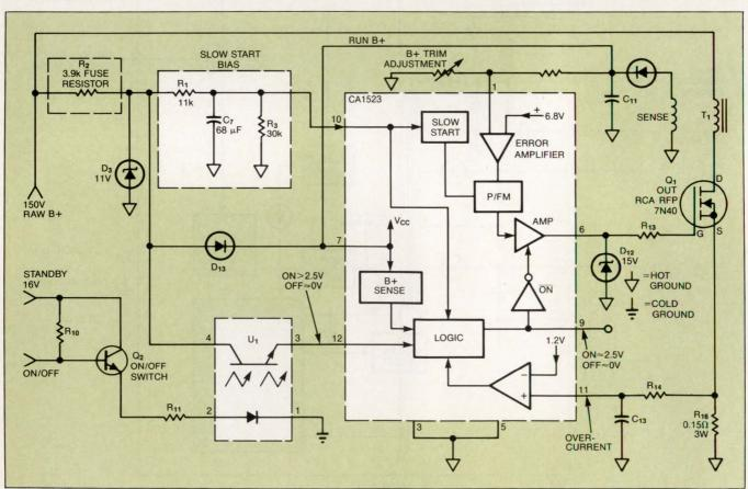
Fig 5—Within the on/off operation, logic function inputs from pin 7, slow-start bias from pin 10, opto-coupler on/off function from pin 12, and over-current protection from pin 11 control system operation.
