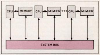
Fig 4—In the shared-local-memory model, bus- and memorybandwidth requirements are less stringent than those of the sharedglobal-memory model, and moving a task from one processor to another becomes easier.
