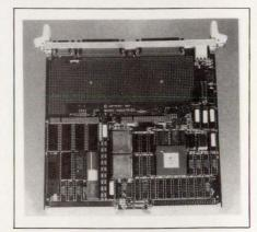
general-purpose intelligent interface to the Multibus II parallel system bus (iPSB). The board includes an 80186  $\mu$ P, an independent configuration processor, as much as 256k bytes of EPROM, as much as 512k bytes of dynamic RAM, an 82258 DMA controller, an 8259 interrupt controller, a serial communications port, and a prototype area that takes up one third of the board's area. The prototype area has access to the local  $\mu$ P bus. The serial com-
