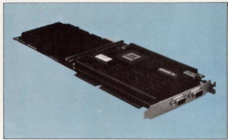
In its PG-1281 intelligent graphics add-in board, Matrox accelerated some of the 34010  $\mu$ P's commonly used graphics software routines by implementing them in ASICs. The company then took advantage of this proprietary hardware by developing its own software library.
