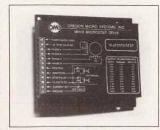
Using an external resistor, you can program the output current yourself. The supply voltage range for the driver spans 24 to 60V. The step and direction inputs are opto-isolated to minimize ground loops and improve noise immunity. The drive is packaged in a 4×4.5×1-in. module, including mounting flange. \$350.
