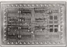
The ALA200 UHF linear array is divided into 12 modules: eight standard, two power, one input, and one trim. Each standard module contains 12 npn and seven pnp transistors, as well as 84 implanted resistors. The other modules contain similar quantities of components, which vary slightly for each module. The array is laid out on a grid system, which facilitates the interconnection of components.
