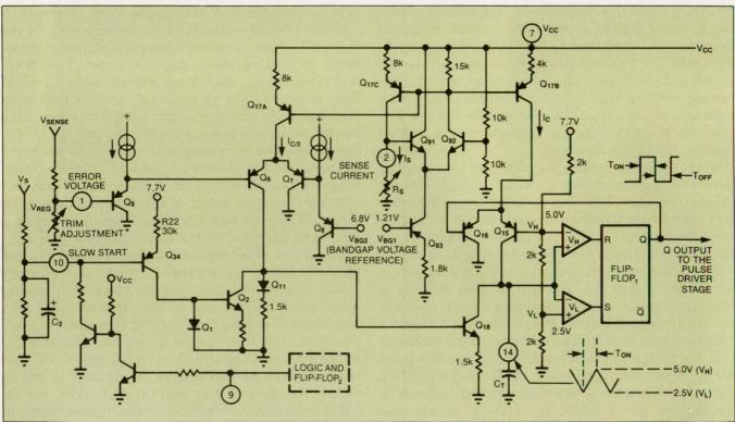
Fig 3—For a given timing capacitance,  $C_T$ , in the modulation and timing circuit of the CA1523, the maximum frequency of the P/FM circuit is determined by the current sense bias set by resistor  $R_S$  at pin 2.
