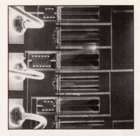
Acceleration Switches: Cantilever beams of silicon dioxide overhang shallow wells in silicon. Beams flex under acceleration, making electromechanical contact.
