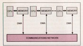
Fig 3—In the processor-network model, each processor has its own local memory, and processors communicate with each other by sending messages over a communications network. The distribution of tasks becomes a complex software problem.
