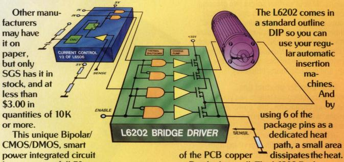
power integrated circuit lets you put a full 70 watts into your stepper or DC motor and control it directly from TTL, CMOS or even a micro.
