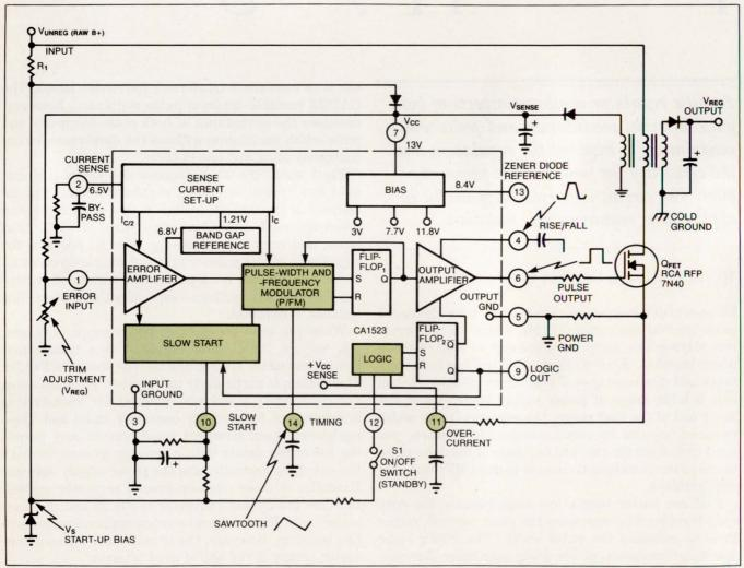
Fig 1—A typical switching-regulator power supply uses this functional block diagram and external circuitry. Features of the CA1523 control IC include a slow-start controlled power-up, logic control of the output pulse, and overcurrent sensing.
