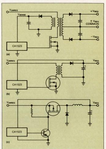
Fig 2—The CA1523 can be useful in various switching powersupply systems: a line-isolated flyback converter (a), a nonisolated flyback converter (b), and a buck converter regulator (c).
