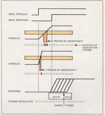
Fig 4—The overall accuracy of a tester's timing measurements depends on both its stimulus and acquisition performance. Slow driver rise times create an area of uncertainty that limits timing accuracy. System skew of both the stimulus and acquisition circuitry also places a fundamental limit on the integrity of the device measurements.
