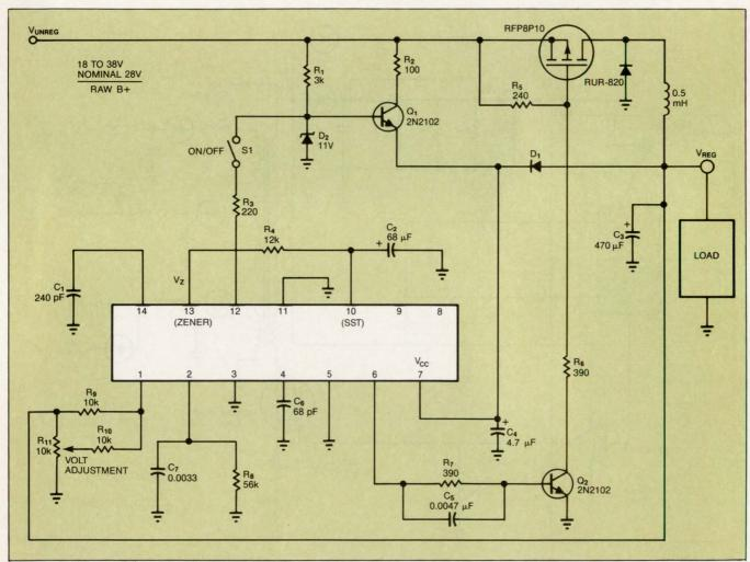
Fig 7—The buck regulator is useful in low voltage applications. It has an adjustable output voltage and a special start-up feature that minimizes the standby current in zener  $D_2$  and makes use of the internal zener diode for slow-start control. The error feedback voltage is adjustable over a range of 6.8 to 13.5V, and the pulse-frequency range is typically 25 to 75 kHz. Regulation at a nominal 12V output is typically 0.3%.
