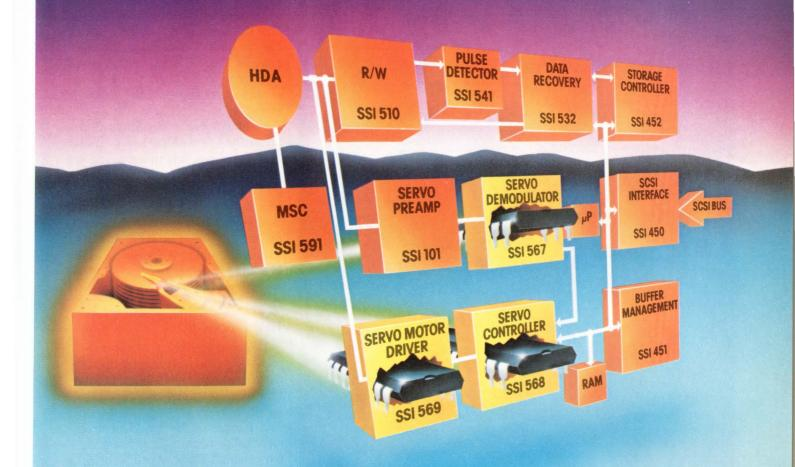
Silicon Systems now introduces the SSI Servo Chip Set. It is a 3-chip servo set for precise head positioning in the new high-performance hard disk drives. This is just the latest development in the company's program for the full integration of disk drive electronics.
