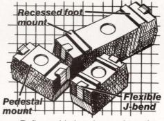
Reflow soldering cleanup is easier with the recessed foot mount design, and the decrease in board contact helps lower your board temperatures.
