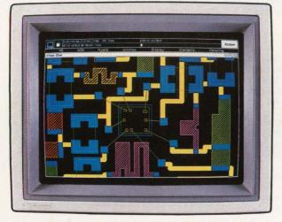
A dedicated package for thick and thin film hybrid design features automatic resistor generation and automatic routing of chip and wire parts and SMDs
