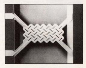
Mass Flow Sensor Element: All-silicon structure with micromachined bridge and channel. Multiple-element structure measures mass flow rate in a commercial gas control system.
