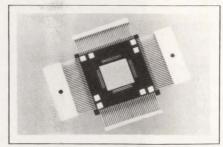
2 nH, and a resistance of 30 m $\Omega$  max. The carriers' design lets you bond the die directly to a heat sink to control heat problems. The standard controlled impedance equals  $50\Omega$ , but other values are available. The Phil units have the same 0.025-
