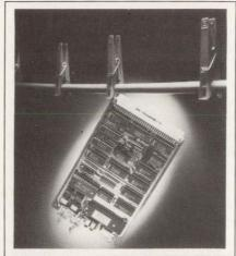
master or as a stand-alone Bitbus node processor. In STE Bus master or stand-alone mode, commands sent via the Bitbus allow you to read or write to STE Bus or local I/Oport locations. As a result, you don't need to write firmware for the SNETM board for simple control applications. For stand-alone operation, the vendor provides an I/O connector with 16 digital lines, so
