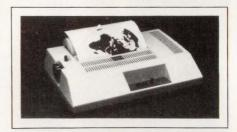
tion, fixed-array, thermal print head, which provides dot-for-dot reproduction of a screen image as dense as  $1536 \times 1024$  pixels. The frame grabber captures an entire screen in ½0 sec, so you don't need to freeze the display. The entire printing process takes 10 sec. You can choose any of 100 preset display types, which automatically set the display size, pixel resolution, and other display parameters. \$2995.
