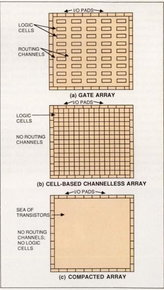
Fig 1—In the traditional architecture of a gate array (a), I/O pads surround columns of logic cells interconnected via the routing channels. Channel-free arrays (b) increase the gate count by filling the entire array with logic cells and by allowing you to use any part of the array for interconnections. The basic building blocks of compacted arrays (c) are p- and n-channel transistors, not logic cells.
