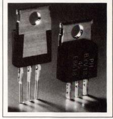
of 30 mA at maximum rated voltage. The maximum output current with both diodes conducting is 10A, and they have a typical forward voltage drop of less than 0.6V. Configured as a common cathode pair, both diodes are diffused onto the same silicon die, providing thermal stability and current-sharing capability. As a result, you can parallel the diodes without derating them. The housing
