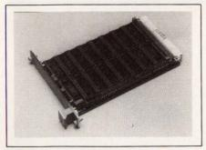
holding as much as 2M bytes of static RAM or ROM. You can load the board with a combination of RAM and ROM as your application requires. The device-access times can range from 100 to 250 nsec, and the board is divided into two separate memory areas for which you can specify different access times. The board will accept RAM or ROM devices with capacities as high as 1M bit. The board makes provision for the battery backup of the static RAM. DM 990.
