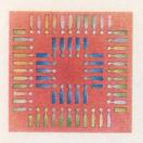
Fig 4—We caught this photoplotting error just in time. The lower plot shows a normal edge connector on the board's component side, but the pads on the upper plot are rotated 90°, thus creating a shorting bar instead of an edge connector on the circuit side of the board. The error occurred when human intervention was required to transfer information from the pc-board CAD development system to the CAD system at the pcboard vendor.
