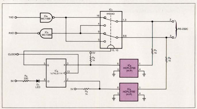
Fig 1—If you inadvertently plug in an RS-232C connector backwards (crossing the transmit and receive signals), this circuit will detect the fault and automatically swap the signals back to the proper lines.
