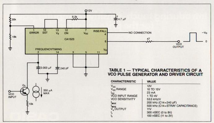
Fig 9—The CA1523 can act as a general-purpose VCO pulse generator. The external transistor provides a linear drive current to the current sense input, pin 2. The timing capacitor at pin 14 controls the pulse-frequency output; pin 2 current controls the 50% duty cycle.
