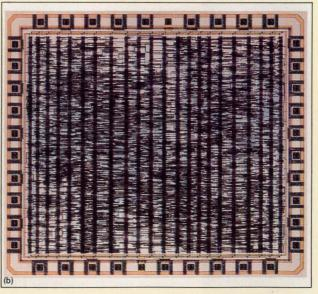
Fig A—All three of these RISC processors are derived from the same user input. They were implemented by VLSI Technology's silicon compiler, which lets you design your ICs in a technology-independent fashion: You can make the choice to use cell-based (a), standard-cell (b), or compacted (c) arrays at the end of the design cycle.
