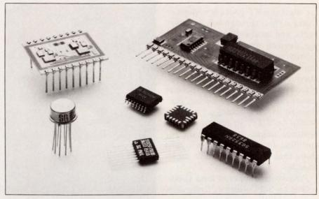
SMT components promise smaller, faster circuits, but a host of subtle spec differences may trip up the unwary design engineer faced with converting through-hole designs to SMT. (Photo courtesy Silicon General)
