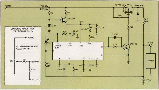
Fig 8—A buck regulator uses the internal zener diode at pin 13 as a reference for the return divider from the regulated output voltage. An optional adjustment uses the external start-up zener diode to replace the resistive divider.
