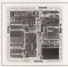
privileged registers, and a 32-bit data bus that operates at 20 MHz. The chip uses a 2-clock bus cycle and 6-stage pipeline to achieve a peak performance of 6.6 MIPS and a peak data-transfer rate of 40M bytes/sec. The V70 supports the Itron operating system and the Unix System V. It includes an emulation mode that executes all V20/V30 and V40/V50 software. Other features include demand-paged memory management with 4G bytes of virtual space for
