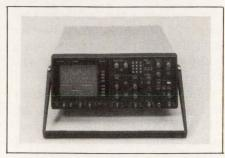
with 10-bit resolution. The scope can capture data at 250M samples/sec. It has two 2048-sample memories (in single-channel mode, it has one 4096-sample memory) and can operate in repetitive-sampling or single-shot modes. The instrument has simple, built-in math functions, and its CRT features cursor and scope-setting readouts. IEEE-488 and RS-232C interfaces are optional. Model PM3320, \$9,900. Delivery, eight weeks ARO.
