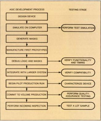
Fig 1—The numerous test stages in a typical ASIC development process range from initial simulation on the CAE workstation to production testing and incoming inspection. Test requirements vary at each stage, so you have to evaluate different ASIC test equipment and feature sets.
