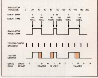
Fig 2—Importing test vectors from the CAE simulation environment can save a lot of time at the functional test stage. Unfortunately, simulators and testers have fundamental operational differences, so the conversion task isn't simple. Testers vary in their ability to mimic the simulator's output. Here, the shaded areas of the "Tester Output" signal represent time increments that are overlooked by simple functional testers lacking data-formatting and edge-placement capability.
