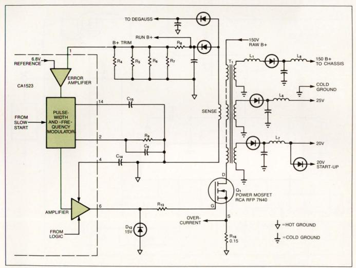
Fig 6—When the CA1523's output functions in a normal feedback mode, the input to the error amplifier from the rectified sense voltage is compared to the 6.8V internal reference and provides the correction signal for the P/FM function. Timing capacitor  $C_{15}$  and sense current resistor  $R_9$  controls the pulse-width and -frequency modulation. The logic input controls the output amplifier, whose rise time is determined by capacitor  $C_{14}$ .
